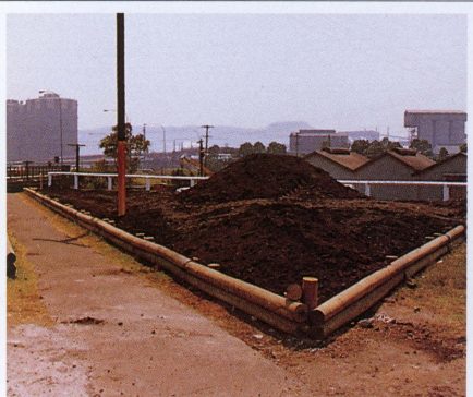
10. Environmental technology enables waste materials – sewage sludge, granulated slag and coal wash – to be turned into 12 tonnes of high quality soil substitute, enough for a good-sized garden.
