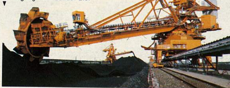
6,600 T/H Stacker x 4 and 8,000 T/H Reclaimer x 2, Kooragang Coal Loader Ltd.
