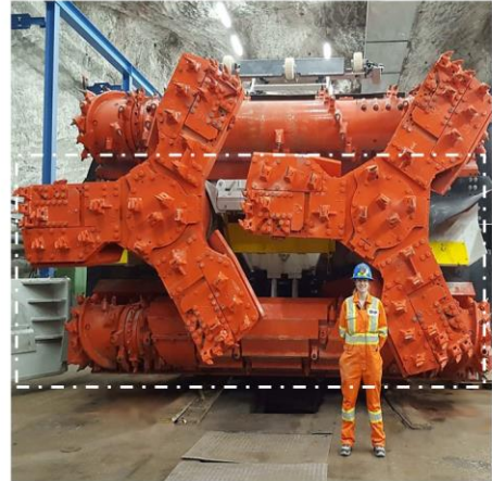
Dotted line indicates typical conventional borer height
