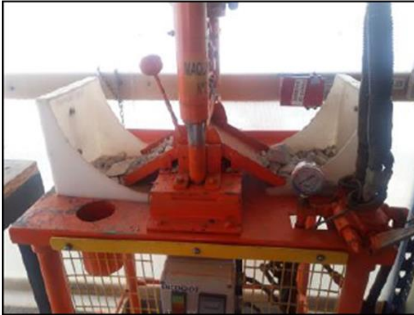
Figure 8-5: Hydraulic Guillotine for Core Cutting
