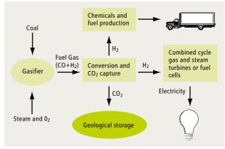
► Capture and storage of CO<sub>2</sub> from coal gasification
