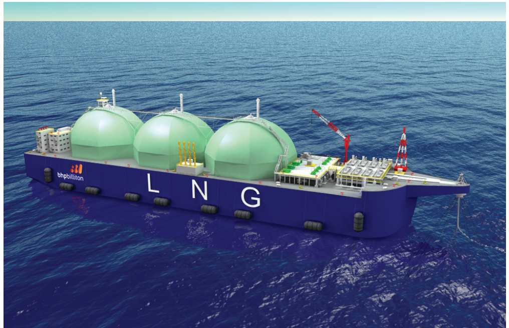
Cabrillo Port's Floating Storage and Re-gasification Unit will be the receiving point for LNG shipments.
