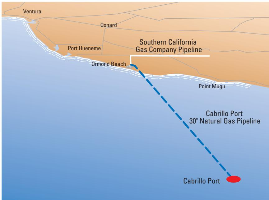
**Cabrillo Port will be approximately 21 miles offshore from the City of Port Hueneme. The pipeline will come to shore to connect with the existing Southern California Gas Company pipeline system.**
