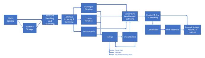
Figure 12 Jansen Process block flow diagram
