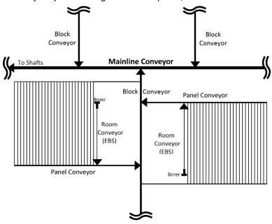
Figure 11 Conveyor type and application
