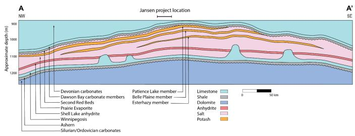
Figure 4. Schematic geological section showing the potash members of the Prairie Evaporite Formation. The location of the section is shown on Figure 3.
