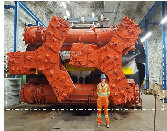
Dotted line indicates typical conventional borer height
