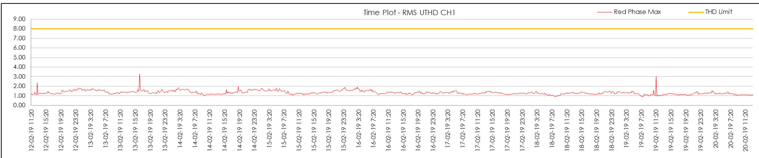
Figure 68 | TC2 End U-THD measurements (Red Phase)
