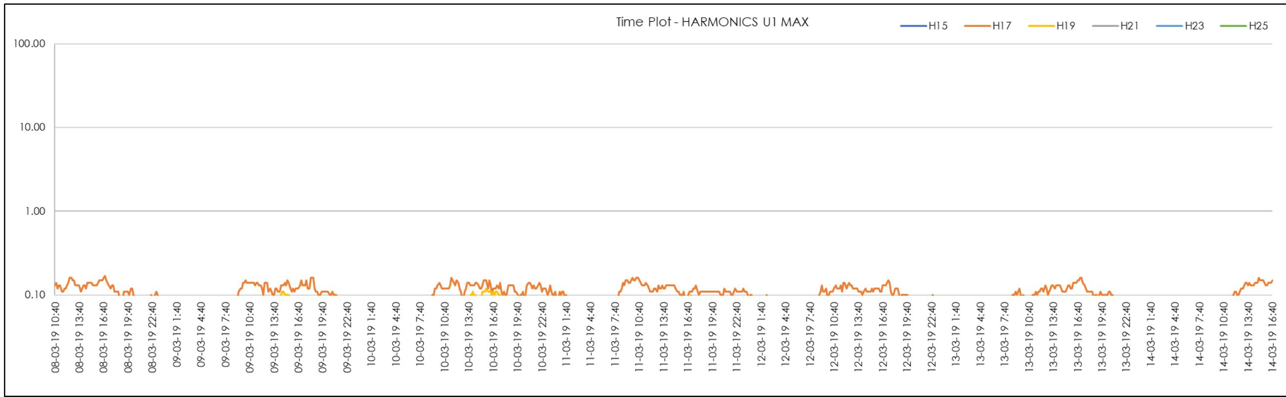
Figure 102 | TC3 Start Odd 15<sup>th</sup>-25<sup>th</sup> Harmonics (Red Phase)
