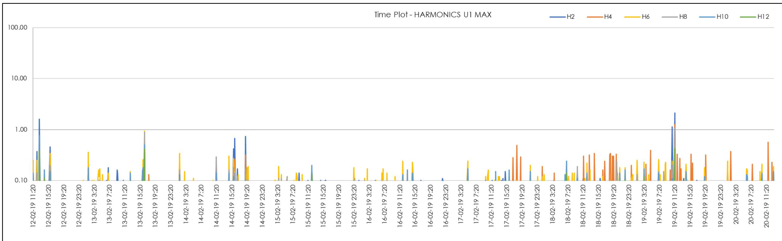
Figure 75 | TC2 End Even 2<sup>nd</sup>-12<sup>th</sup> Harmonics (Red Phase)
