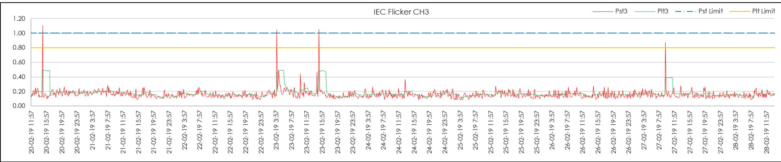
Figure 112 | TC4 End Flicker measurements (Blue Phase)
