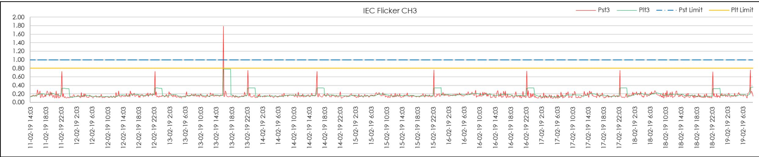
Figure 28 | TC1 End Flicker measurements (Blue Phase)
