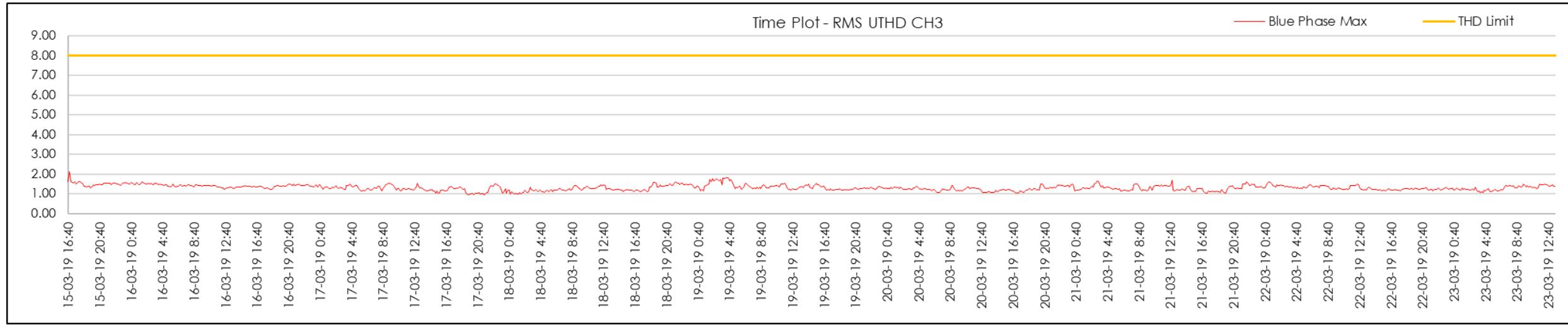
Figure 67 | TC2 Start U-THD measurements (Blue Phase)
