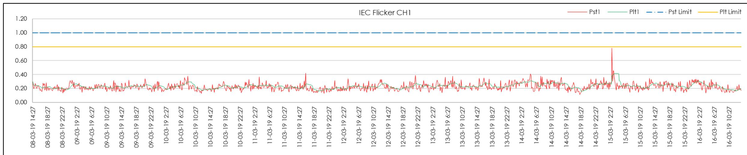
**Figure 194 | STS4 End Flicker measurements (Red Phase)**
