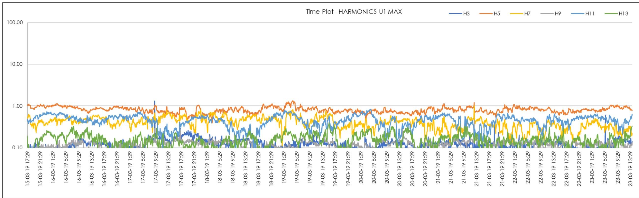
Figure 129 | TC4 Start Odd 3<sup>rd</sup>-13<sup>th</sup> Harmonics (Red Phase)
