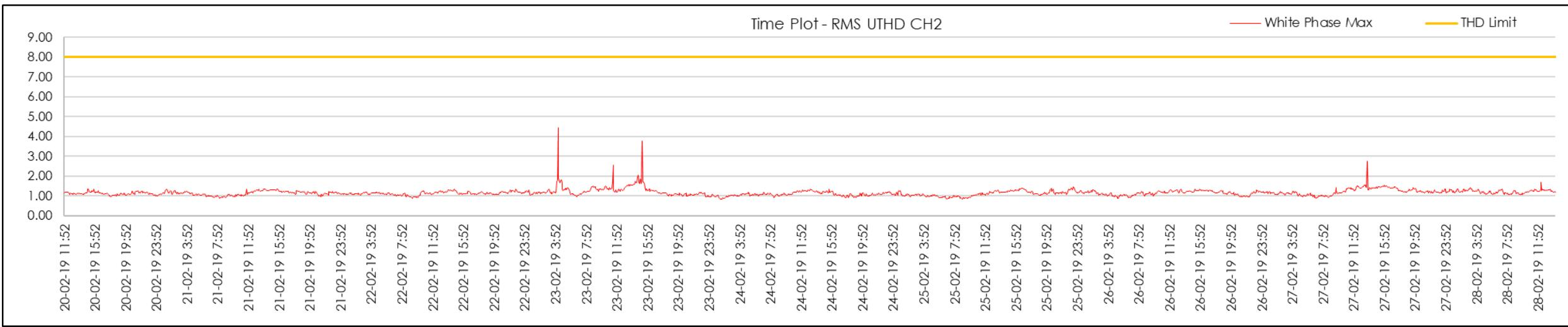
Figure 125 | TC4 End U-THD measurements (White Phase)
