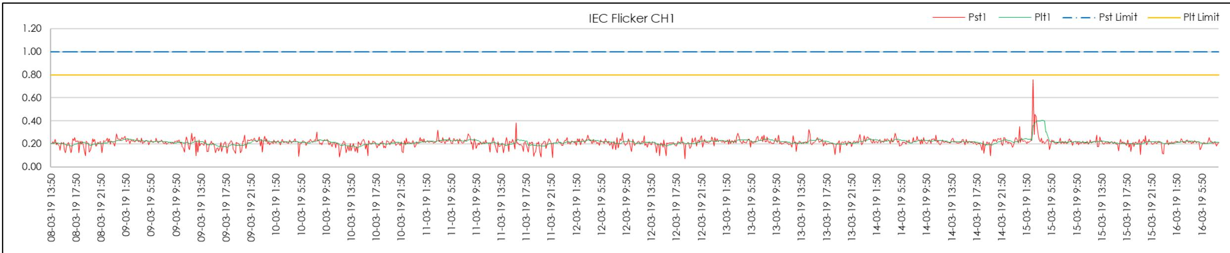
Figure 191 | STS4 Start Flicker measurements (Red Phase)
