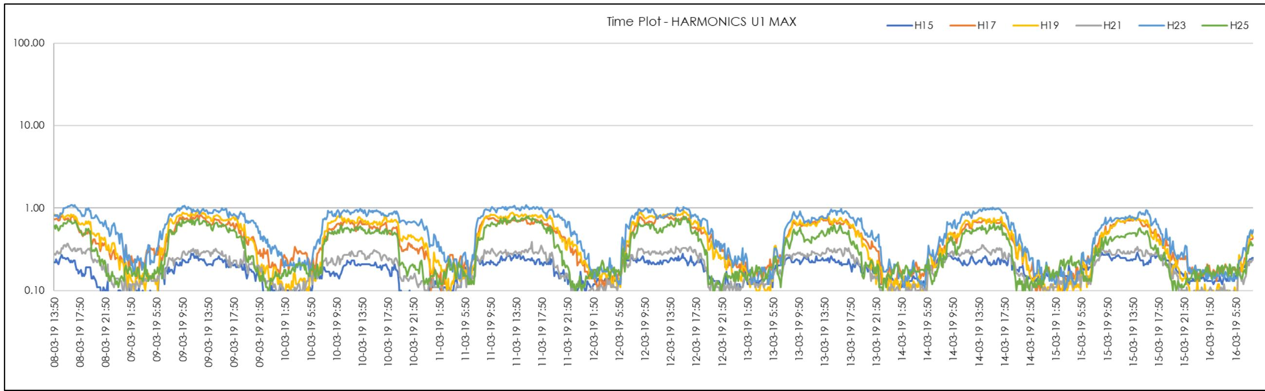
Figure 214 | STS4 Start Odd 15<sup>th</sup>-25<sup>th</sup> Harmonics (Red Phase)
