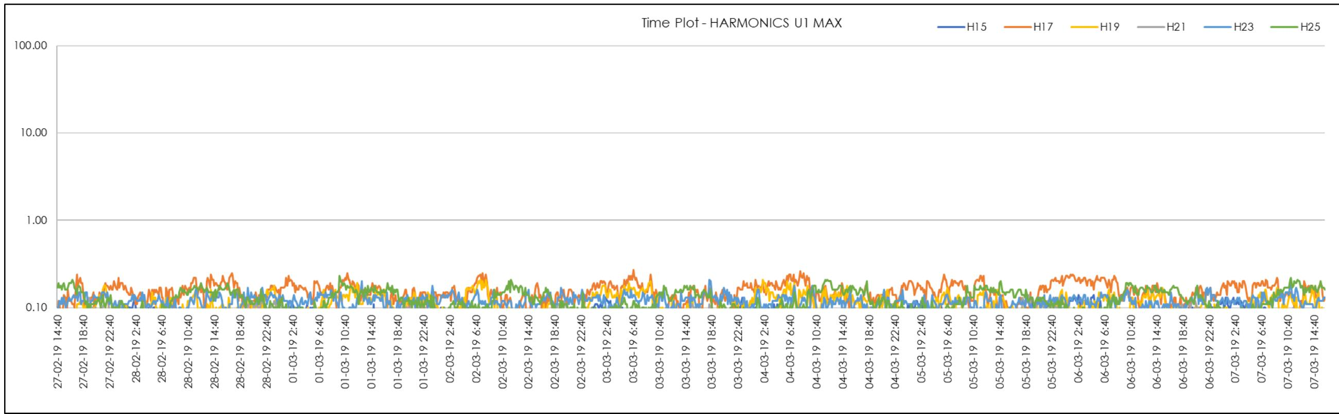
Figure 190 | STS2 End Odd 15<sup>th</sup>-25<sup>th</sup> Harmonics (Red Phase)
