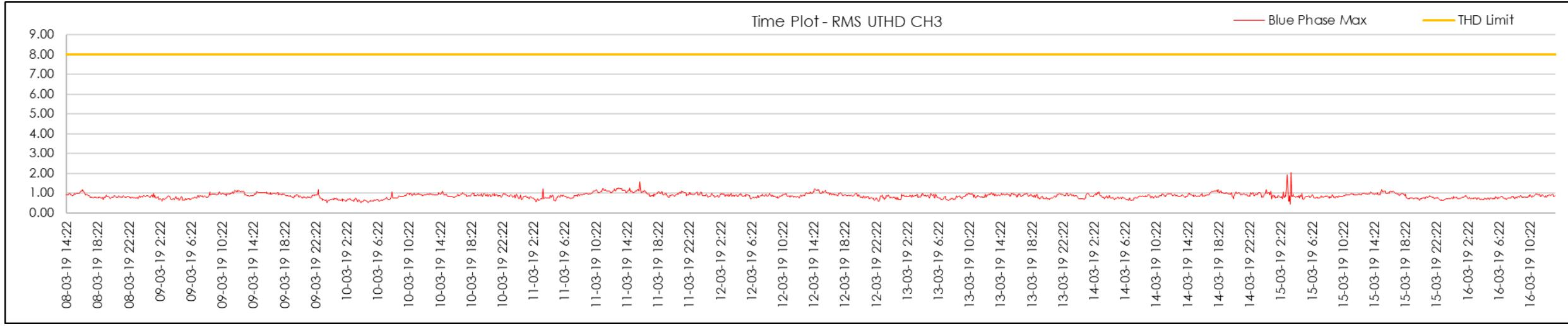
Figure 210 | STS4 End U-THD measurements (Blue Phase)
