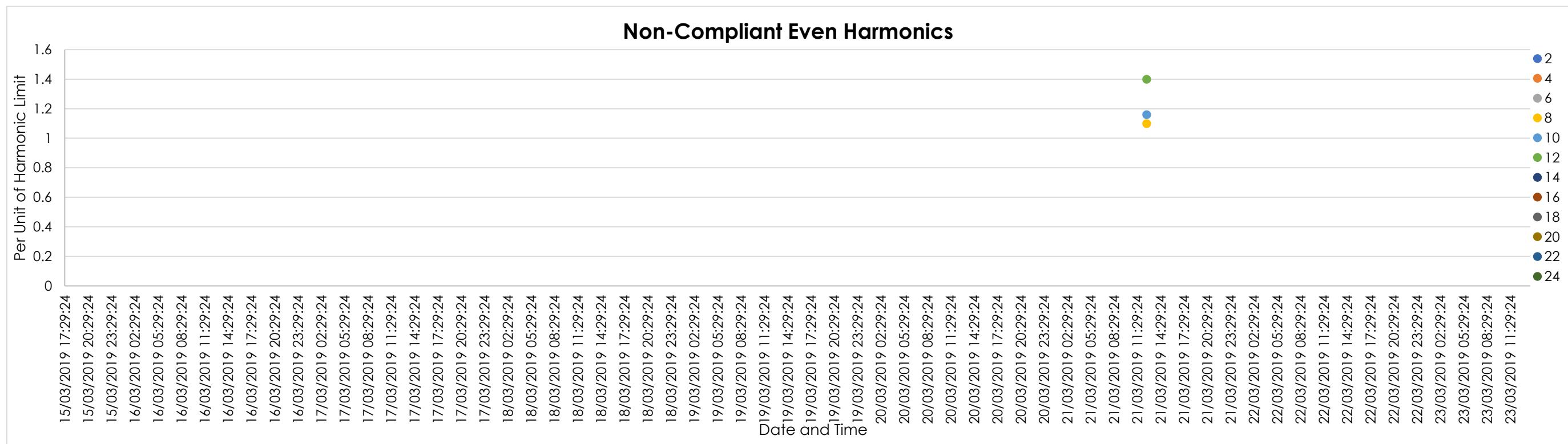
Figure 11 | TC4 Feeder (Start) - Non-Compliant Even Harmonics
