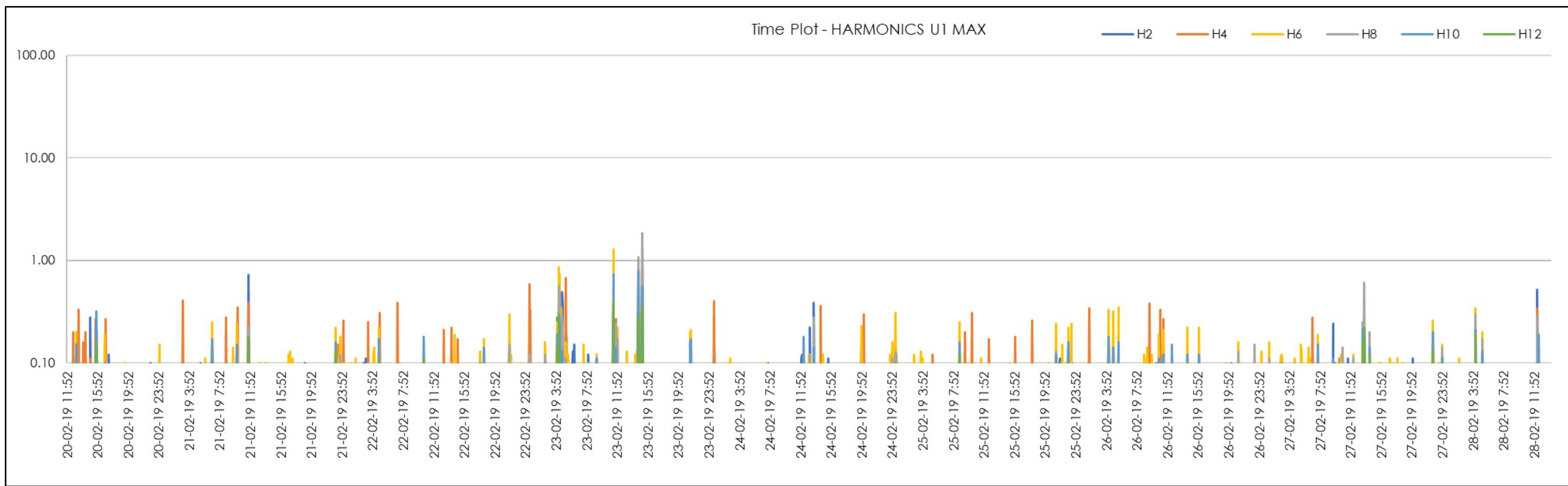
Figure 131 | TC4 End Even 2<sup>nd</sup>-12<sup>th</sup> Harmonics (Red Phase)
