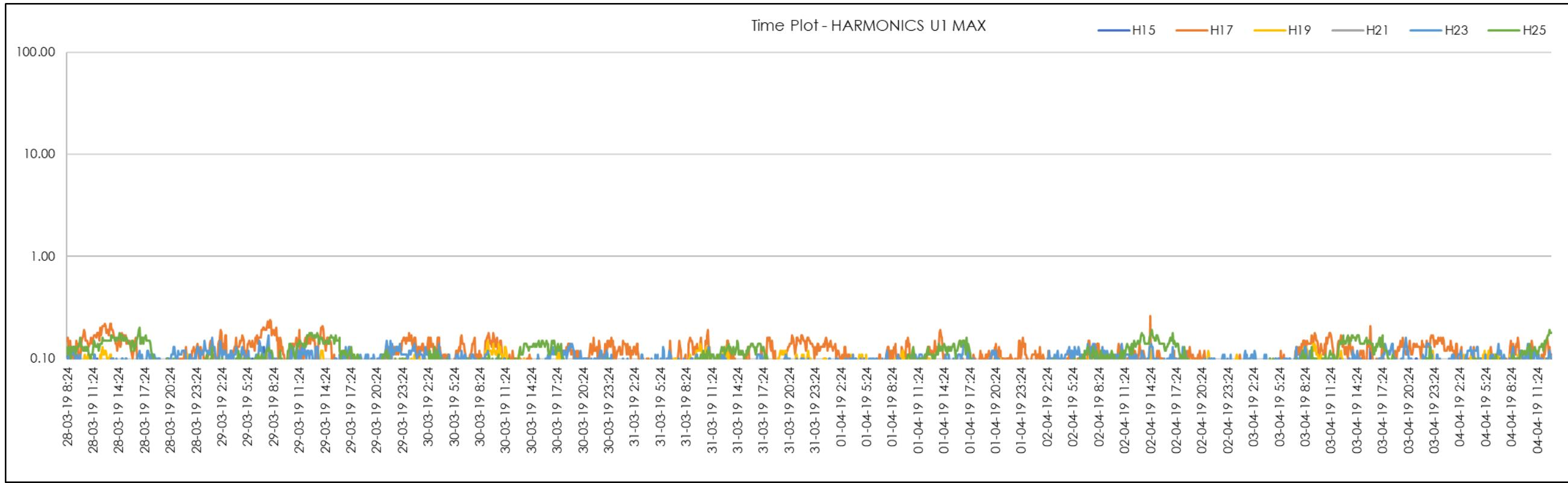
Figure 186 | STS2 Start Odd 15<sup>th</sup>-25<sup>th</sup> Harmonics (Red Phase)
