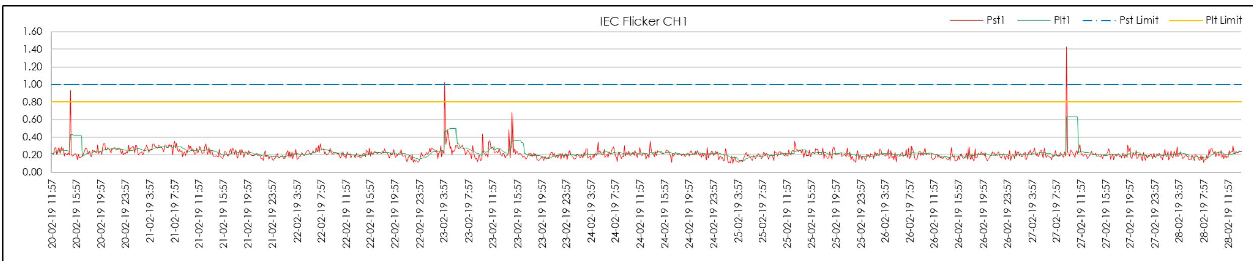
Figure 110 | TC4 End Flicker measurements (Red Phase)
