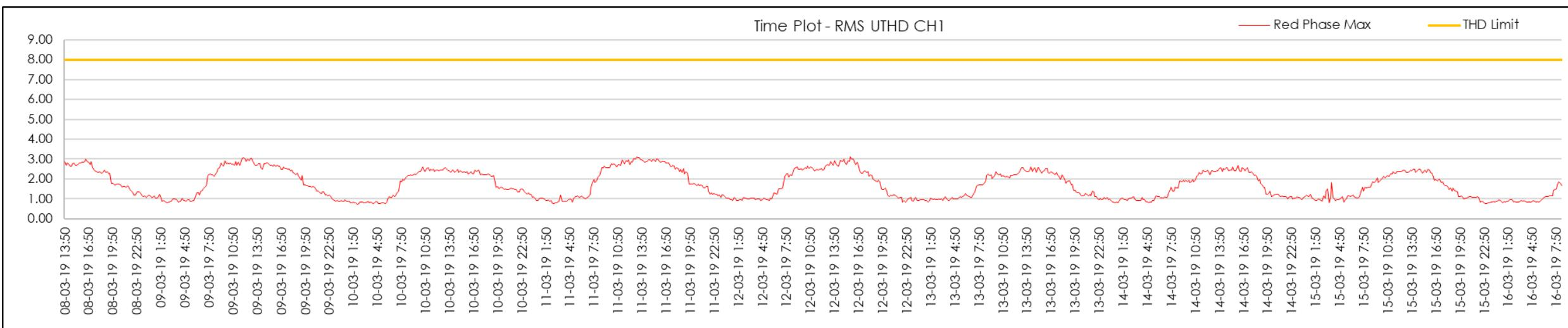
Figure 205 | STS4 Start U-THD measurements (Red Phase)
