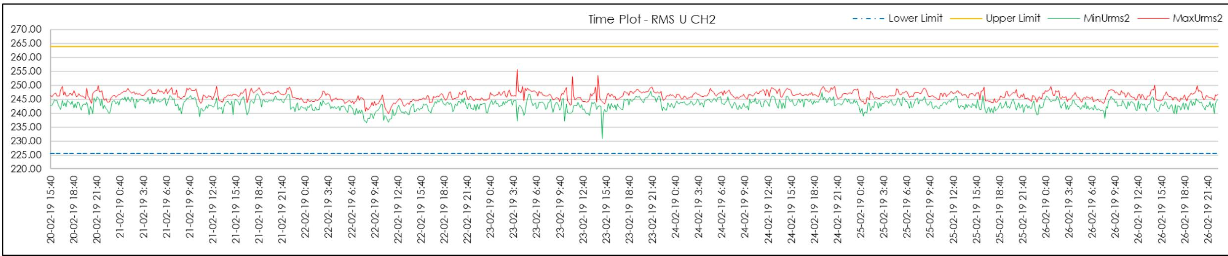
Figure 142 | STS1 Start Voltage measurements (White Phase)
