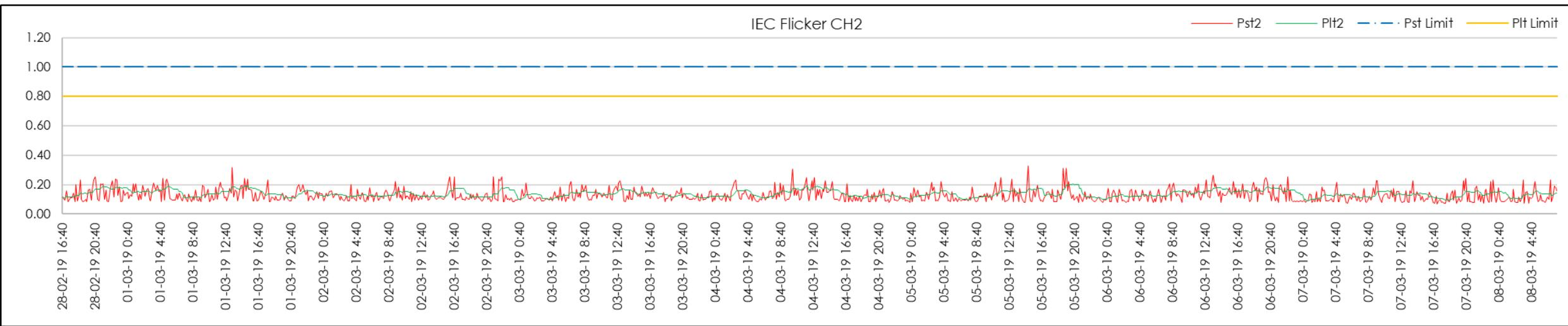
Figure 223 | STS6 End Flicker measurements (White Phase)
