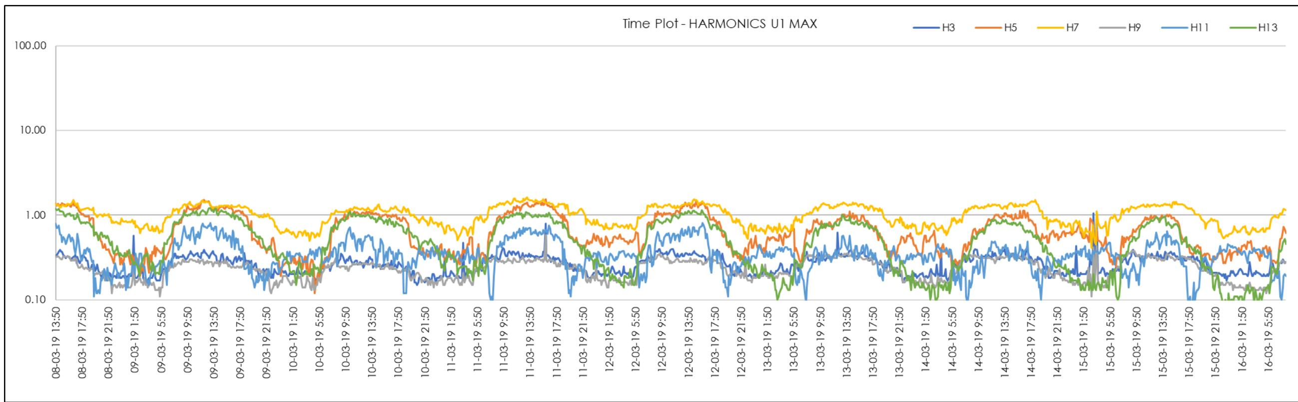
Figure 213 | STS4 Start Odd 3<sup>rd</sup>-13<sup>th</sup> Harmonics (Red Phase)
