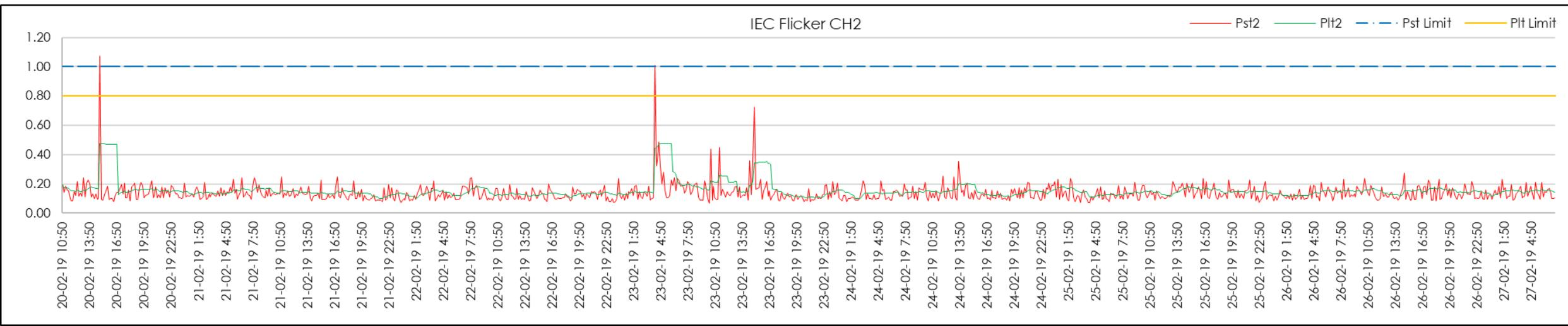
Figure 83 | TC3 End Flicker measurements (White Phase)
