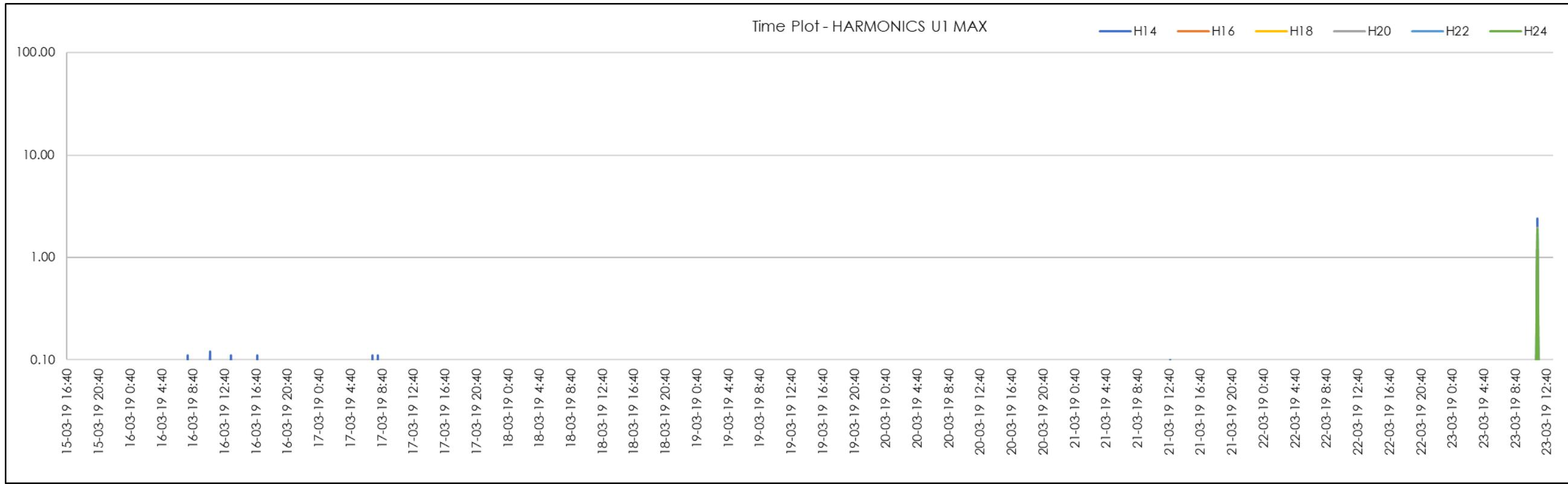
Figure 72 | TC2 Start Even 14<sup>th</sup>-24<sup>th</sup> Harmonics (Red Phase)
