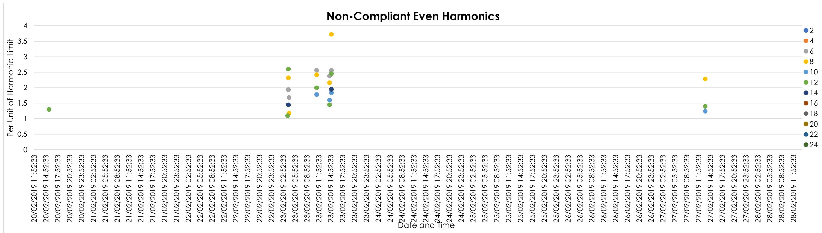
Figure 12 | TC4 Feeder (End) - Non-Compliant Even Harmonics
