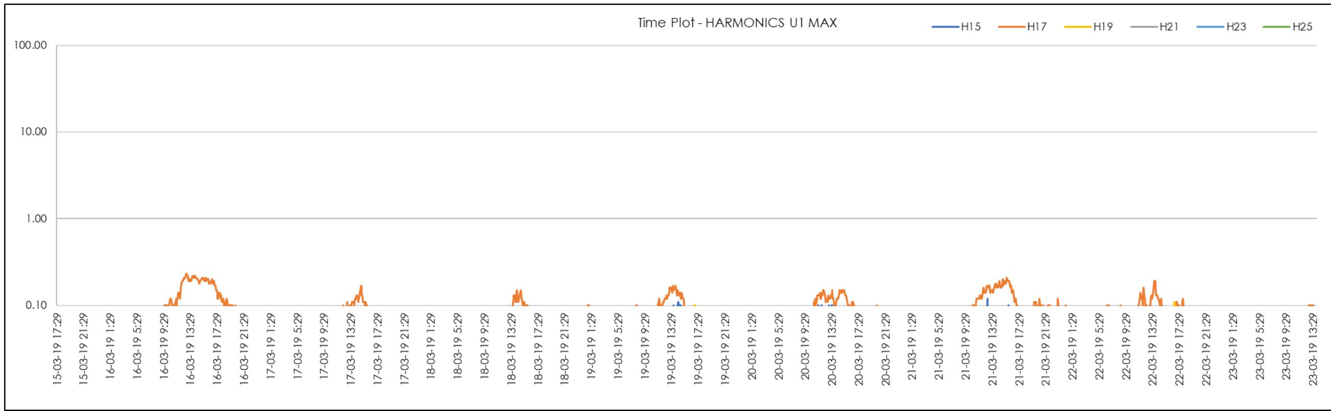
Figure 130 | TC4 Start Odd 15<sup>th</sup>-25<sup>th</sup> Harmonics (Red Phase)
