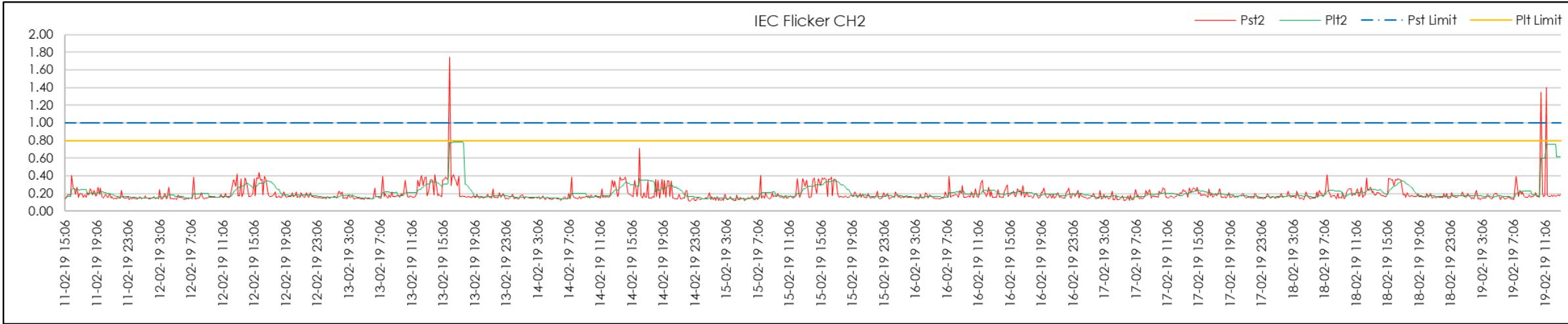
Figure 24 | TC1 Start Flicker measurements (White Phase)
