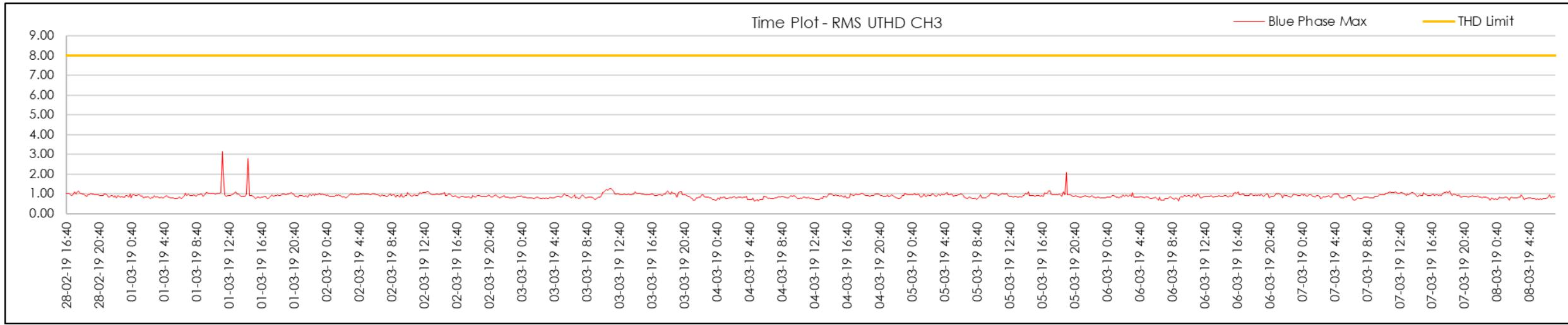
Figure 238 | STS6 End U-THD measurements (Blue Phase)
