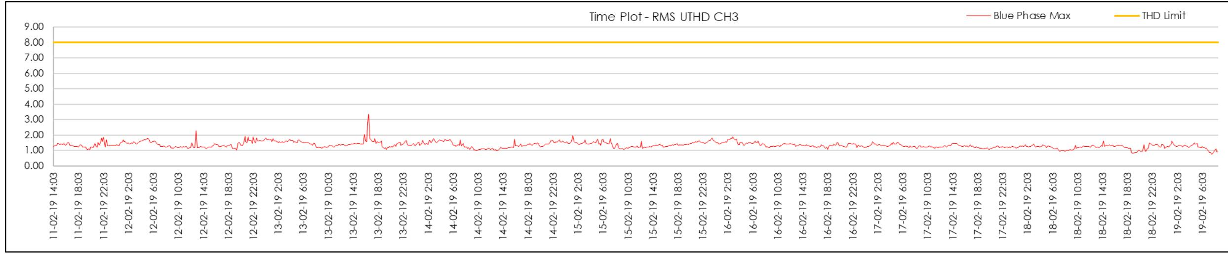
Figure 42 | TC1 End U-THD measurements (Blue Phase)
