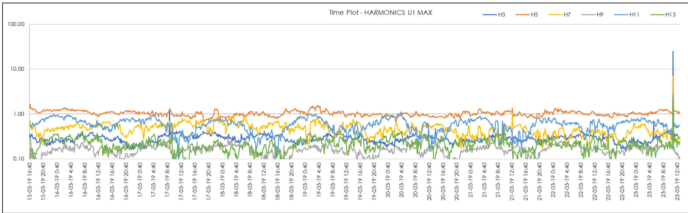
Figure 73 | TC2 Start Odd 3<sup>rd</sup>-13<sup>th</sup> Harmonics (Red Phase)
