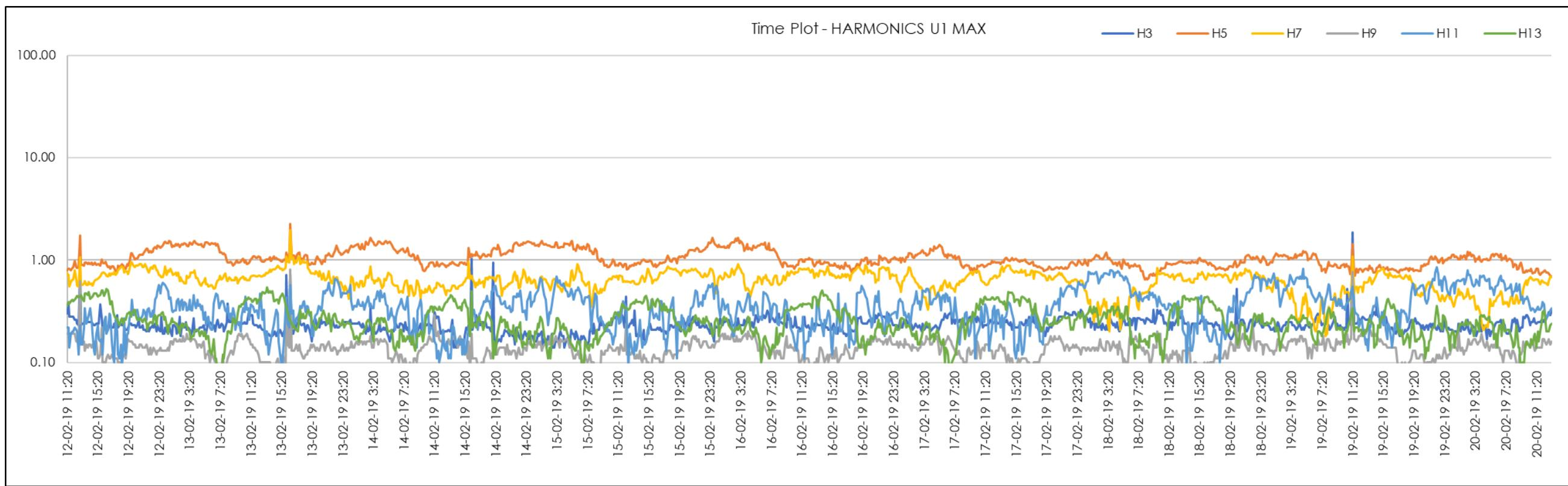
Figure 77 | TC2 End Odd 3<sup>rd</sup>-13<sup>th</sup> Harmonics (Red Phase)
