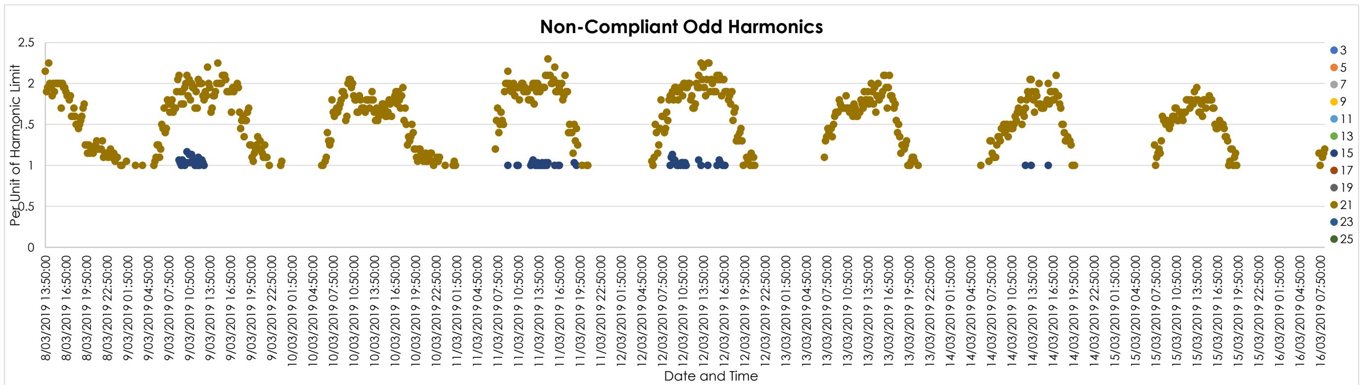
Figure 19 | STS4 Feeder (Start) - Non-Compliant Odd Harmonics
