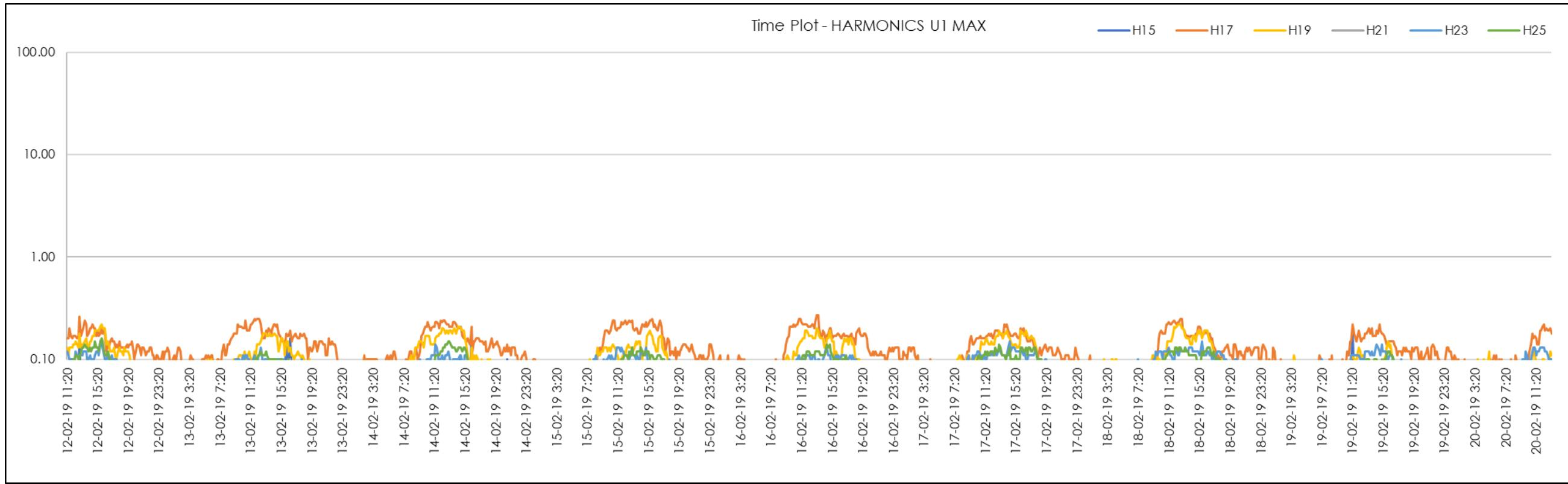
Figure 78 | TC2 End Odd 15<sup>th</sup>-25<sup>th</sup> Harmonics (Red Phase)
