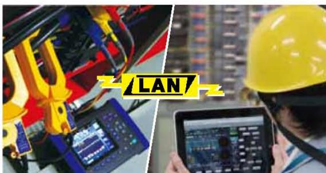
Conduct off-site remote control with a tablet PC using a wireless LAN router
