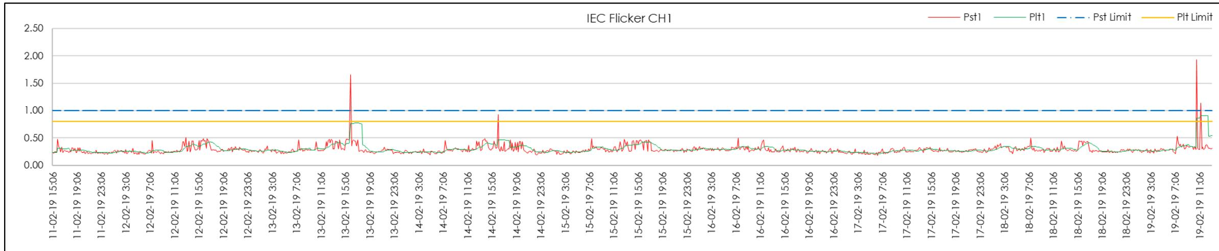
Figure 23 | TC1 Start Flicker measurements (Red Phase)
