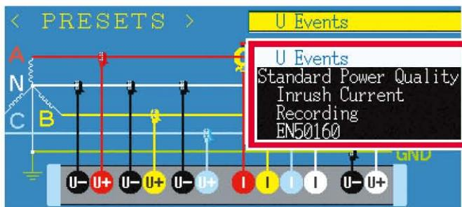
Simply choose the course based on the measurement objective and the necessary configurations will be set automatically.
