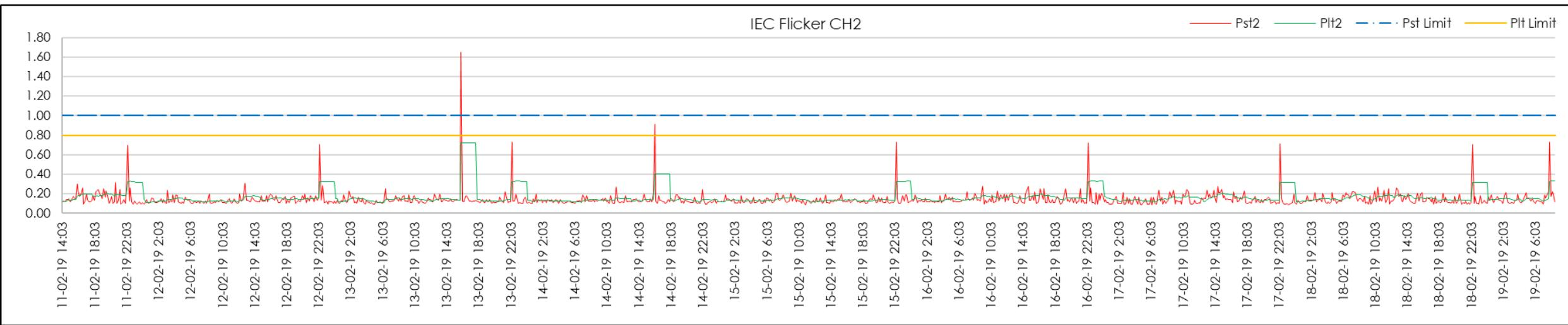
Figure 27 | TC1 End Flicker measurements (White Phase)
