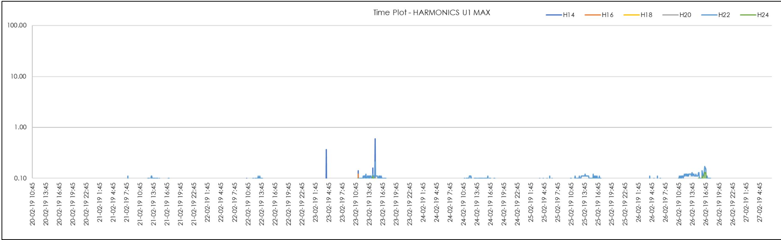
Figure 104 | TC3 End Even 14<sup>th</sup>-24<sup>th</sup> Harmonics (Red Phase)
