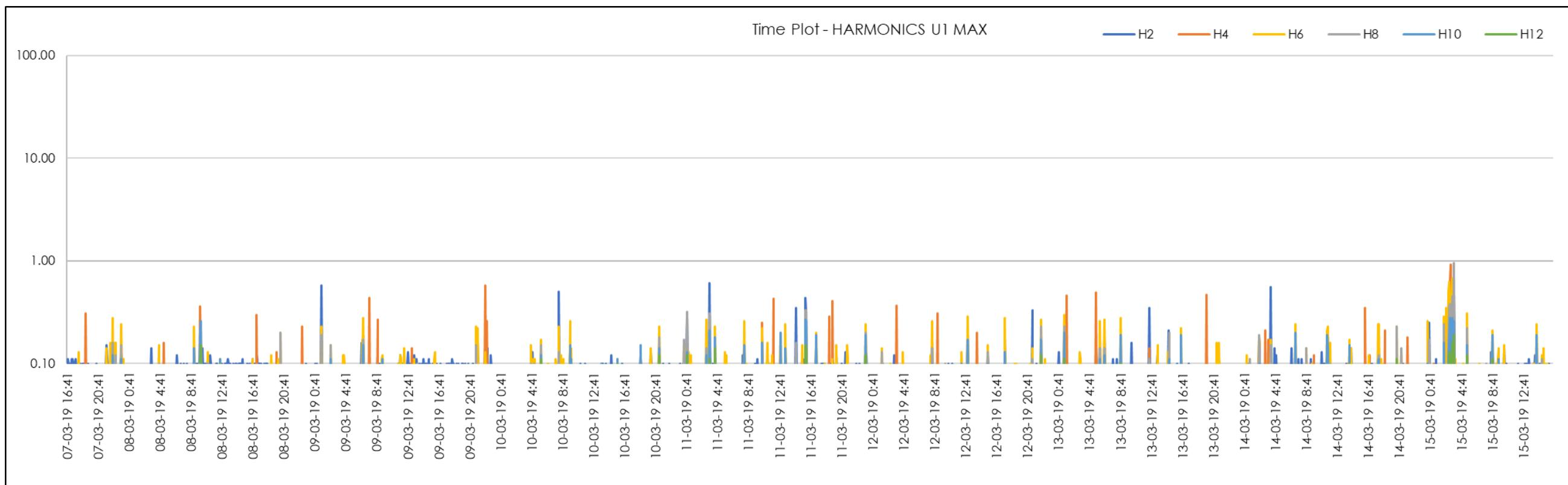
Figure 159 | STS1 End Even 2<sup>nd</sup>-12<sup>th</sup> Harmonics (Red Phase)
