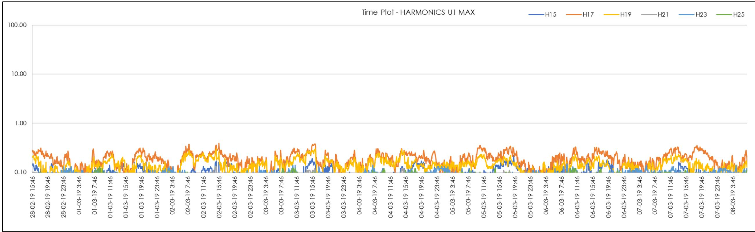
Figure 242 | STS6 Start Odd 15<sup>th</sup>-25<sup>th</sup> Harmonics (Red Phase)
