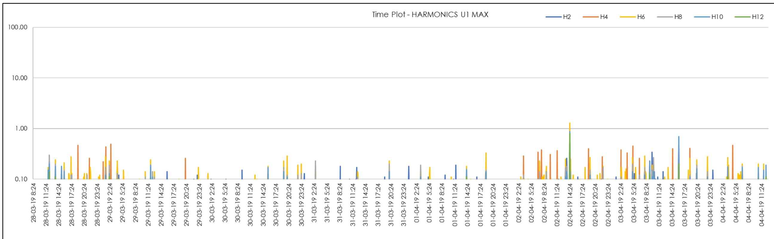
Figure 183 | STS2 Start Even 2<sup>nd</sup>-12<sup>th</sup> Harmonics (Red Phase)
