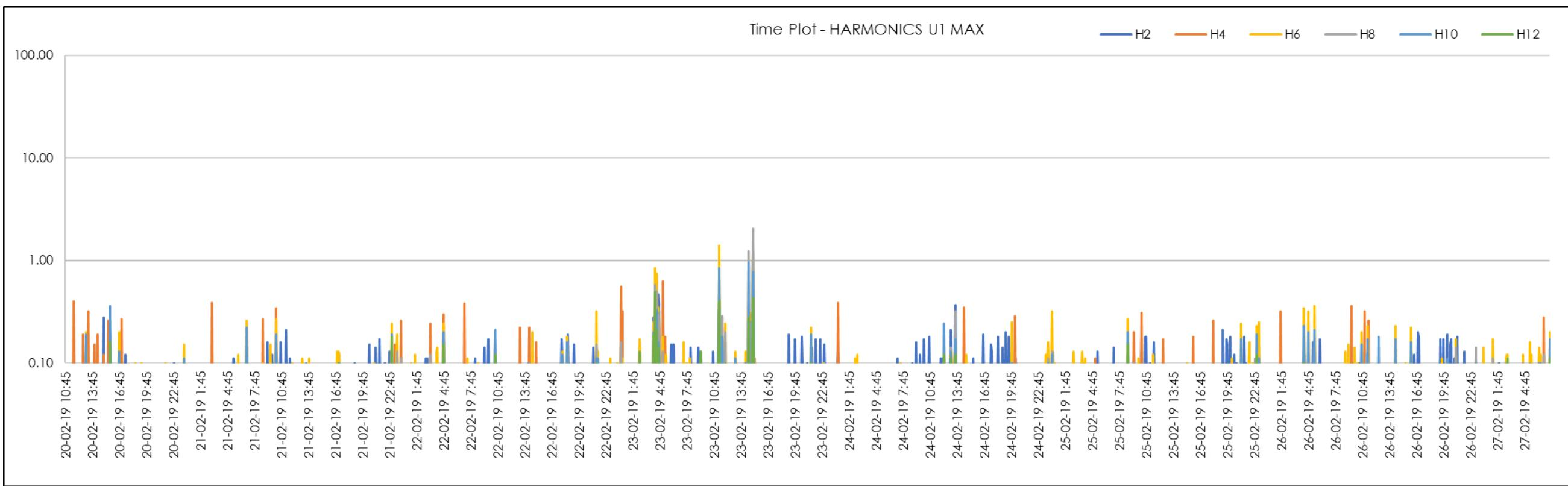
Figure 103 | TC3 End Even 2<sup>nd</sup>-12<sup>th</sup> Harmonics (Red Phase)
