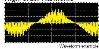
The PW3198 is the first power quality analyzer that can measure the high-order harmonic component of up to 80 kHz.
