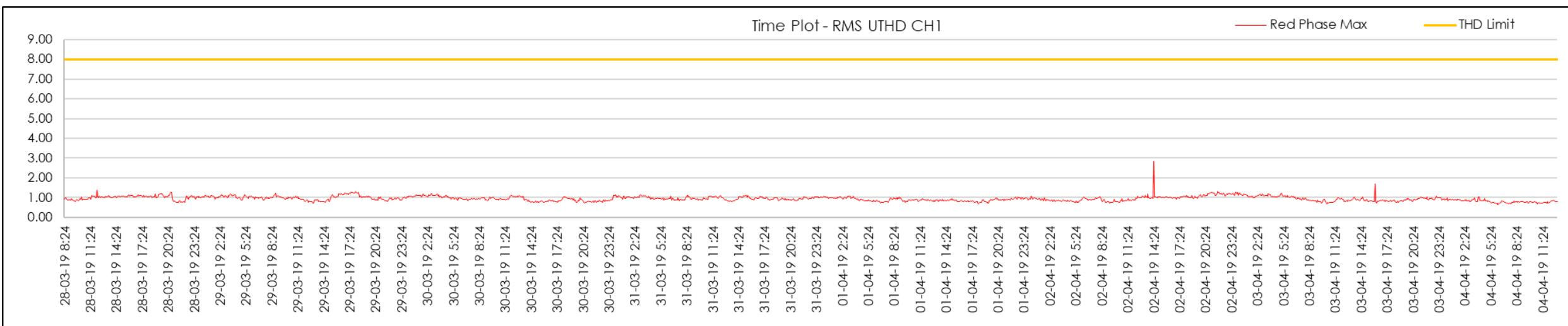
Figure 177 | STS2 Start U-THD measurements (Red Phase)
