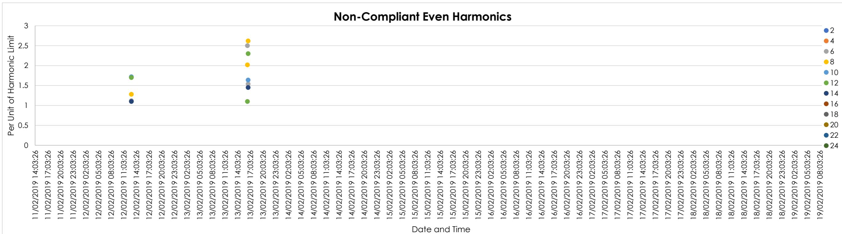
Figure 4 | Feeder TC1 (End) - Non-Compliant Even Harmonics
