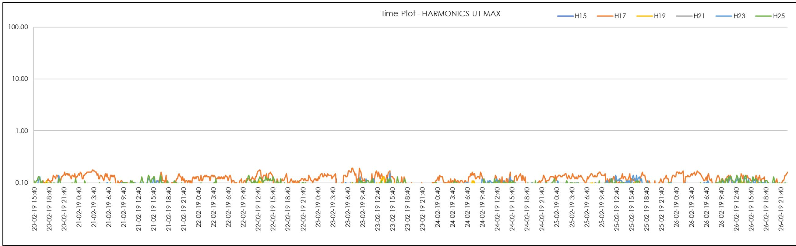
Figure 158 | STS1 Start Odd 15<sup>th</sup>-25<sup>th</sup> Harmonics (Red Phase)
