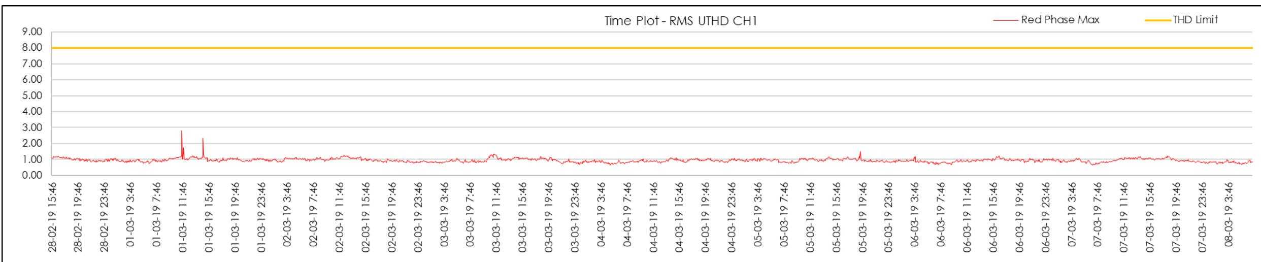
Figure 233 | STS6 Start U-THD measurements (Red Phase)
