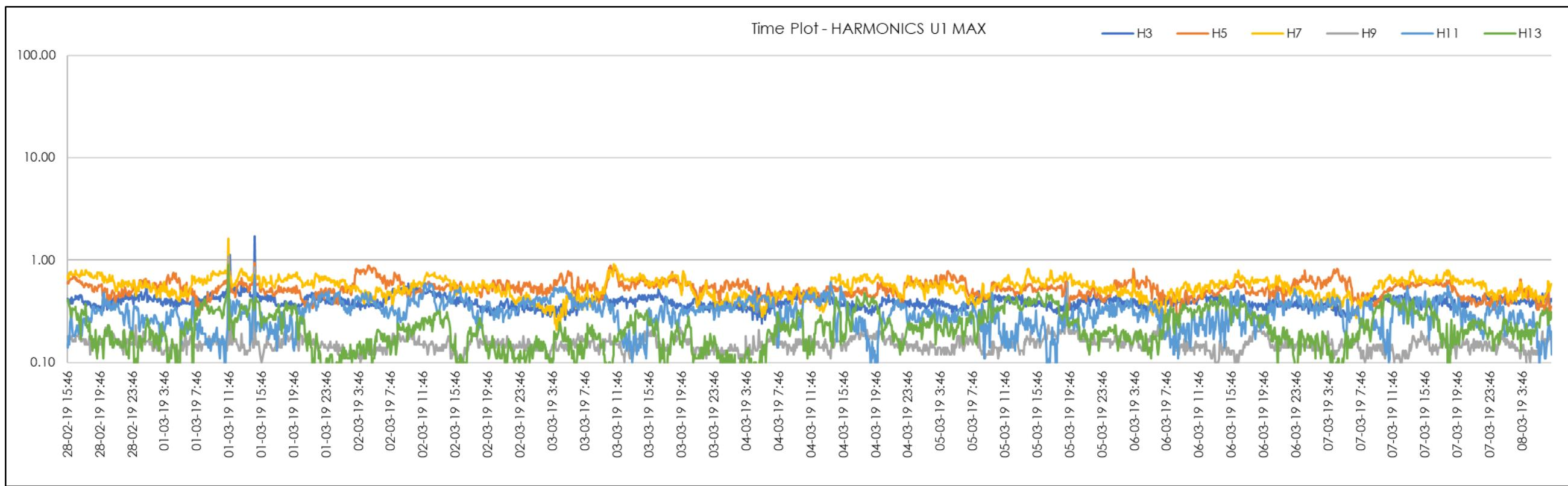
Figure 241 | STS6 Start Odd 3<sup>rd</sup>-13<sup>th</sup> Harmonics (Red Phase)
