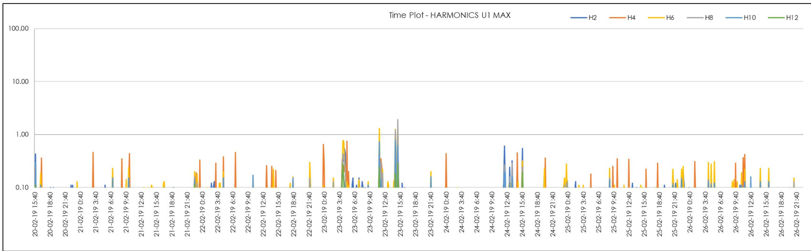
Figure 155 | STS1 Start Even 2<sup>nd</sup>-12<sup>th</sup> Harmonics (Red Phase)
