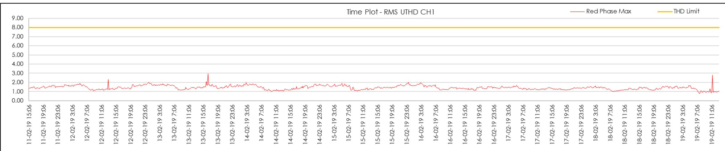
Figure 37 | TC1 Start U-THD measurements (Red Phase)
