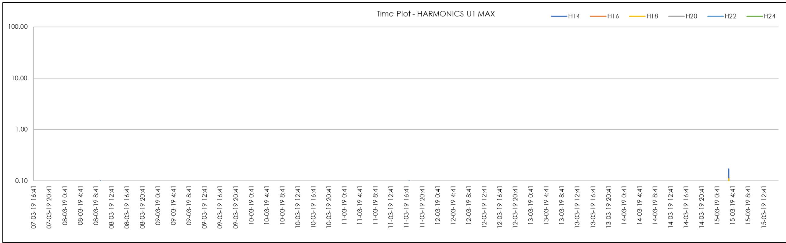
Figure 160 | STS1 End Even 14<sup>th</sup>-24<sup>th</sup> Harmonics (Red Phase)
