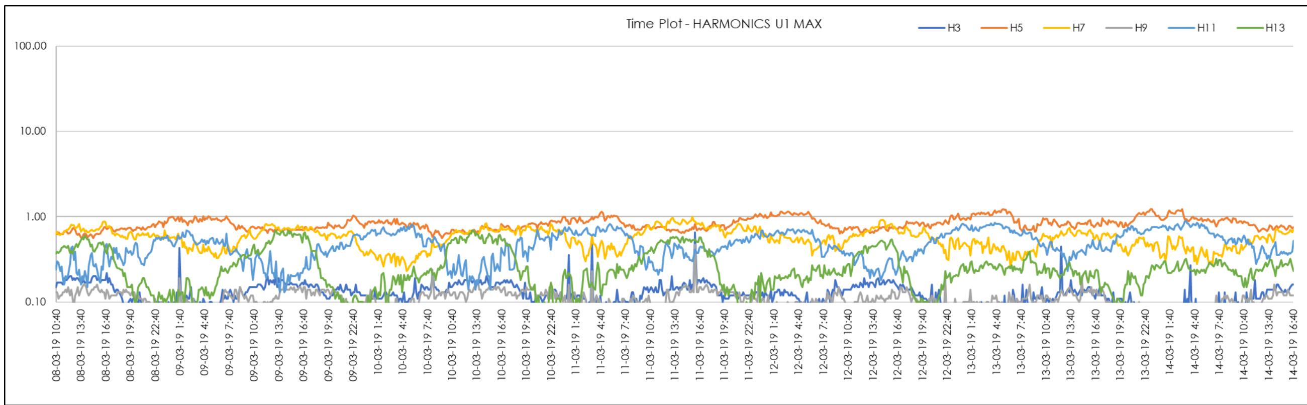
Figure 101 | TC3 Start Odd 3<sup>rd</sup>-13<sup>th</sup> Harmonics (Red Phase)
