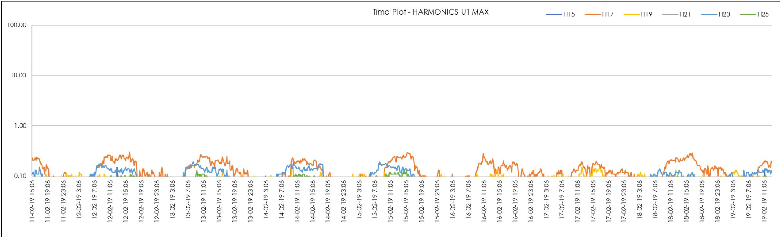
Figure 46 | TC1 Start Odd 15<sup>th</sup>-25<sup>th</sup> Harmonics (Red Phase)
