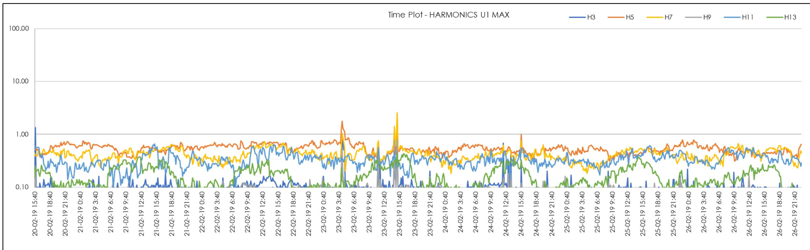
Figure 157 | STS1 Start Odd 3<sup>rd</sup>-13<sup>th</sup> Harmonics (Red Phase)
