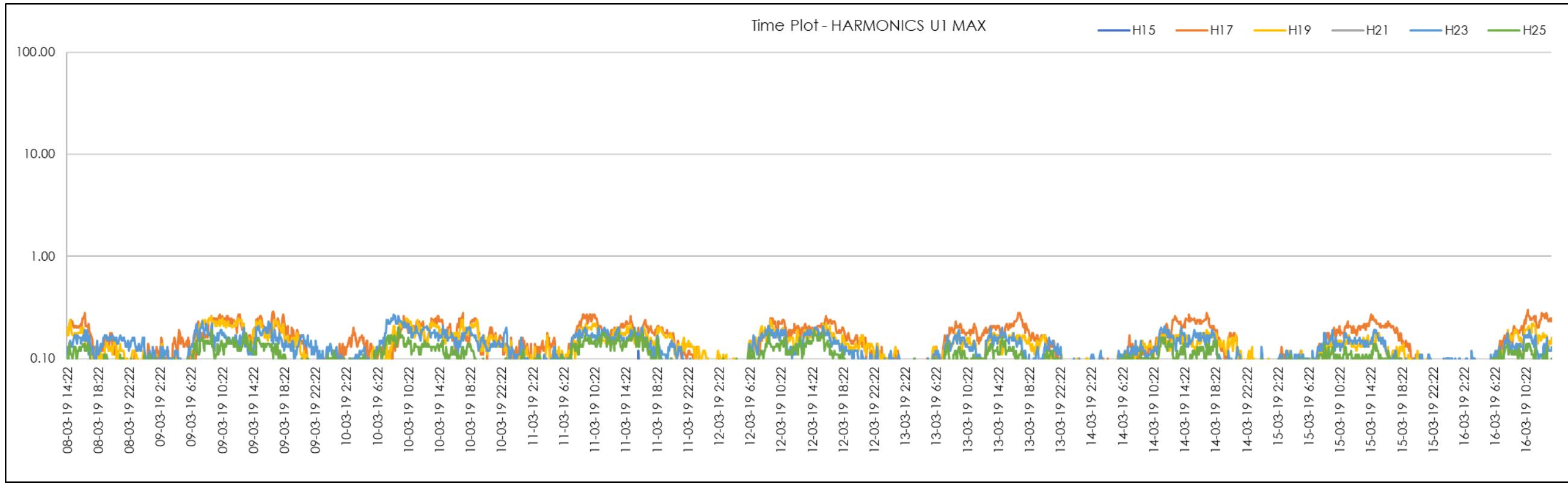
Figure 218 | STS4 End Odd 15<sup>th</sup>-25<sup>th</sup> Harmonics (Red Phase)
