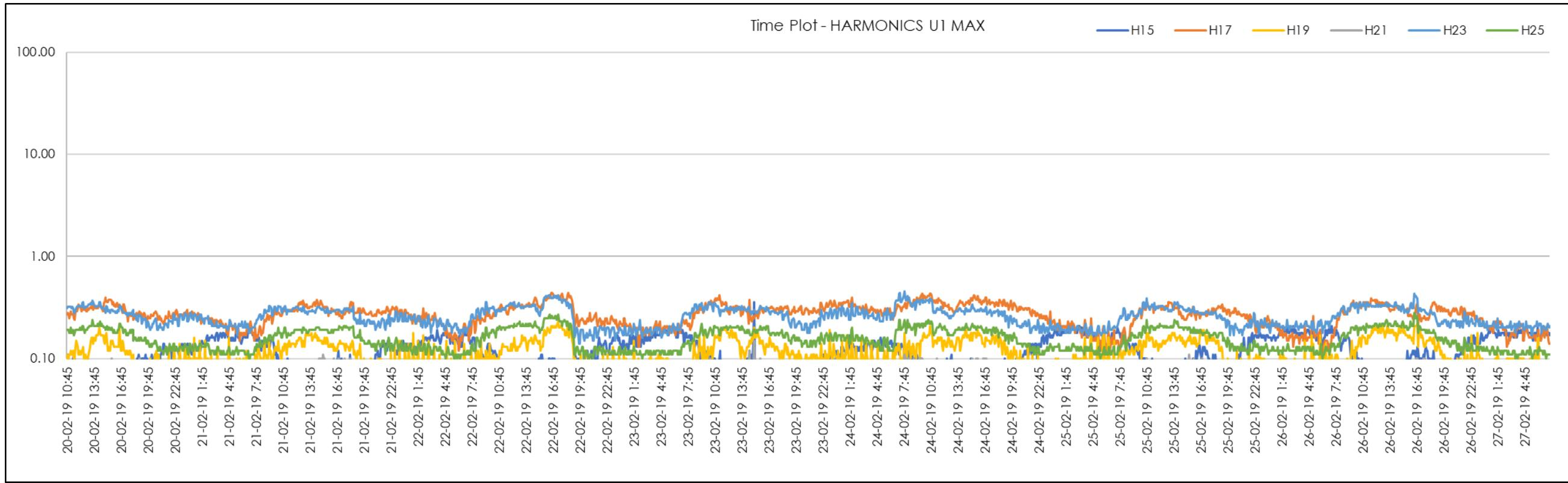
Figure 106 | TC3 End Odd 15<sup>th</sup>-25<sup>th</sup> Harmonics (Red Phase)
