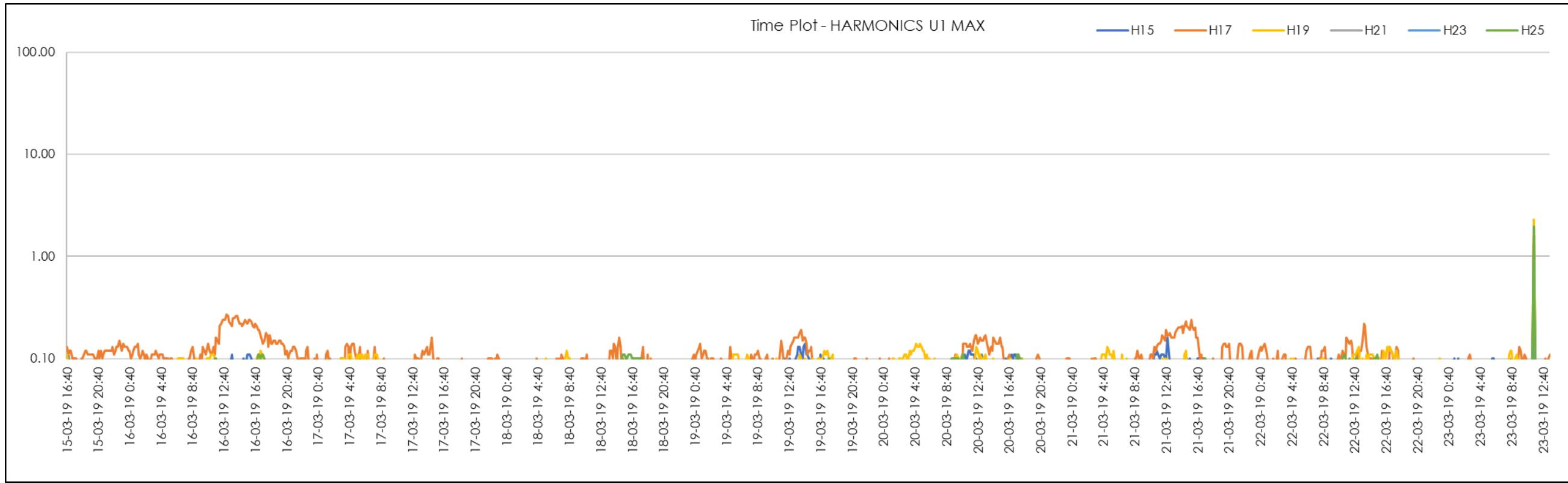
Figure 74 | TC2 Start Odd 15<sup>th</sup>-25<sup>th</sup> Harmonics (Red Phase)
