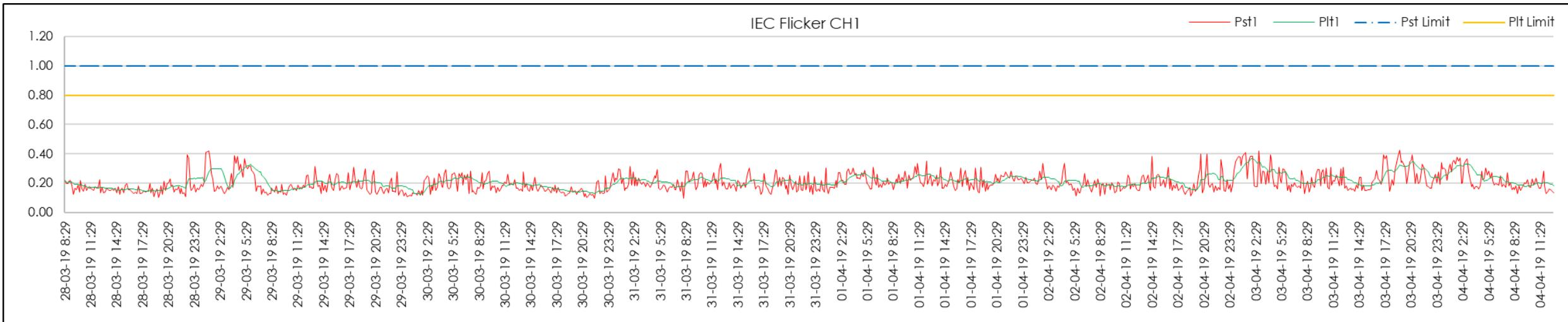
Figure 163 | STS2 Start Flicker measurements (Red Phase)
