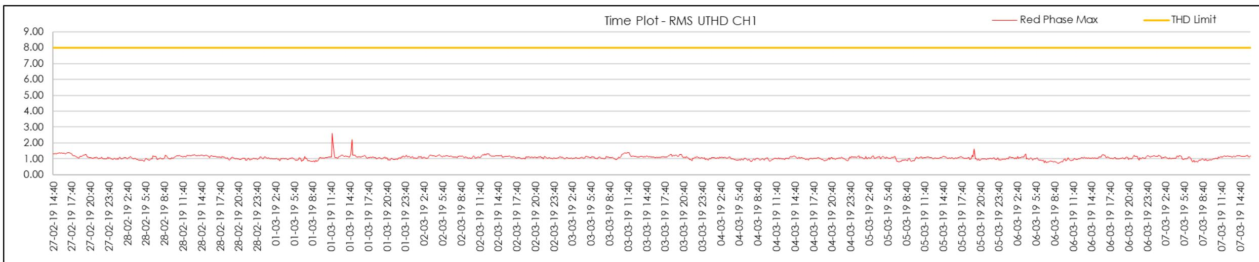
Figure 180 | STS2 End U-THD measurements (Red Phase)
