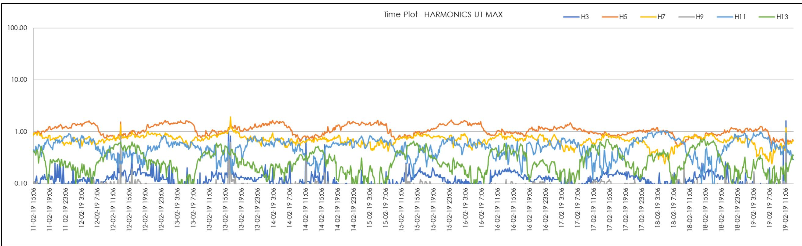
Figure 45 | TC1 Start Odd 3<sup>rd</sup>-13<sup>th</sup> Harmonics (Red Phase)
