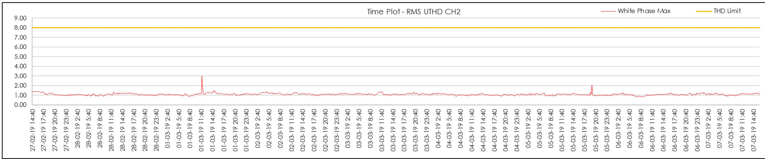
**Figure 181 | STS2 End U-THD measurements (White Phase)**
