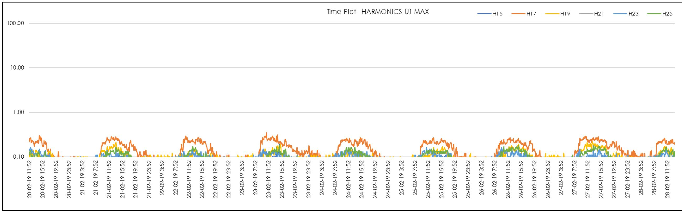
Figure 134 | TC4 End Odd 15<sup>th</sup>-25<sup>th</sup> Harmonics (Red Phase)
