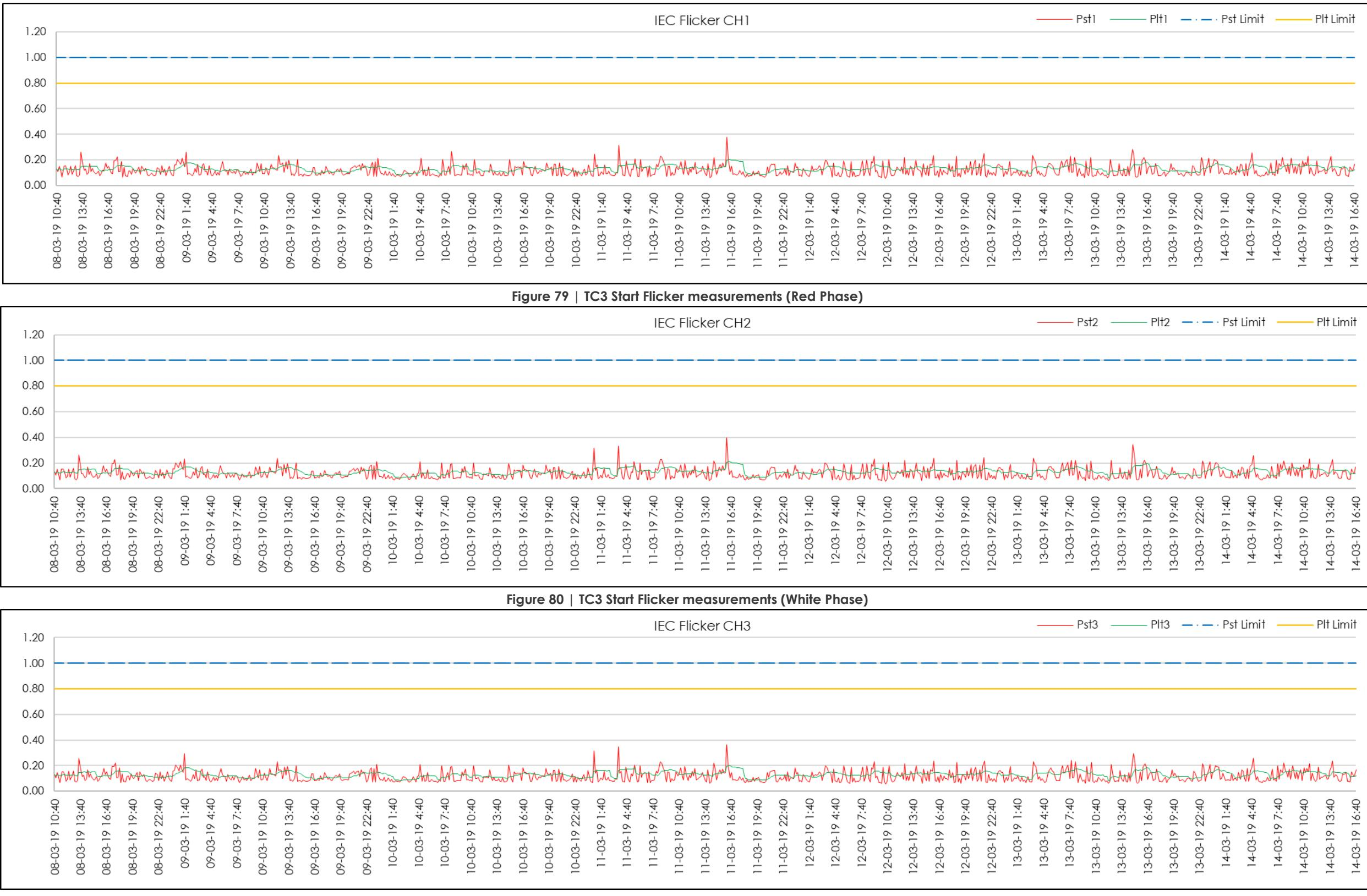
Figure 79 | TC3 Start Flicker measurements (Red Phase)
