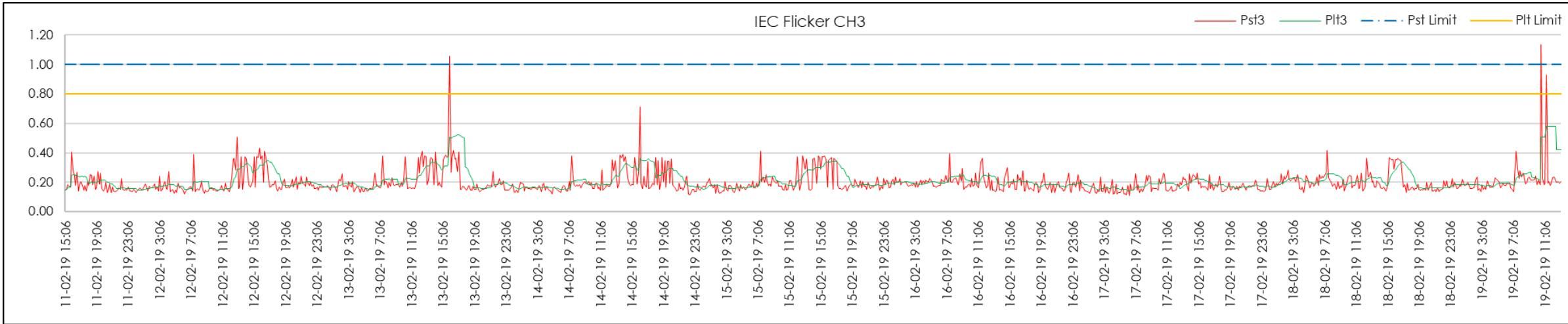
Figure 25 | TC1 Start Flicker measurements (Blue Phase)
