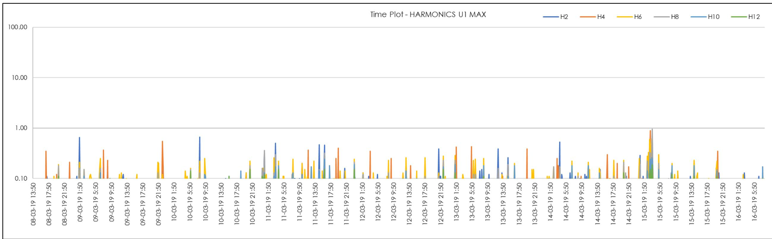
Figure 211 | STS4 Start Even 2<sup>nd</sup>-12<sup>th</sup> Harmonics (Red Phase)
