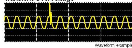
Transient overvoltage can also be measured in a range between the maximum 6,000 V and minimum 1  $\mu$ s (2 MS/s).
