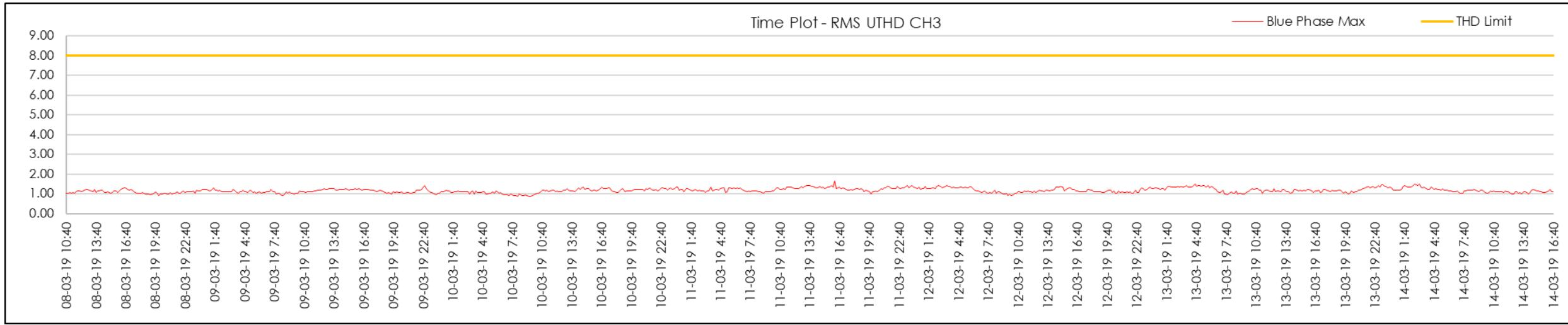
Figure 95 | TC3 Start U-THD measurements (Blue Phase)
