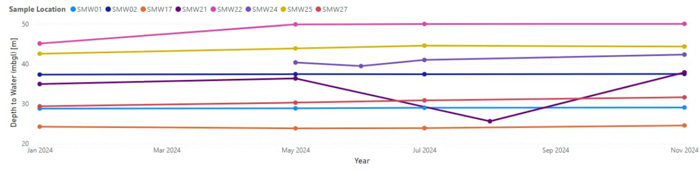
Figure 2: Groundwater level monitoring data around GMW Pit
