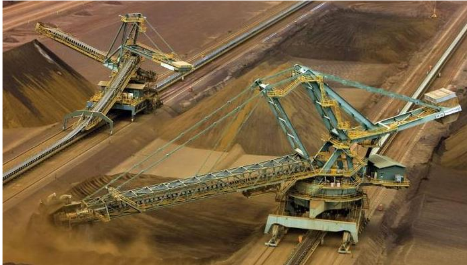
Figure 8-2 Picture of a stacker and reclaimer with their associated conveyor belt system
