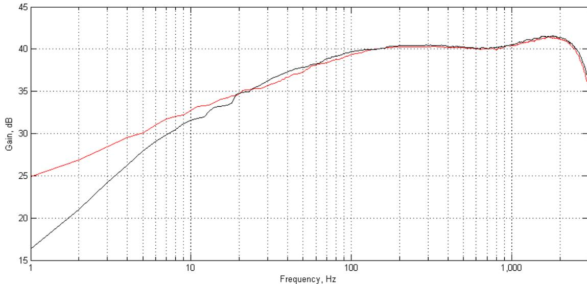
Figure 2: System gain (dB with frequency as determined from white noise calibration before deployment) for dataset 2972 (red) and 2973 (black).
