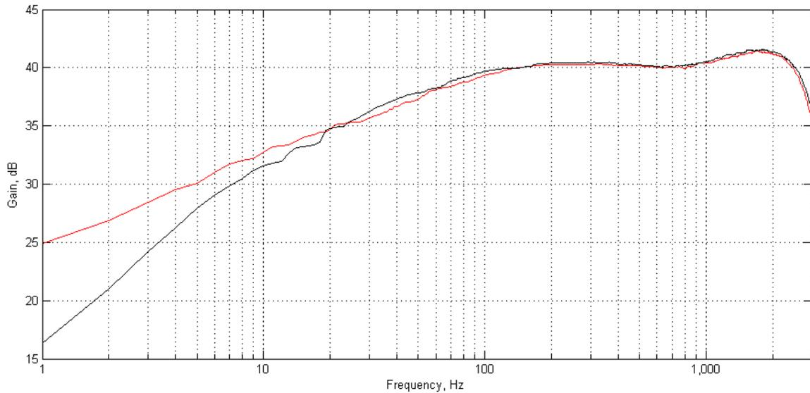
Figure 2: System gain (dB with frequency as determined from white noise calibration before deployment) for dataset 2972 (red) and 2973 (black).
