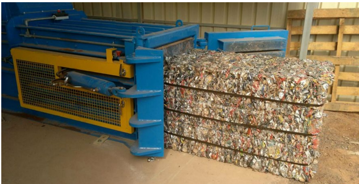
Plate 8.3 | On-site bailing press
