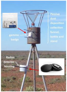
Figure 2-2: Radiation monitoring equipment
