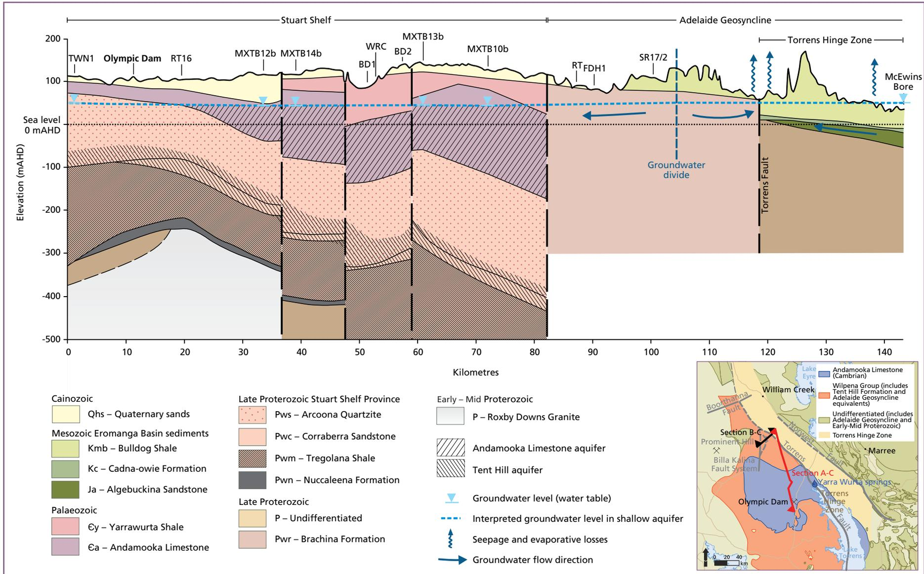
Figure 12.2 Cross-section A-C showing interpreted hydrostratigraphic and structural relationships north of Olympic Dam toward Billa Kalina spring
