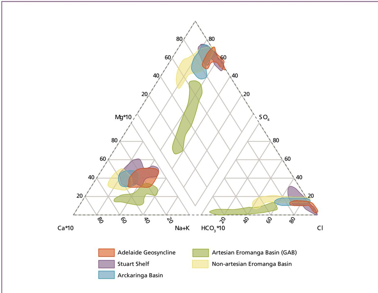
Figure 12.6 Piper tri-linear plot showing regional major ion data for different groundwater systems
