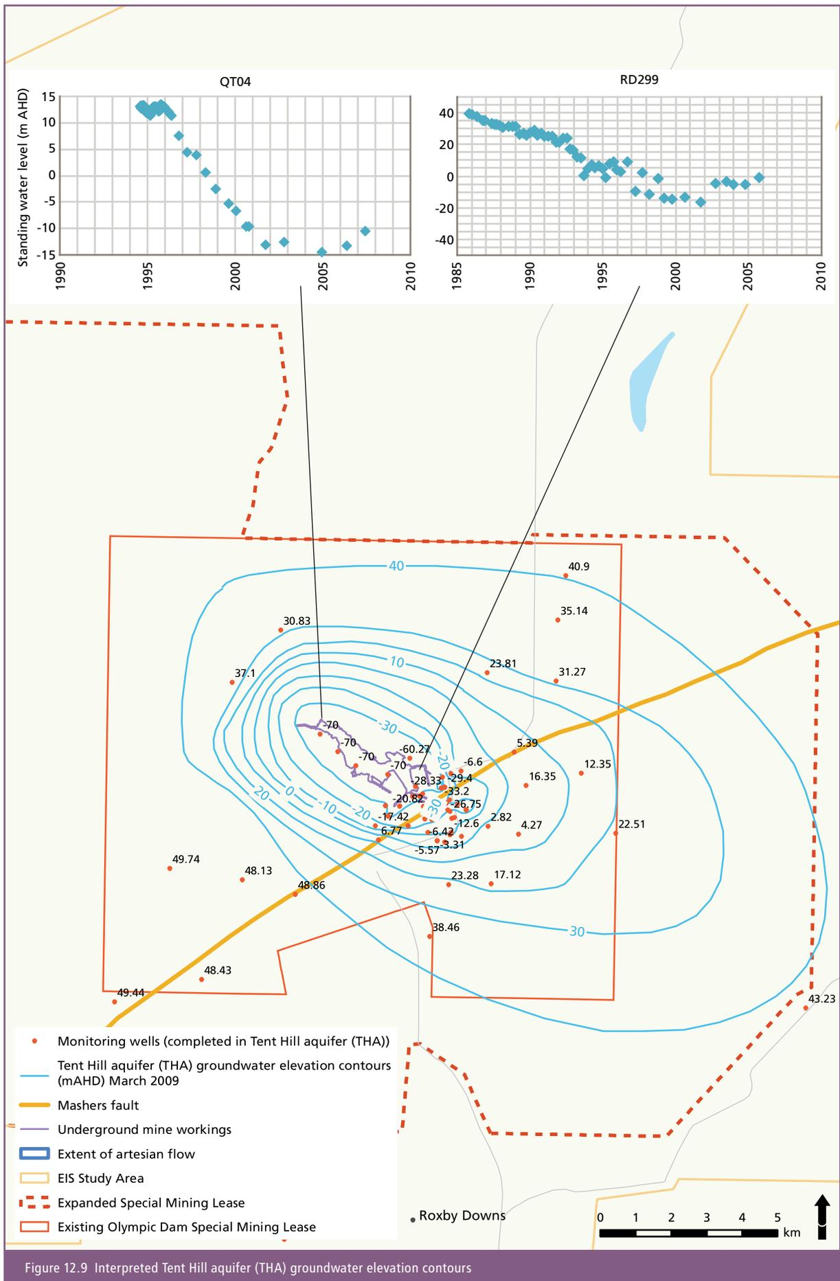
Figure 12.9 Interpreted Tent Hill aquifer (THA) groundwater elevation contours
