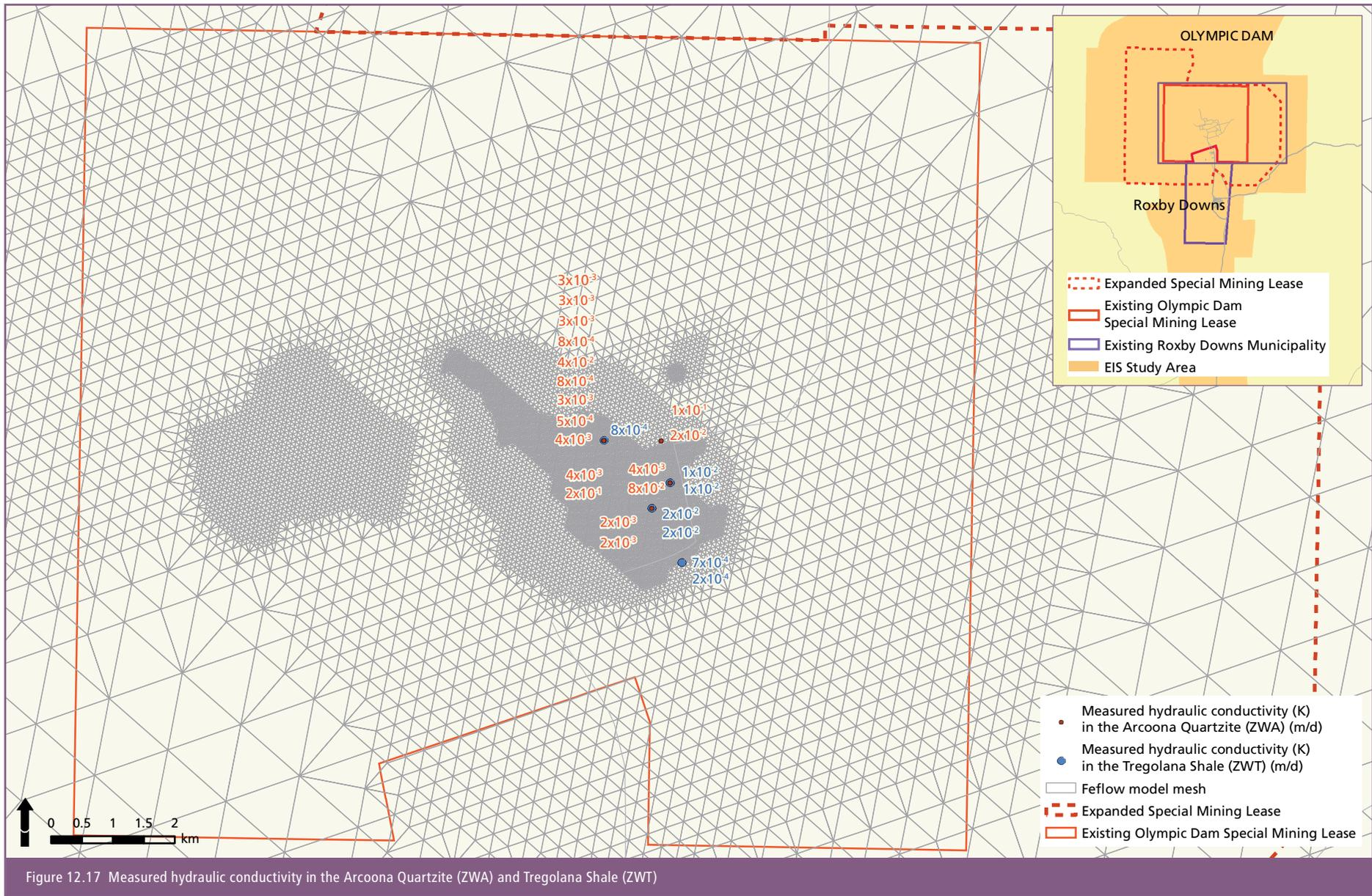
Figure 12.17 Measured hydraulic conductivity in the Arcoona Quartzite (ZWA) and Tregolana Shale (ZWT)
