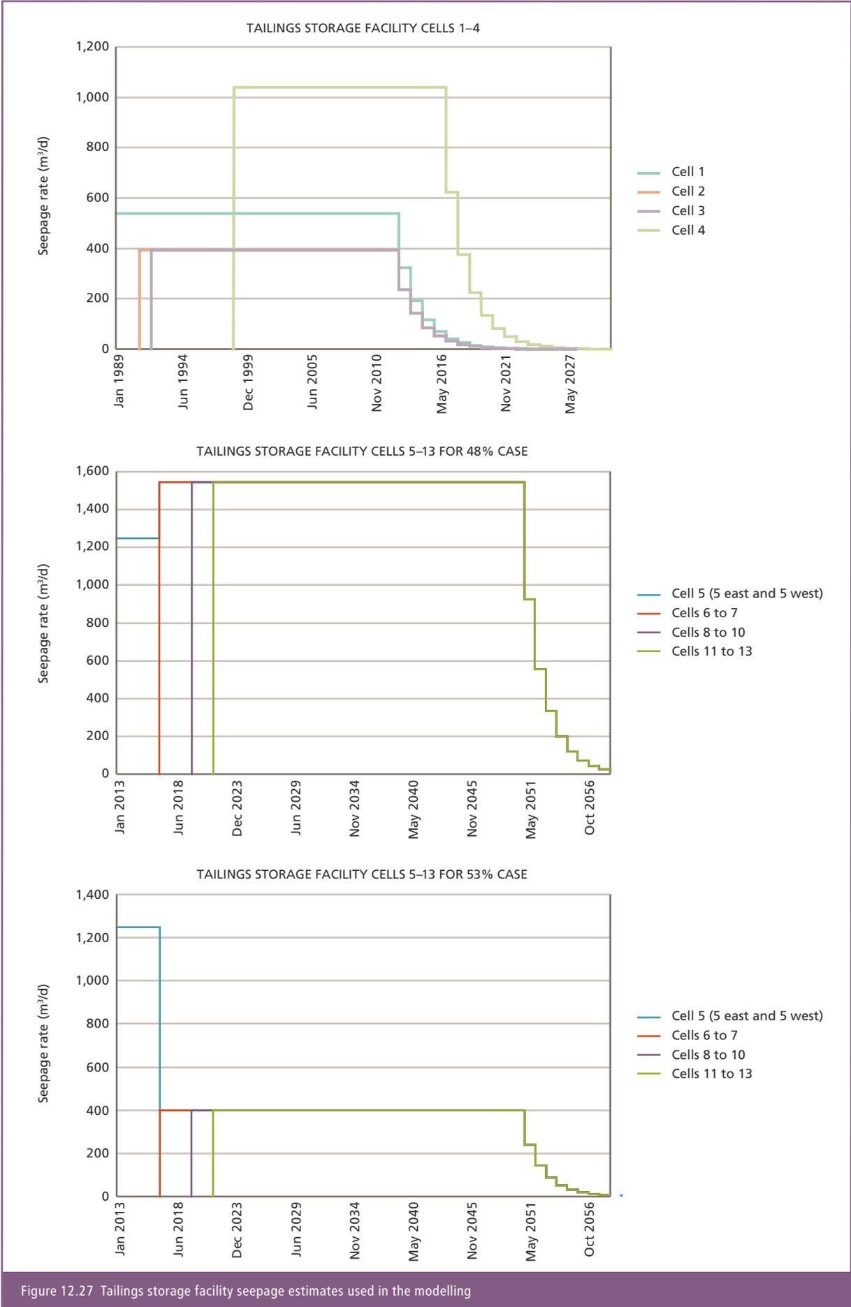
Figure 12.27 Tailings storage facility seepage estimates used in the modelling
