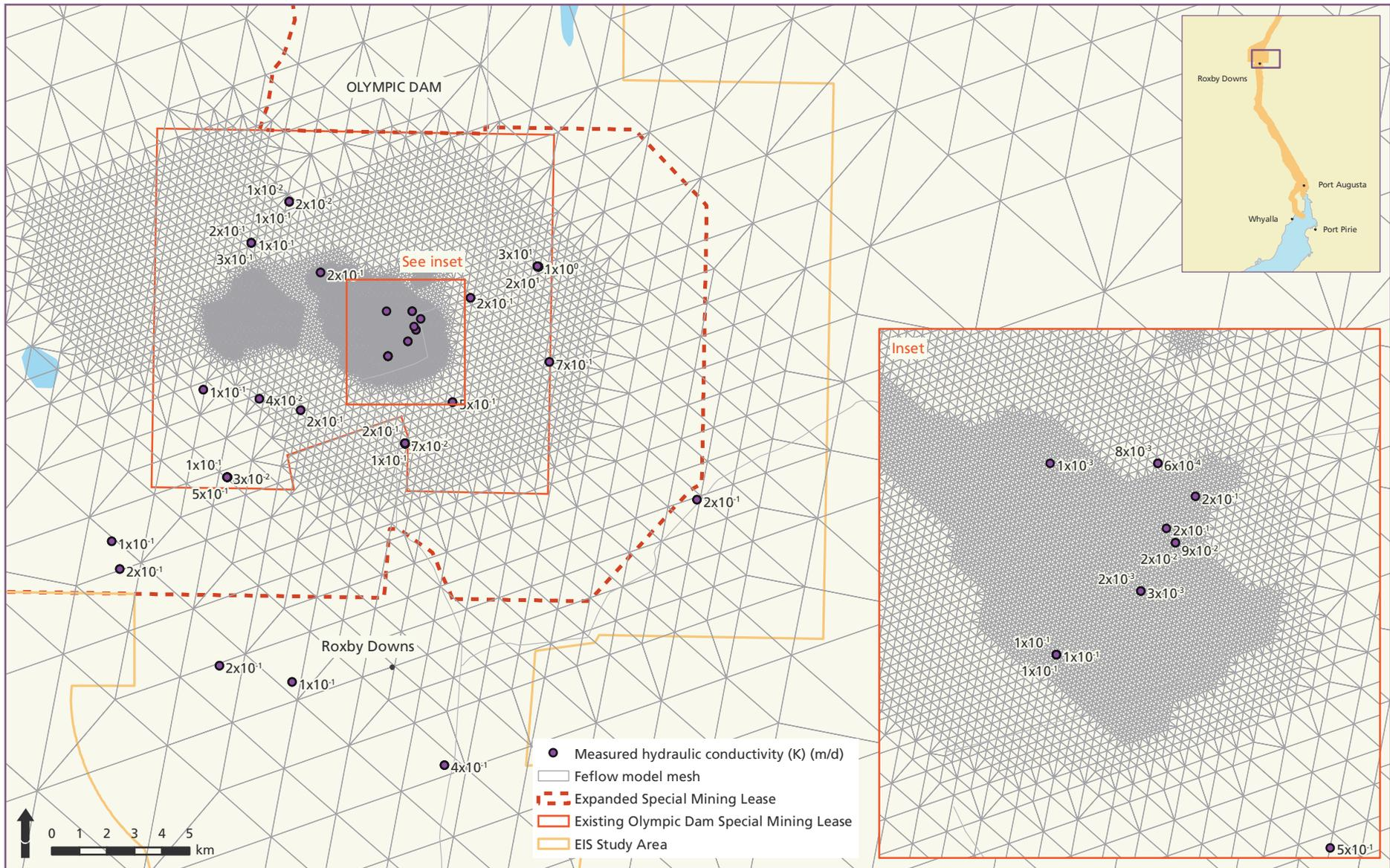
Figure 12.16 Measured hydraulic conductivity in the Corraberra Sandstone (ZWC)
