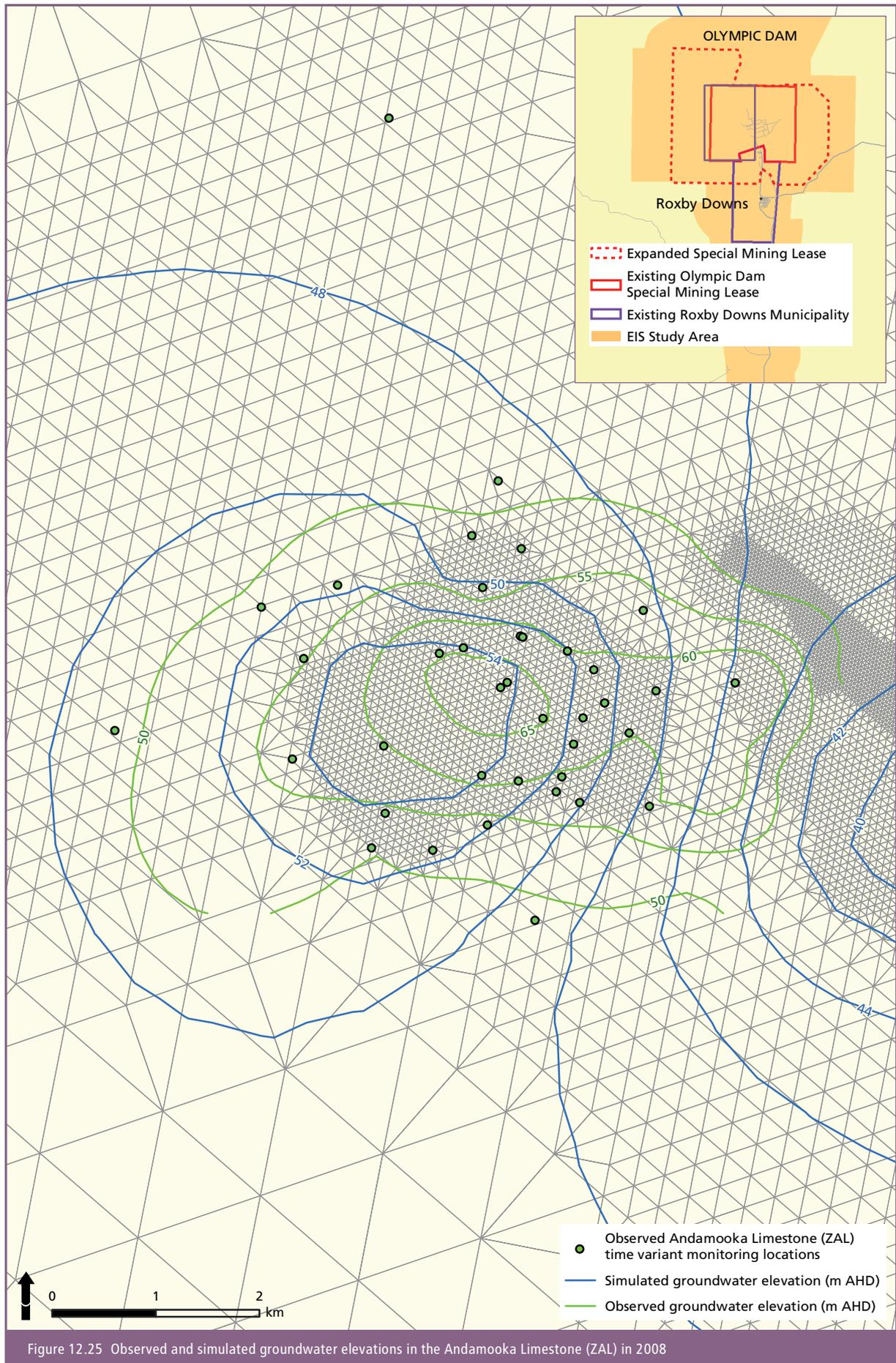
Figure 12.25 Observed and simulated groundwater elevations in the Andamooka Limestone (ZAL) in 2008
