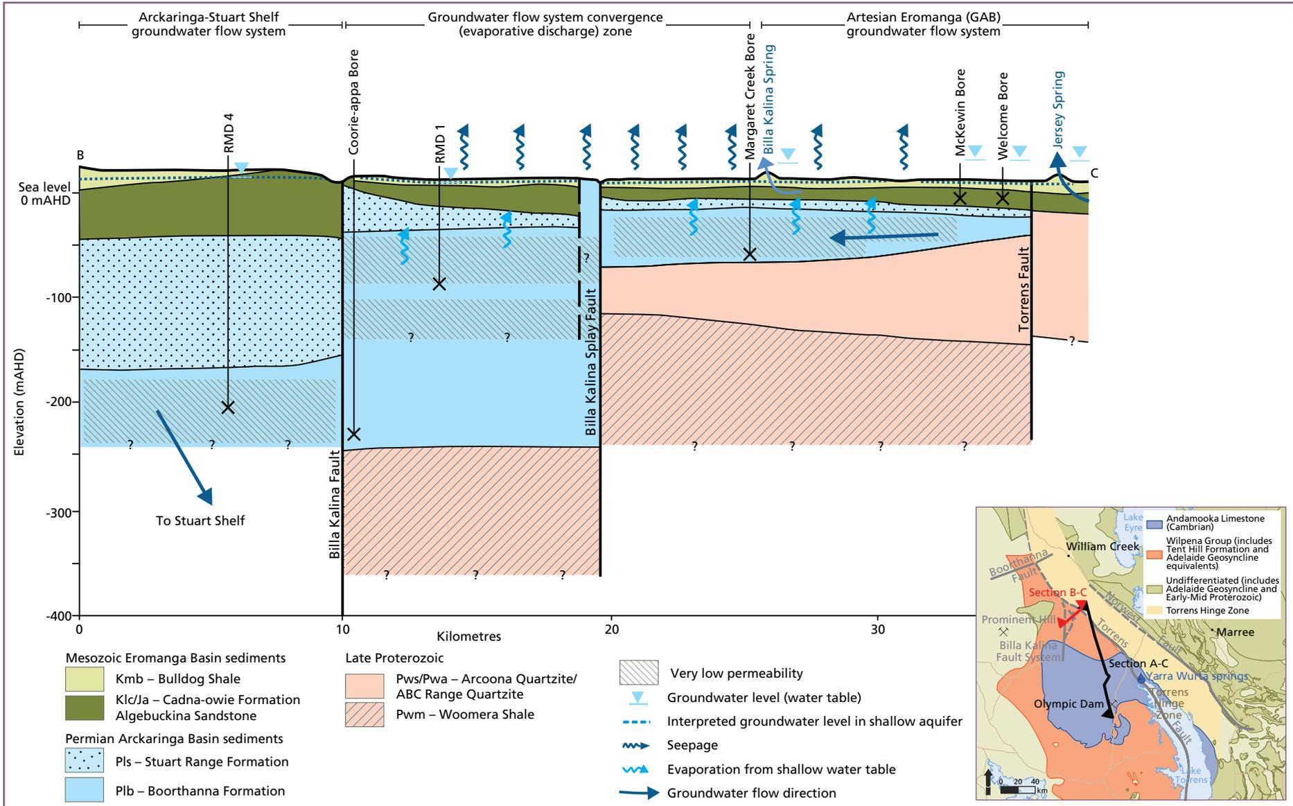
Figure 12.3 Cross-section B-C showing interpreted hydrostratigraphic and structural relationships from the Arckaringa Basin through to the Eromanga Basin
