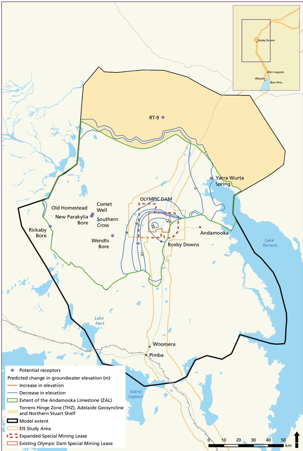
Figure 12.23 Predicted change in Andamooka Limestone (ZAL) groundwater elevation at 2550
