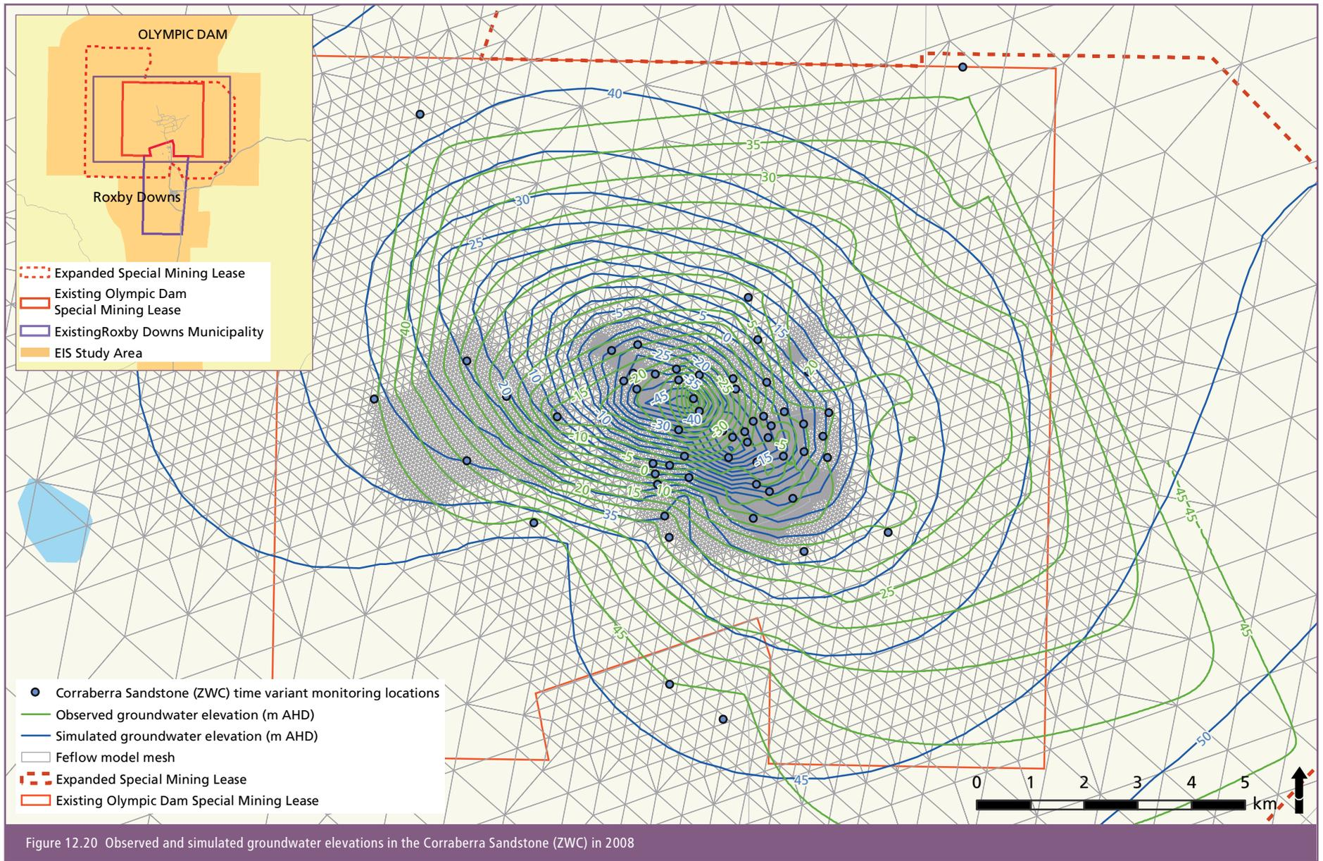
Figure 12.20 Observed and simulated groundwater elevations in the Corraberra Sandstone (ZWC) in 2008
