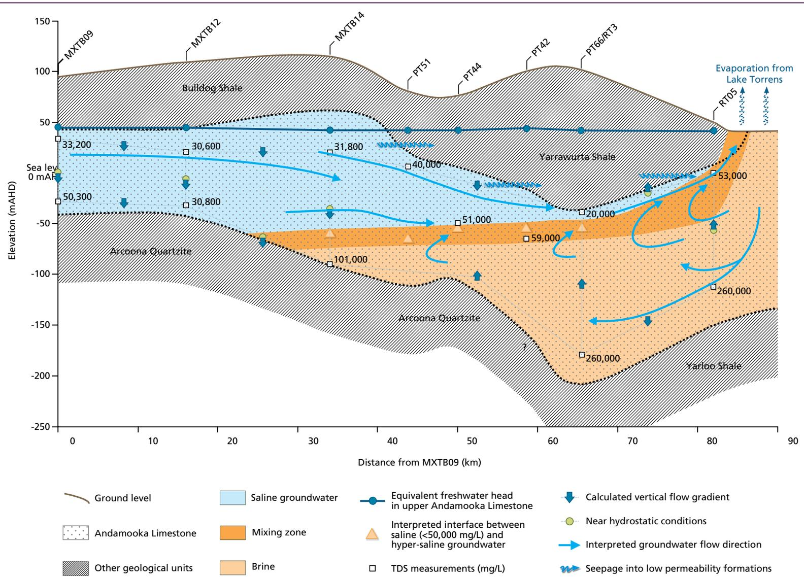
Figure 12.12 Hydrostratigraphic cross-section through the Andamooka Limestone aquifer (ALA) showing the interface between Lake Torrens brine and saline regional groundwaters
