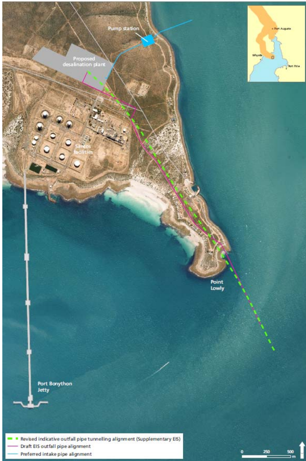
Figure 1: Alignment of the intake and outfall pipelines
