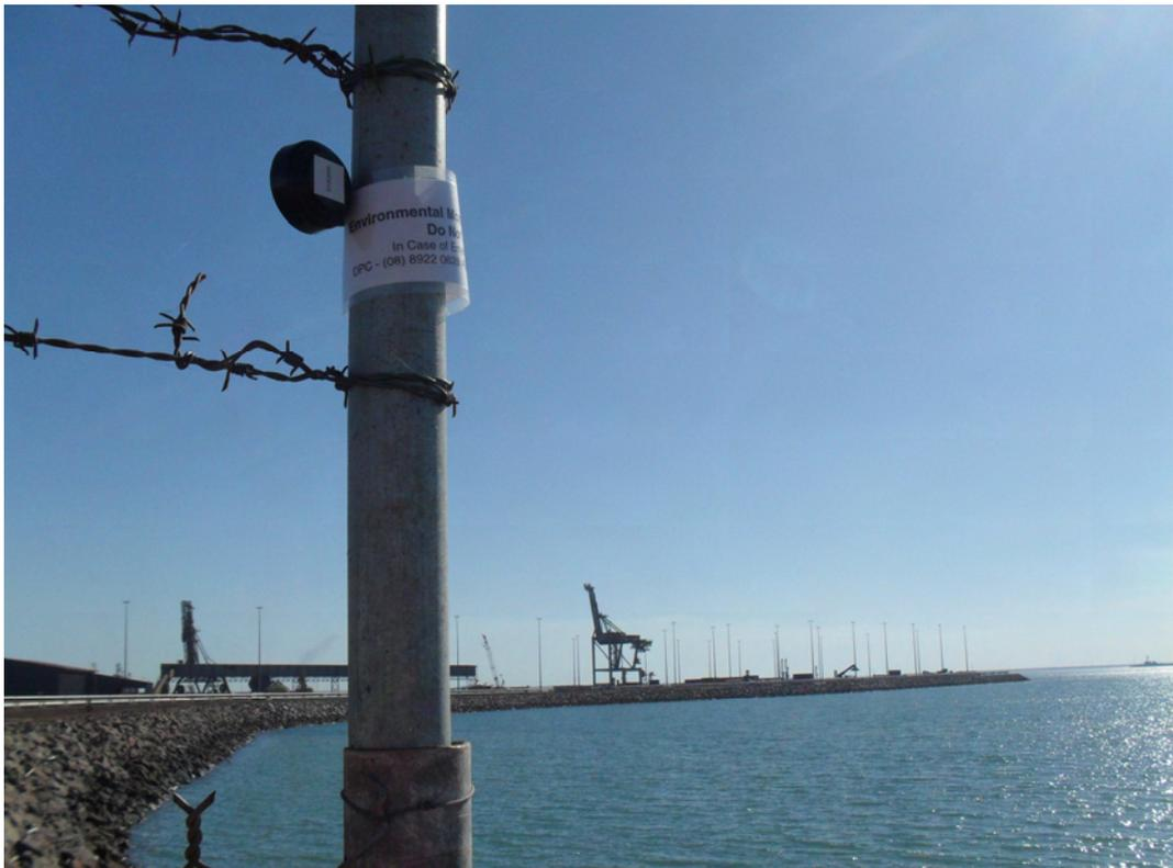
Plate P-2: Track Etch Detector, East Arm Wharf
