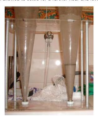
**Figure 2.** Imhoff cone with settleable solids on the right and non-settleable solids on the left.
