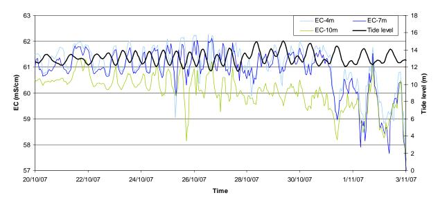
Figure 11 Specific conductance measured at 4m, 7m and 10 m above the seabed and tidal level measured by the Sonde at the Fire Pump site from 20/10/07 to 3/11/07
