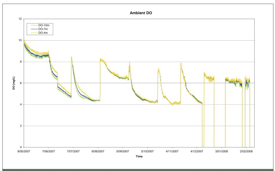
Figure H2.2.6 Dissolved oxygen (DO) measured by the monitoring station (Note instrument drift immeadiately after calibration, resulting in the only reliable data being each peak when the instrument was serviced)
