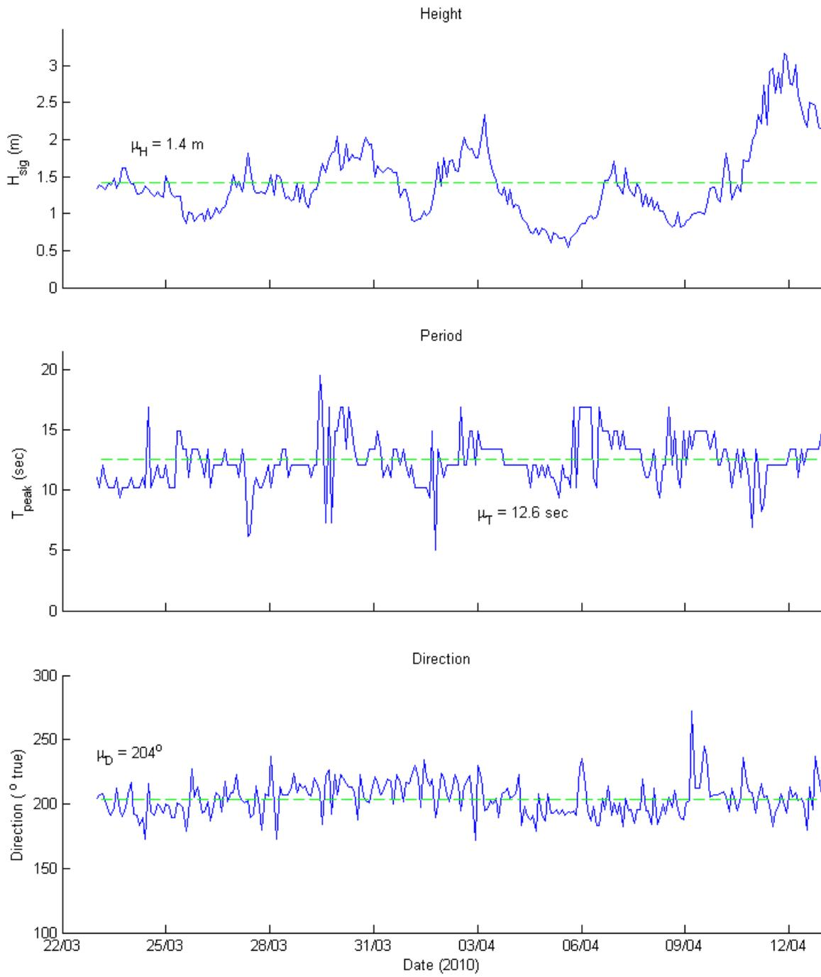
Figure 4-5 ADCP Site 1 Wave Characteristics
