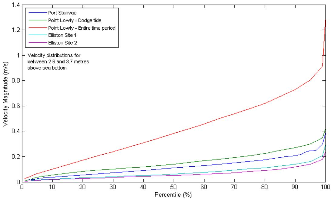
**Figure 4-4 Velocity Magnitude Percentile Comparison with Other Locations at Approximately 2.6 to 3.7 metres from the Seabed at all Locations**
