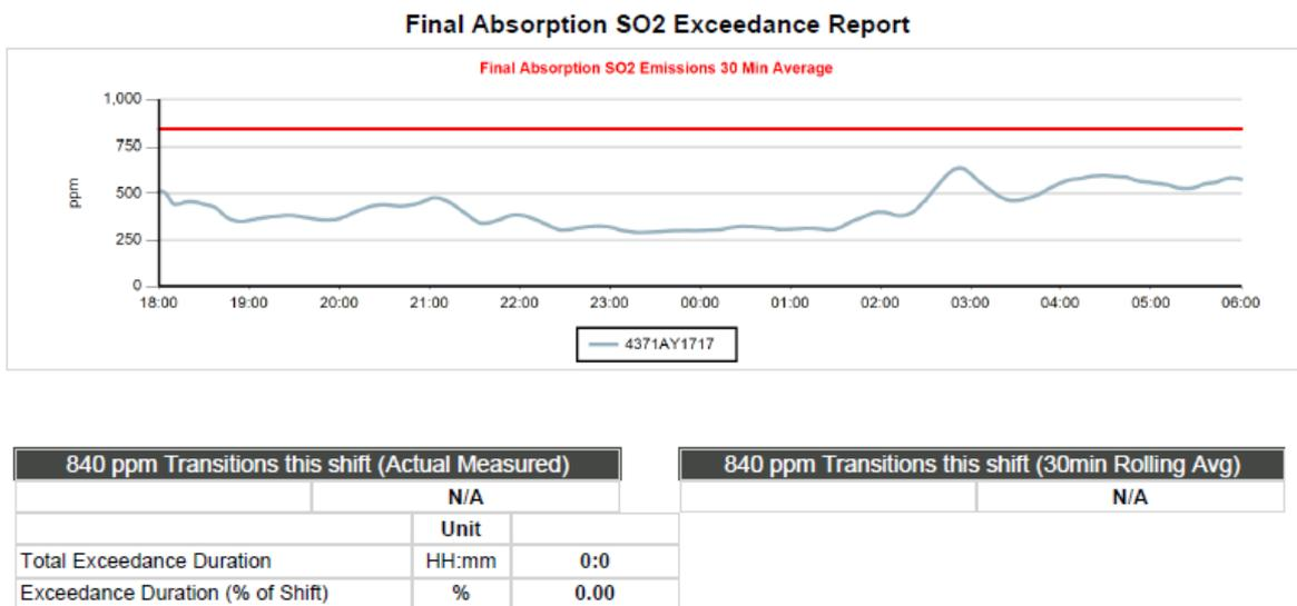
Figure 5.6: Acid Plant Tail Gas Stack SO<sub>2</sub> emission exceedance report
