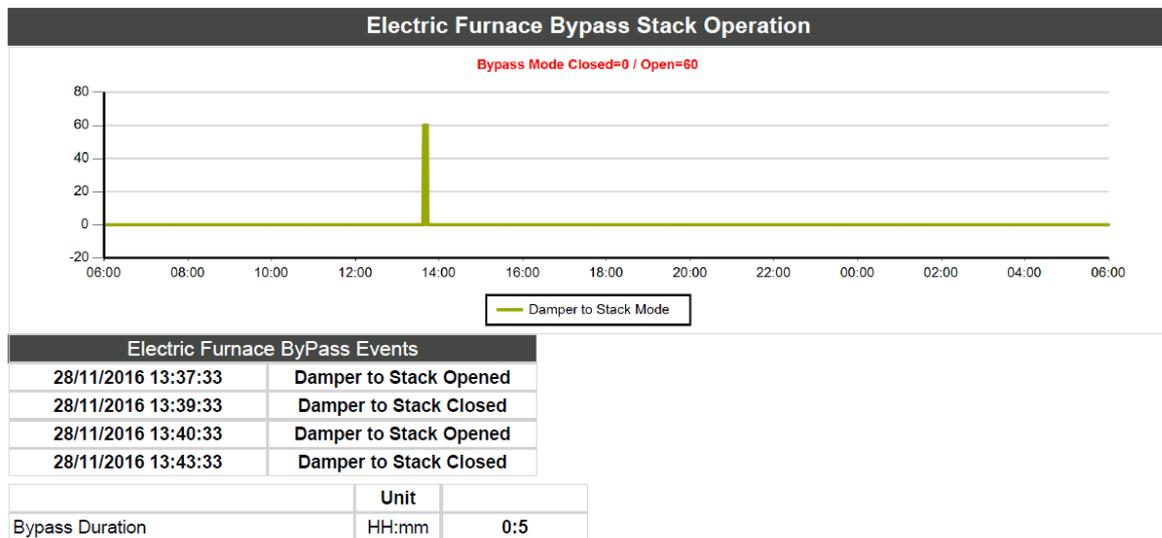
Figure 5.2: Electric Furnace Bypass Stack operation report
