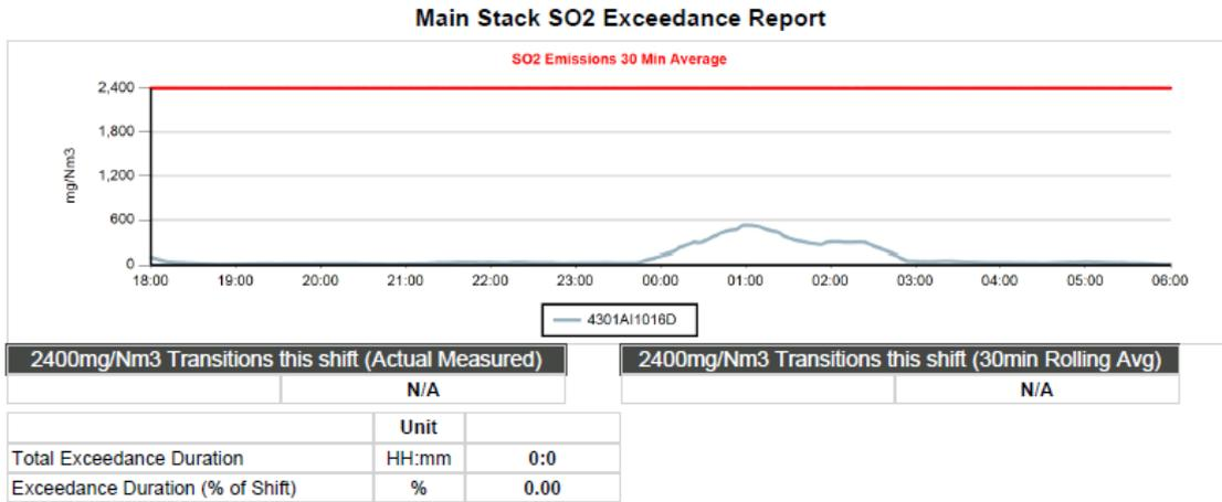
Figure 5.5: Main Smelter Stack SO<sub>2</sub> emission exceedance report
