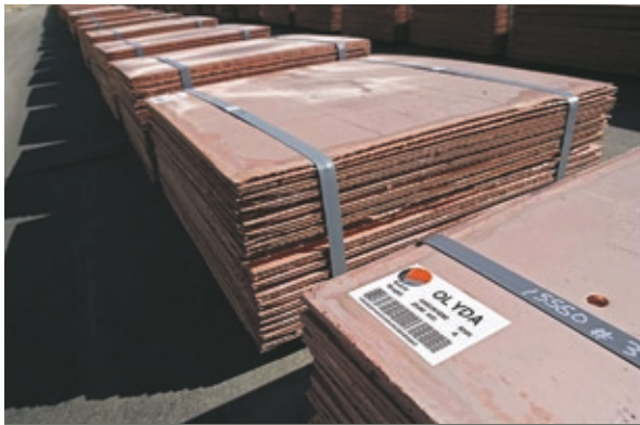
Plate 21.2 Copper cathodes produced at Olympic Dam
