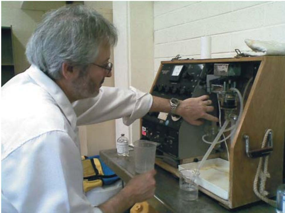
Plate O9.1 Salinity measurement using salinometer
