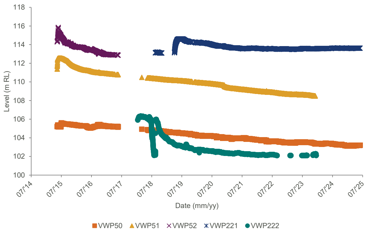
Figure 62: TSF2/3 decant wall VWP (03_C2-3 Decant)
