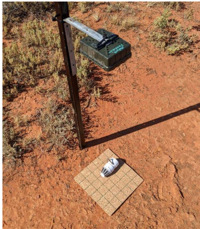
Figure 8. Example setup of remote cameras used to detect plains mouse, with a canister containing bait below.
