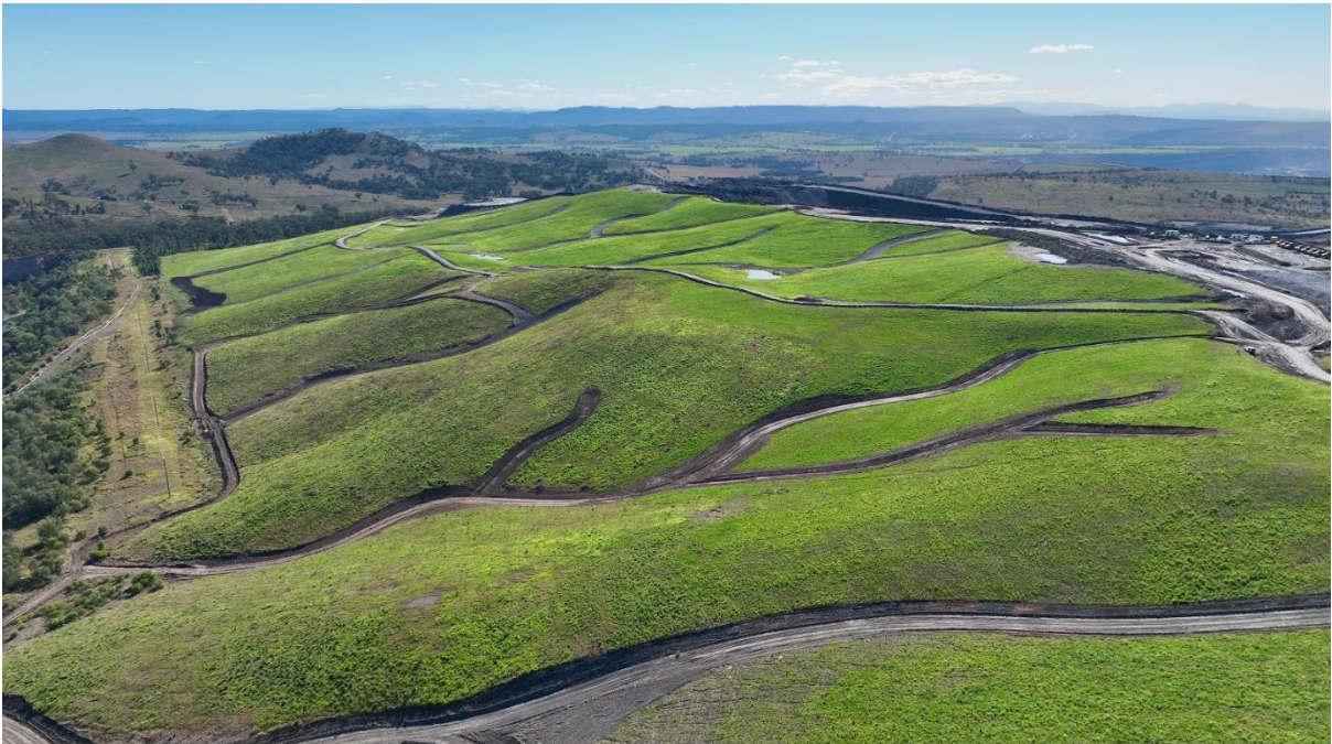
Figure 3: Drain construction in FY23-24 pasture rehabilitation in the OPD emplacement
