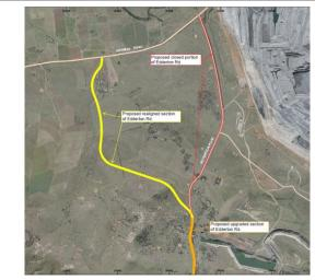
4.3km of new road alignment; Intersection relocation, west from current location to around the Windmill homestead.
