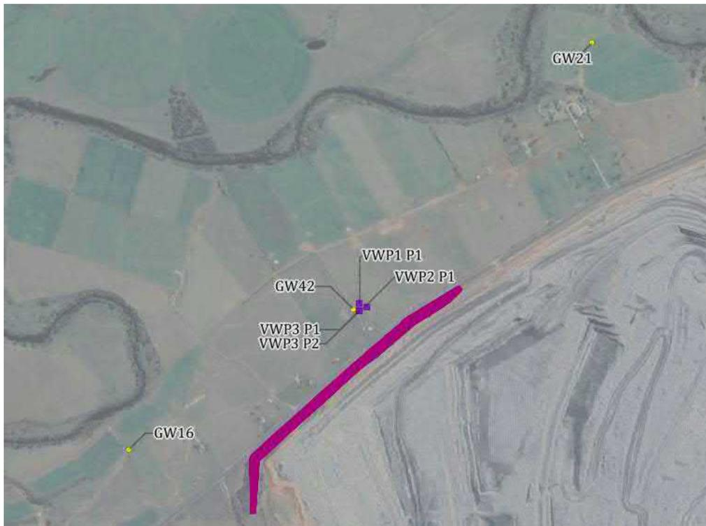
**Figure 3.5 Cut-off wall and HRA monitoring bore locations**
