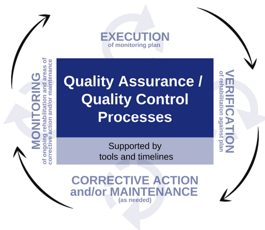
Figure 27: Rehabilitation monitoring quality assurance/quality control process
