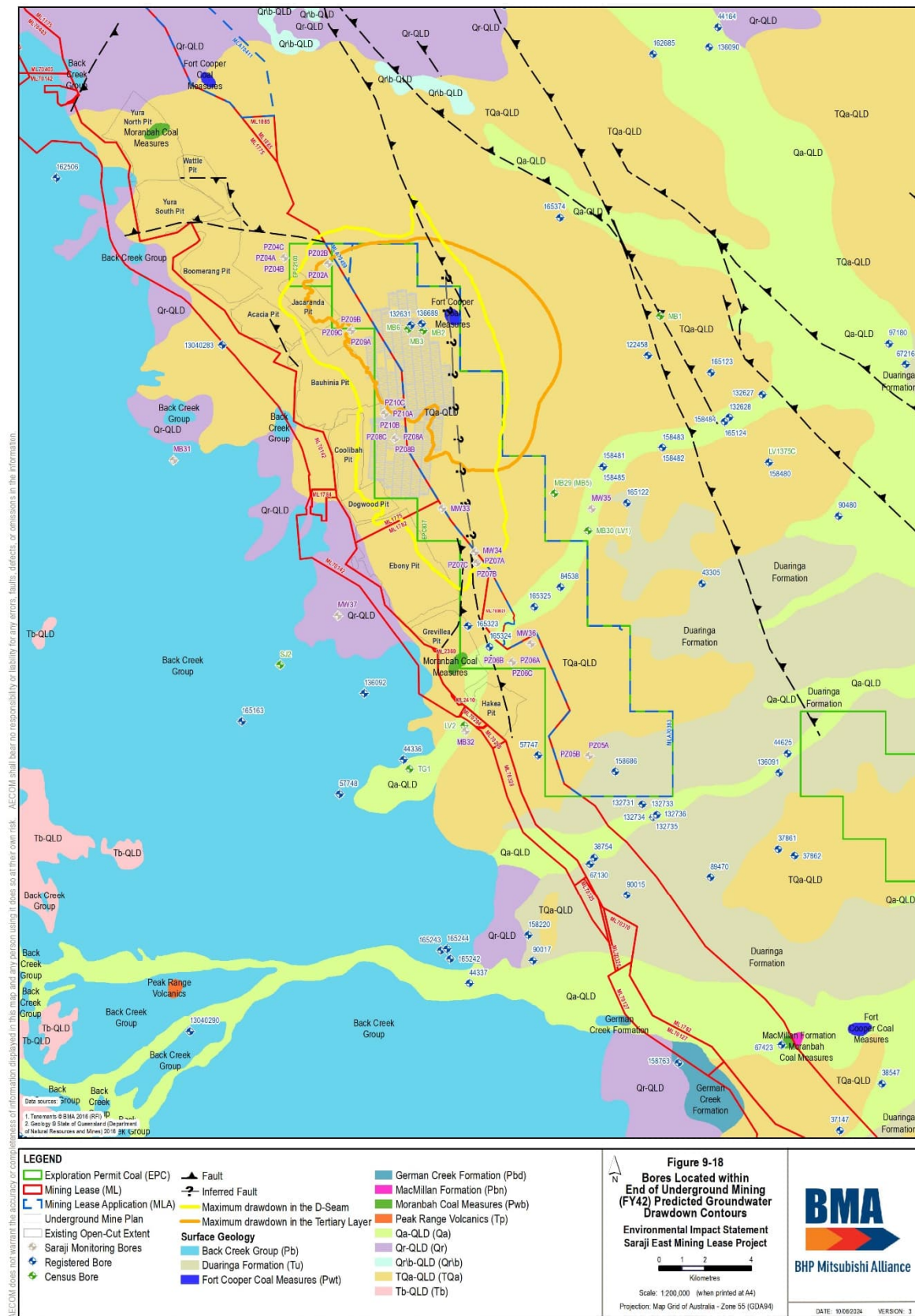
Figure 9-18 Boreholes located within the predicted maximum incremental drawdown in the Tertiary and target D seam
