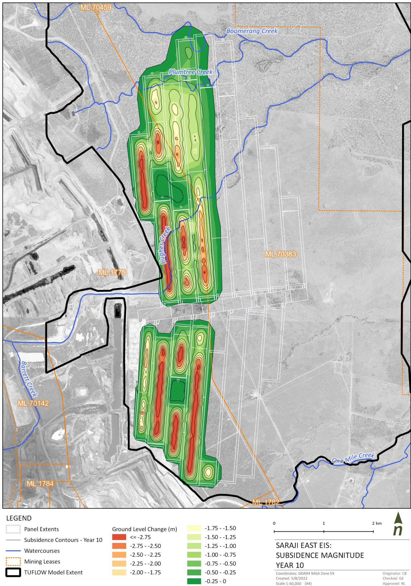
Figure 3-1. Predicted subsidence depths below existing surface (Year 10)
