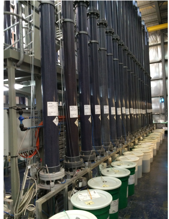
Heap leaching test columns, Olympic Dam
