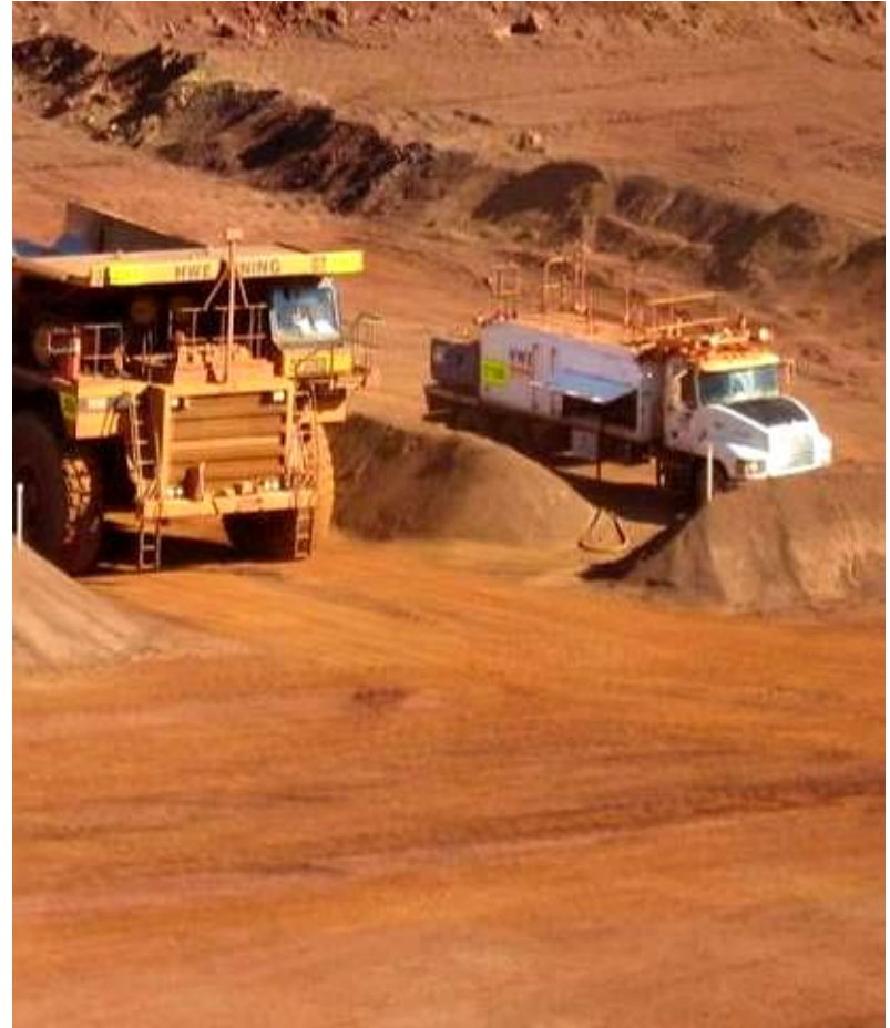
Physical barriers are now in place to separate heavy and light vehicles
