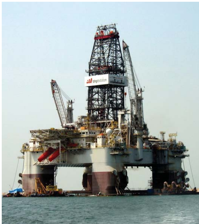
The Development Driller 1, on contract to BHP Billiton through 2007, was specially designed for deepwater development drilling activities. It includes 18,000 square feet of useable deck space and more than 7,000 metric tons of variable deck load.
