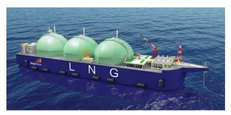
Cabrillo Port's Floating Storage and Re-gasification Unit will be the receiving point for LNG shipments.
