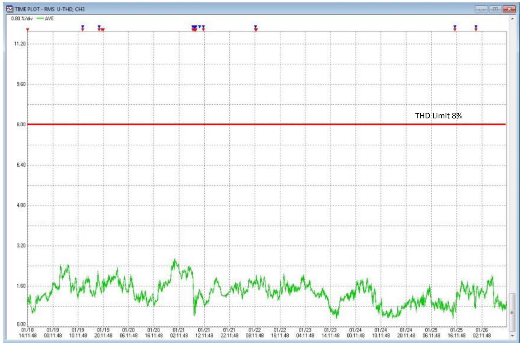
TA Start of Feeder T79 Security Gate 3 rd Phase Vthd
