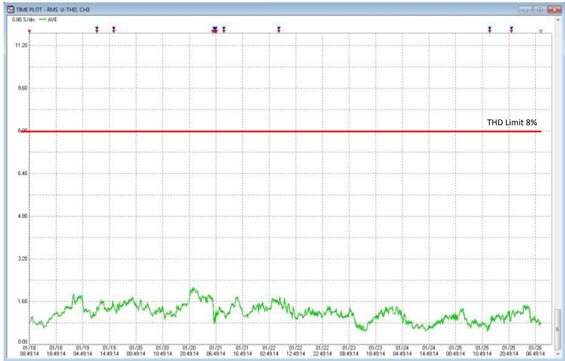
TB Start of Feeder PS60 Forrest Ave 3 rd Phase Vthd
