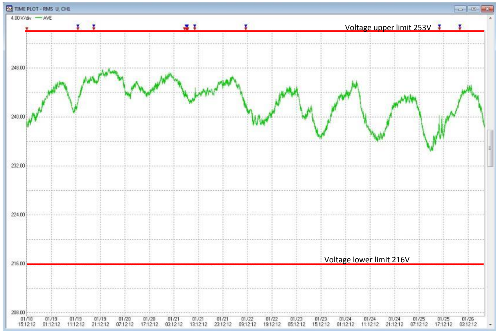
TB End of Feeder PS85 Shovelanna St 1 st Phase Vrms
