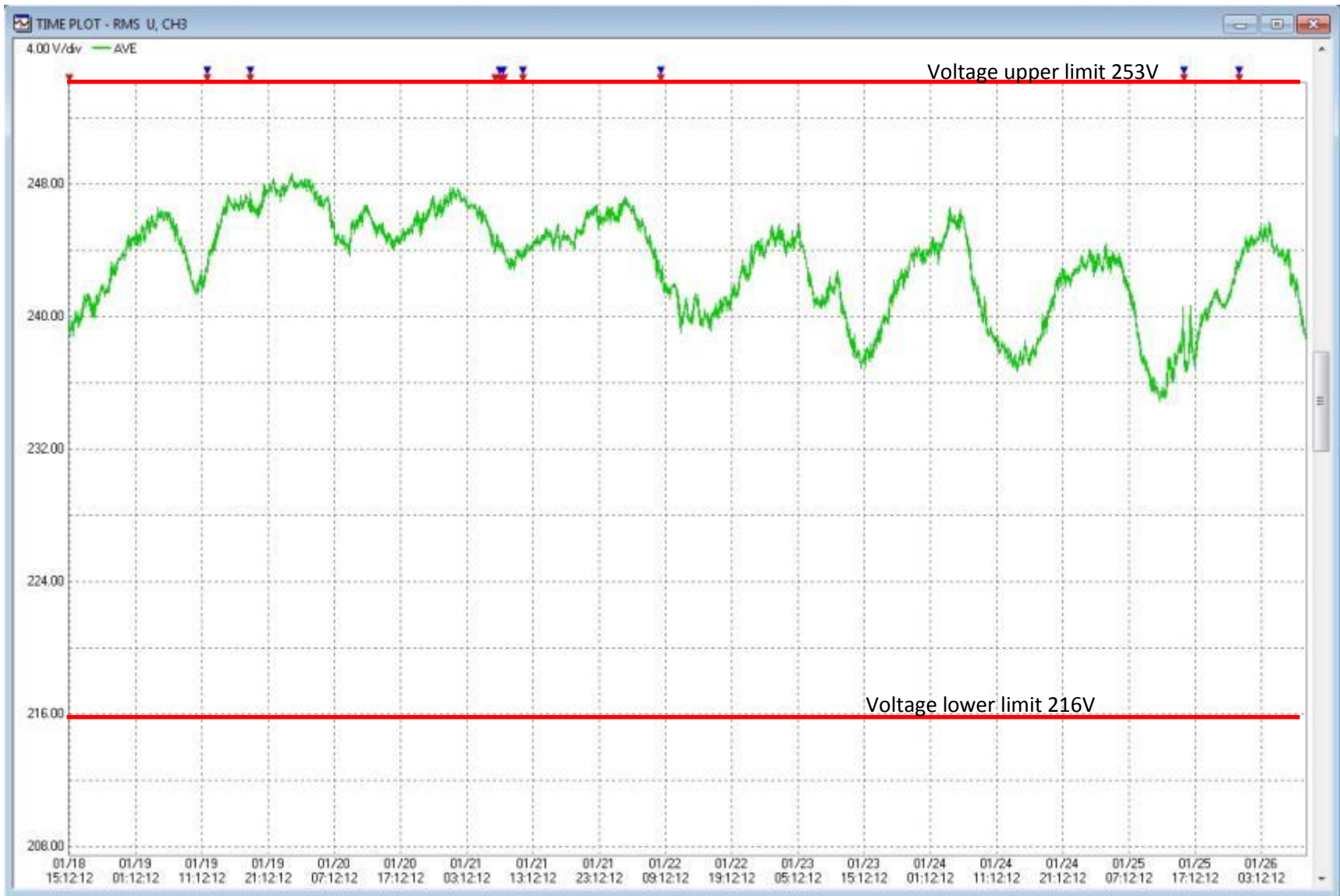
TB End of Feeder PS85 Shovelanna St 3 rd Phase Vrms
