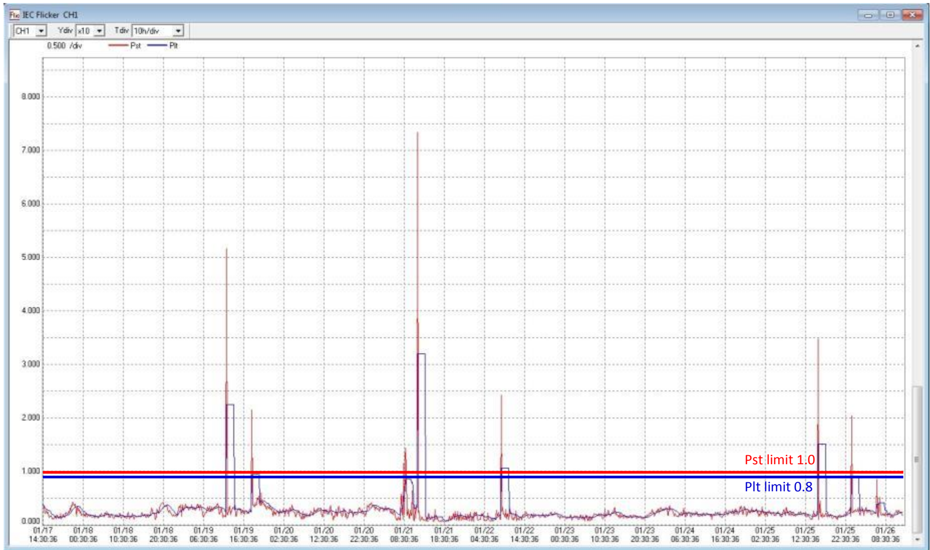
TC3 Start of Feeder T67 Corner of Kurra and Newman Drive 1 st Phase Pst & Plt
