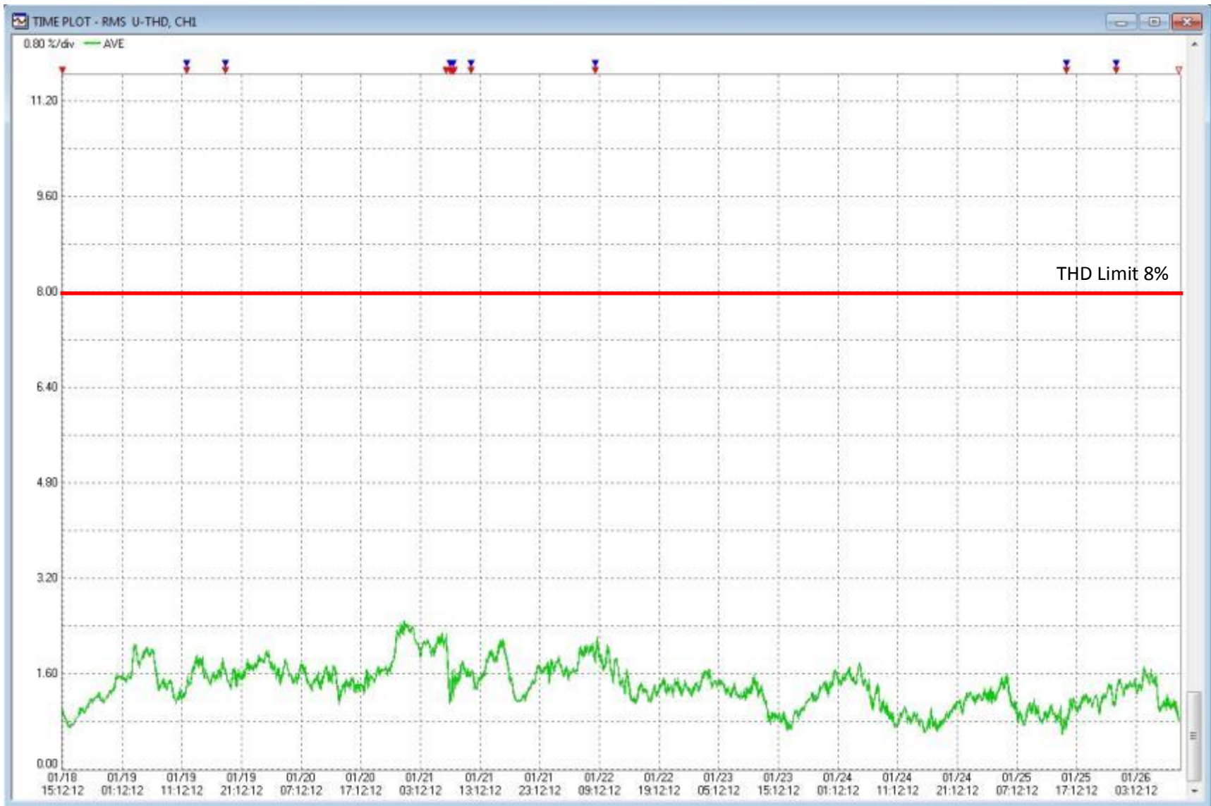
TB End of Feeder PS85 Shovelanna St 1 st Phase Vthd
