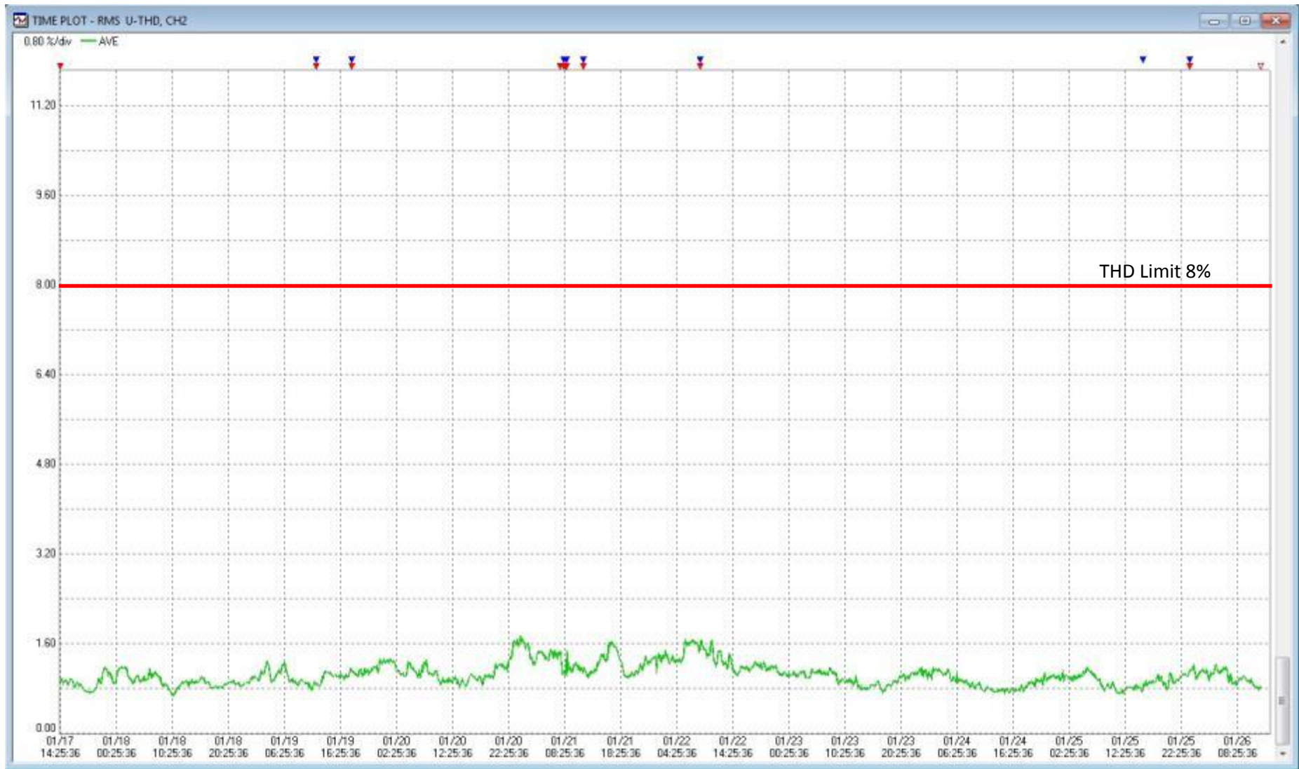
TC3 Start of Feeder T67 Corner of Kurra and Newman Drive 2 nd Phase Vthd
