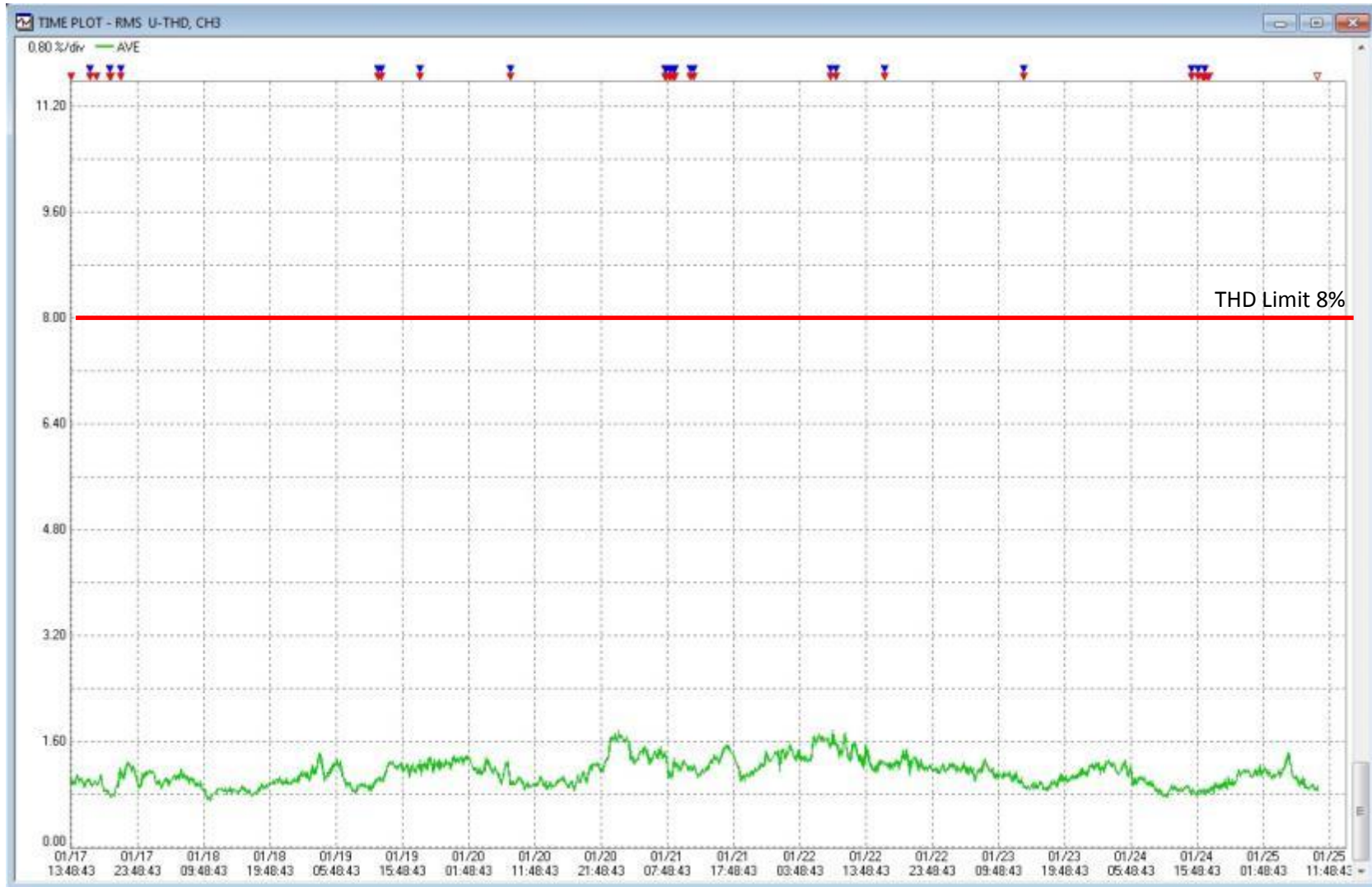
TC4 End of Feeder PS83 Airport 3 rd Phase Vthd
