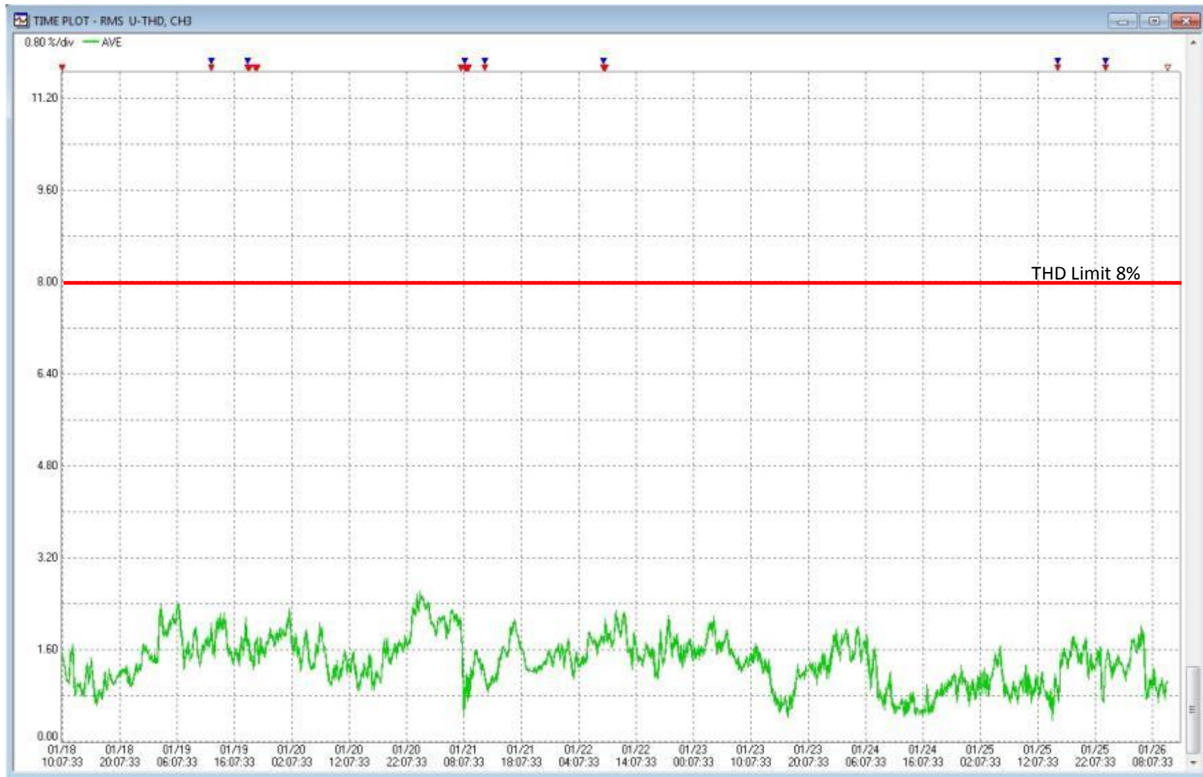
TA End of Feeder T41 Seasons 3 rd Phase Vthd
