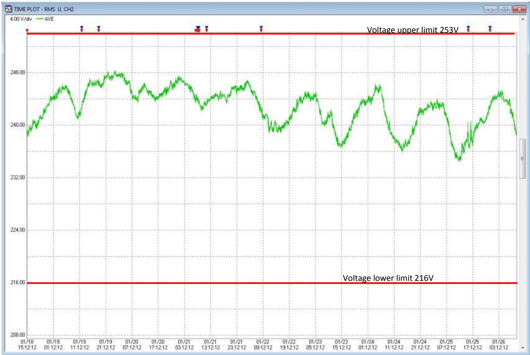
TB End of Feeder PS85 Shovelanna St 2 nd Phase Vrms
