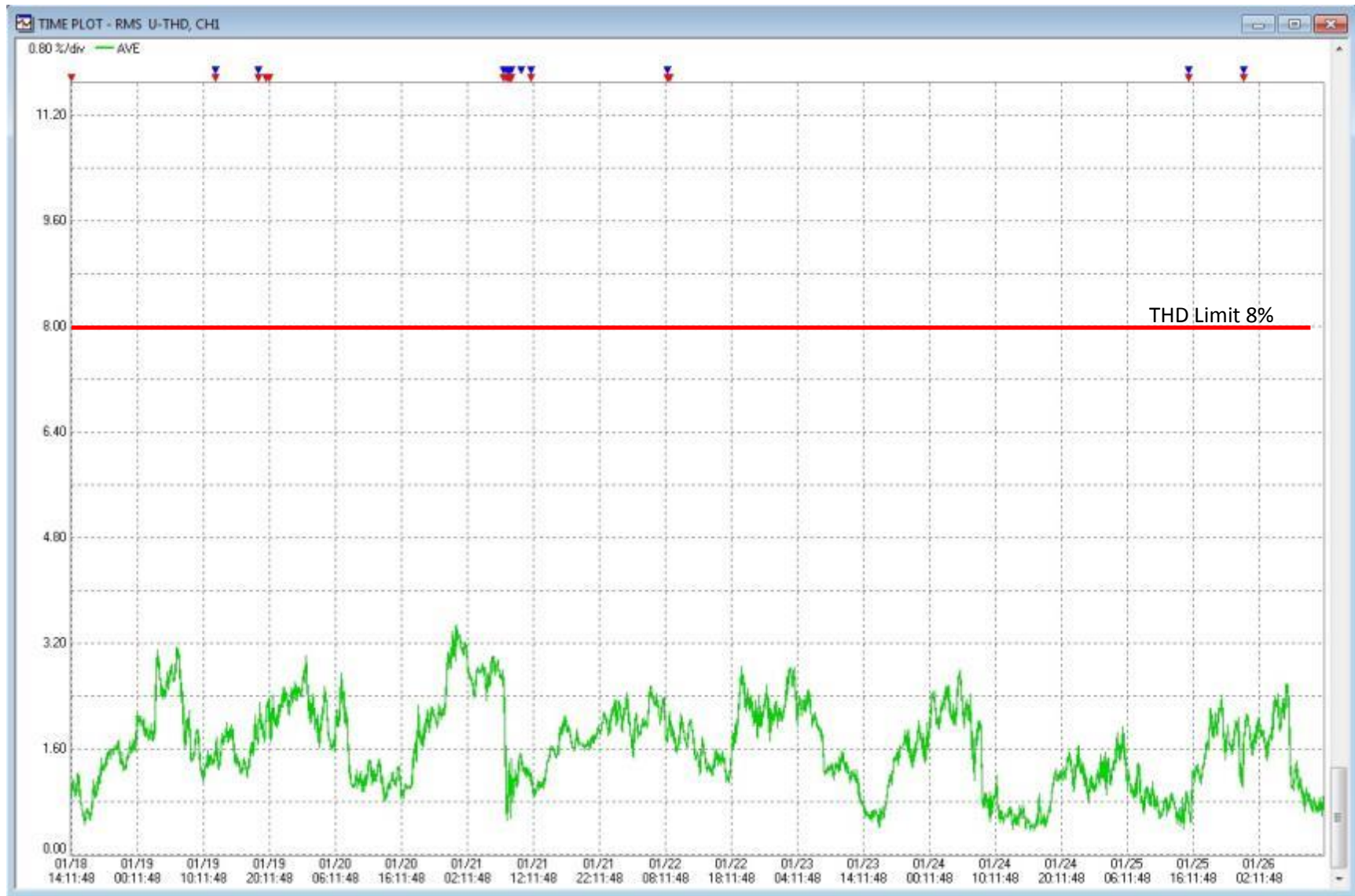
TA Start of Feeder T79 Security Gate 1 st phase Vthd
