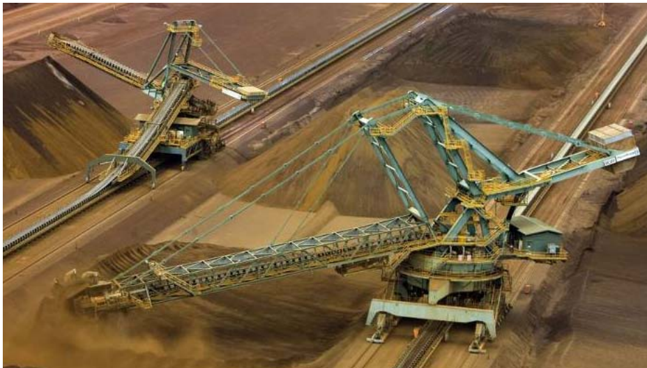
Figure 10-2 Picture of a stacker and reclaimer with their associated conveyor belt system
