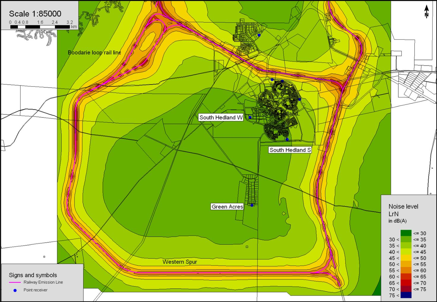
Figure 4-1 Noise Contour plot showing the, Goldsworthy and Western Spur and main lines.
