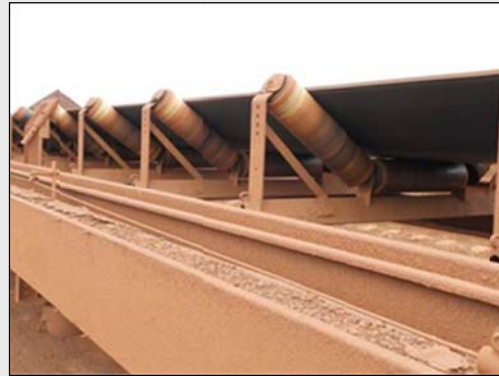
Source: BHP Billiton Iron Ore. Yelloroll idler
