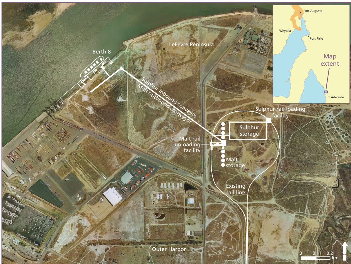
Figure 5.15 Conceptual layout of the proposed Sulphur Handling Facility at Outer Harbor
