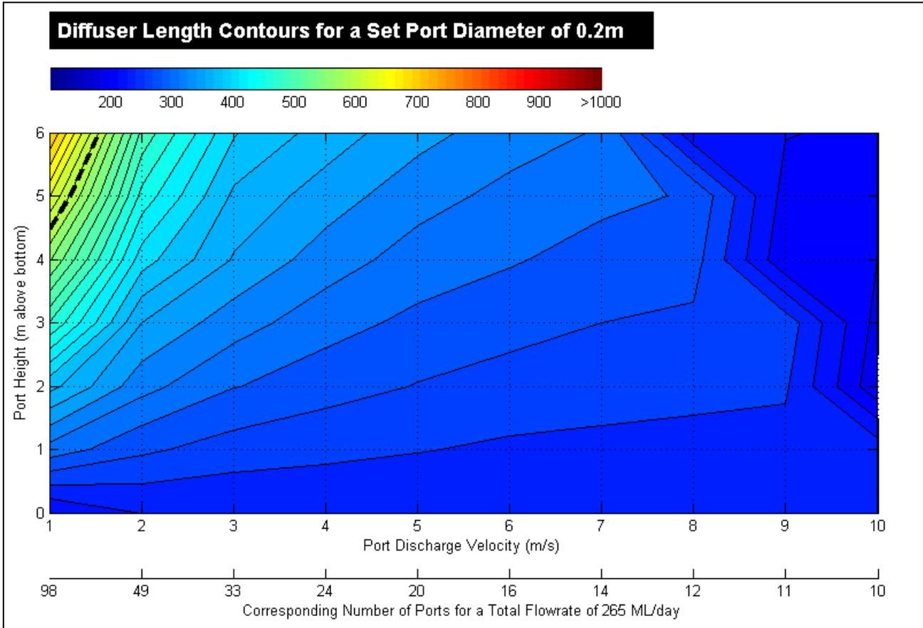
Figure 4-19 Diffuser Length Contours – Port Diameter 0.2m
