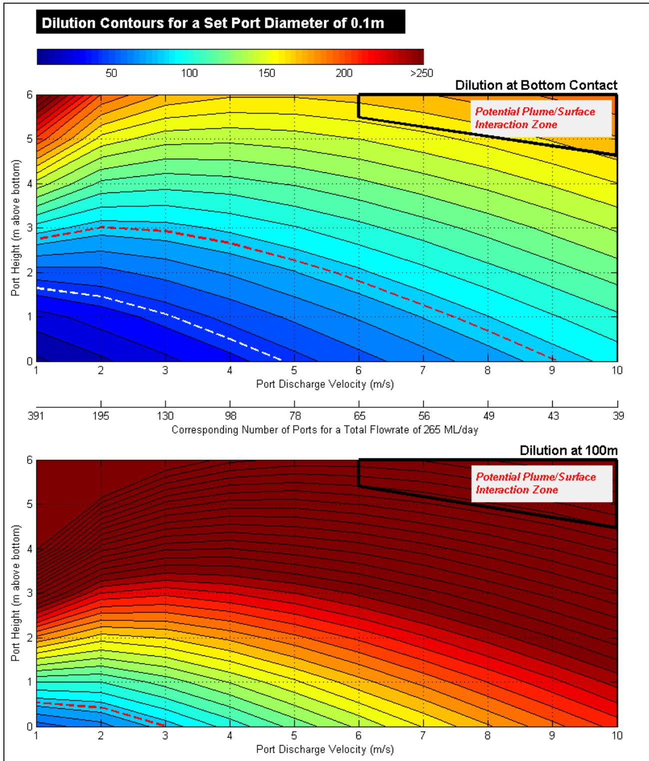
Figure 4-16 Dilution Contours – Port Diameter 0.1m
