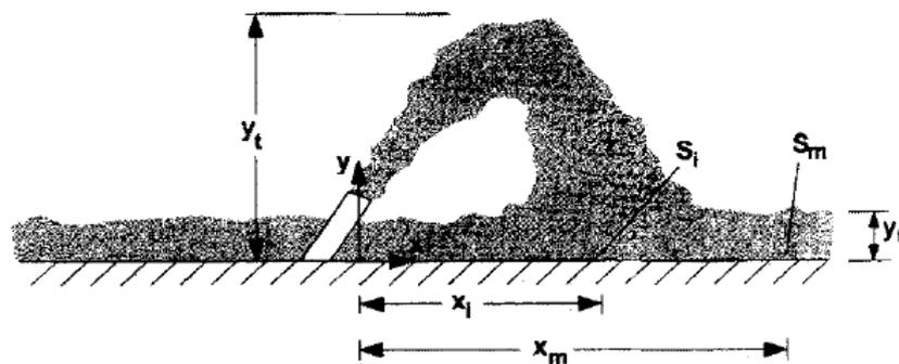
Figure 3-1 Inclined Dense Jet Sketch (reproduced from Roberts *et al.*, 1997)
