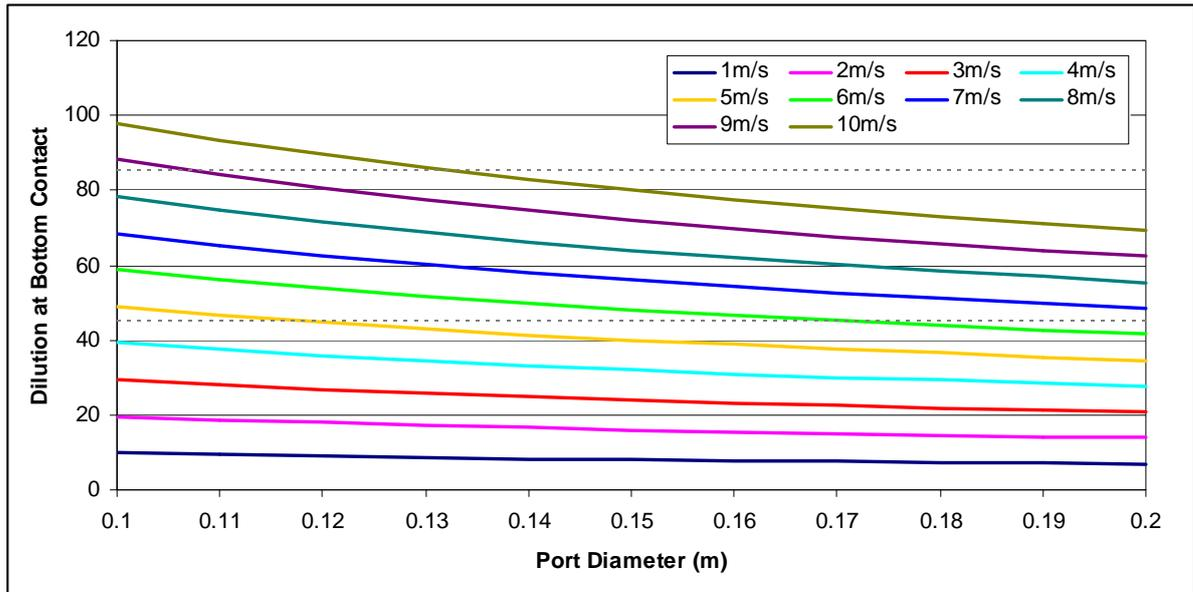
**Figure 4-11 Dilution vs. Port Diameter for a range of Port Exit Discharge Velocities**
