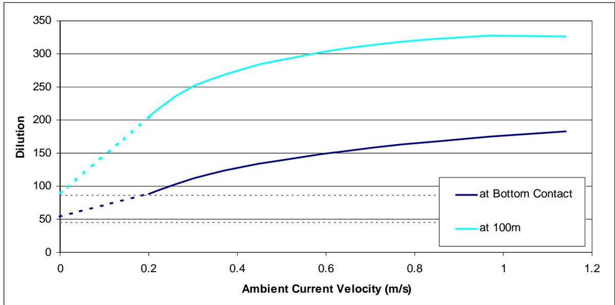
**Figure 4-14 Dilution vs. Ambient Current Velocity for Example 2 Design**
