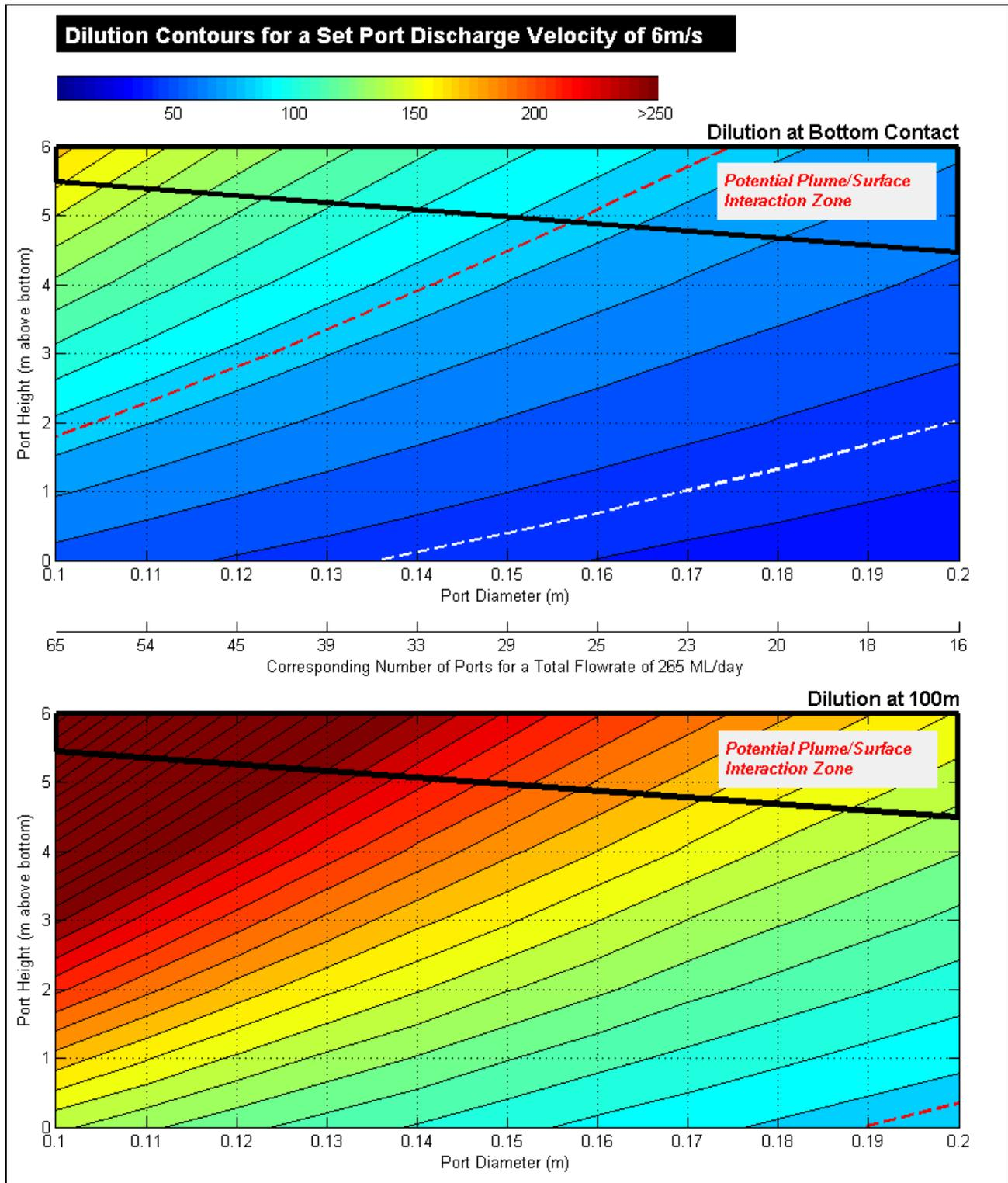
Figure 4-18 Dilution Contours – Port Discharge Velocity 6 m/s
