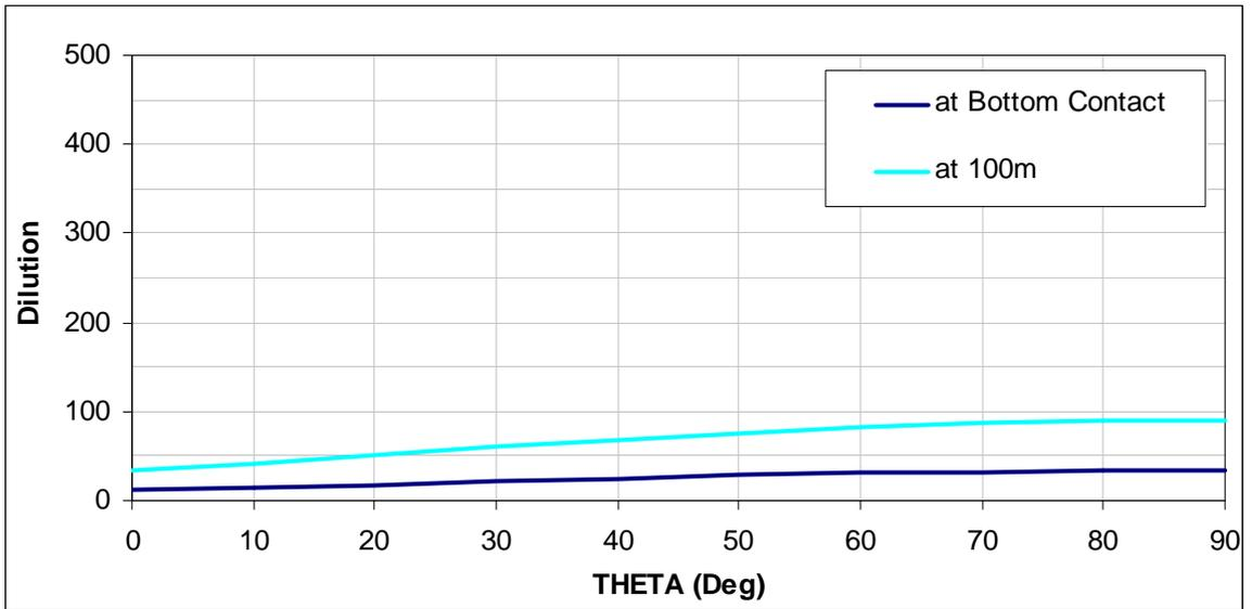
Figure 4-8 Dilution vs. Angle to Horizontal Plane
