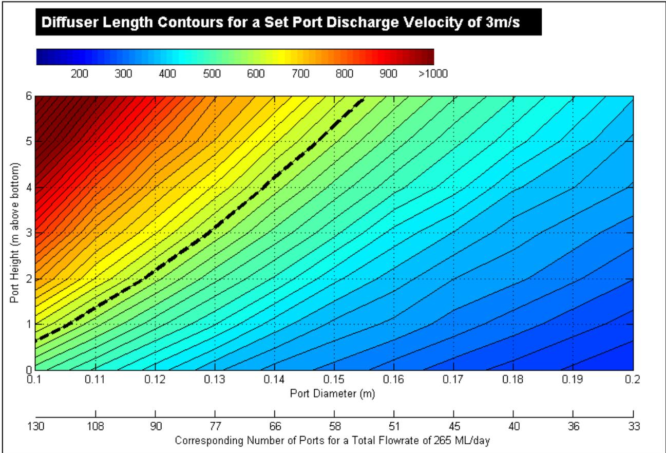
Figure 4-21 Diffuser Length Contours – Port Discharge Velocity 3 m/s
