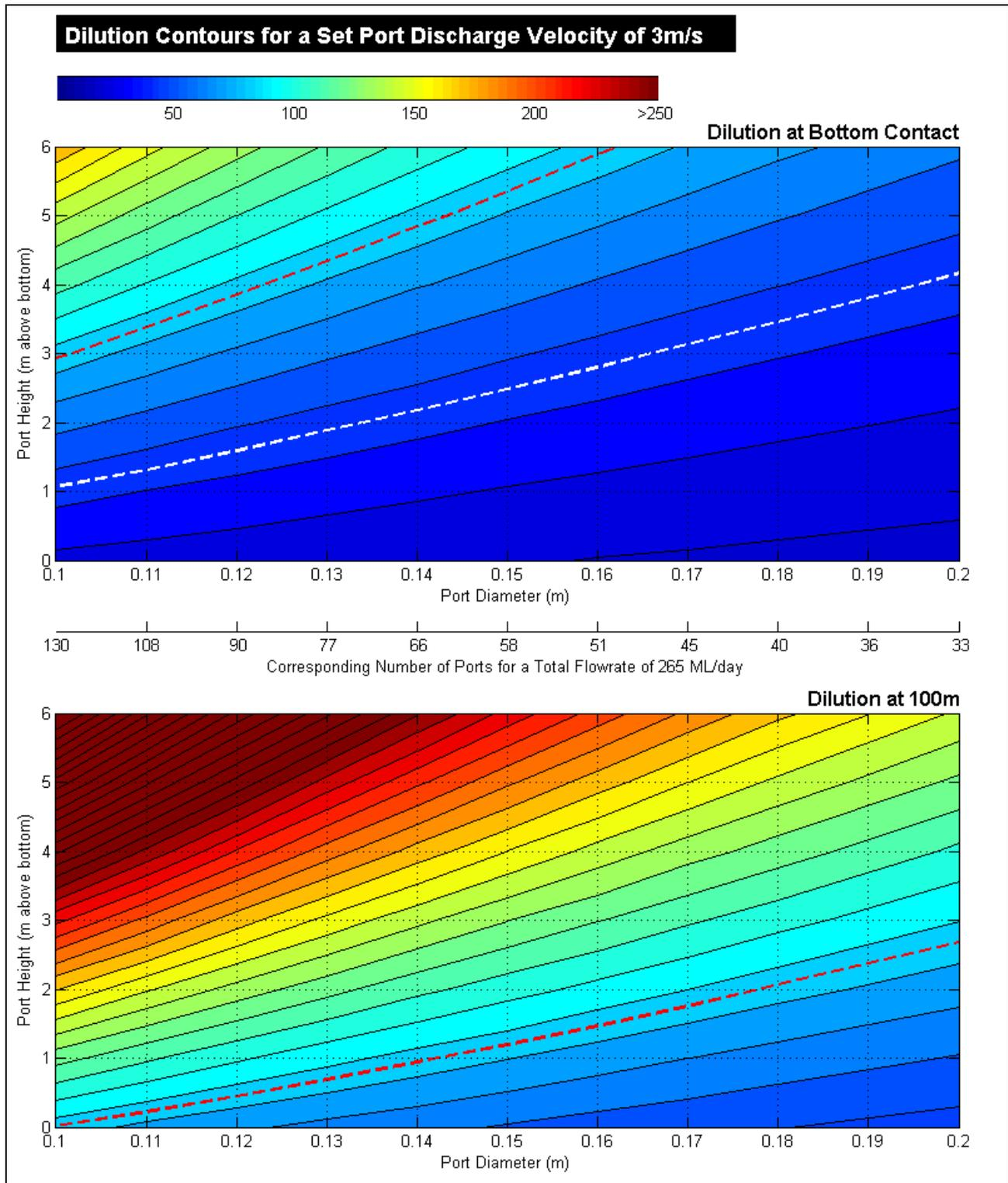
Figure 4-17 Dilution Contours – Port Discharge Velocity 3 m/s
