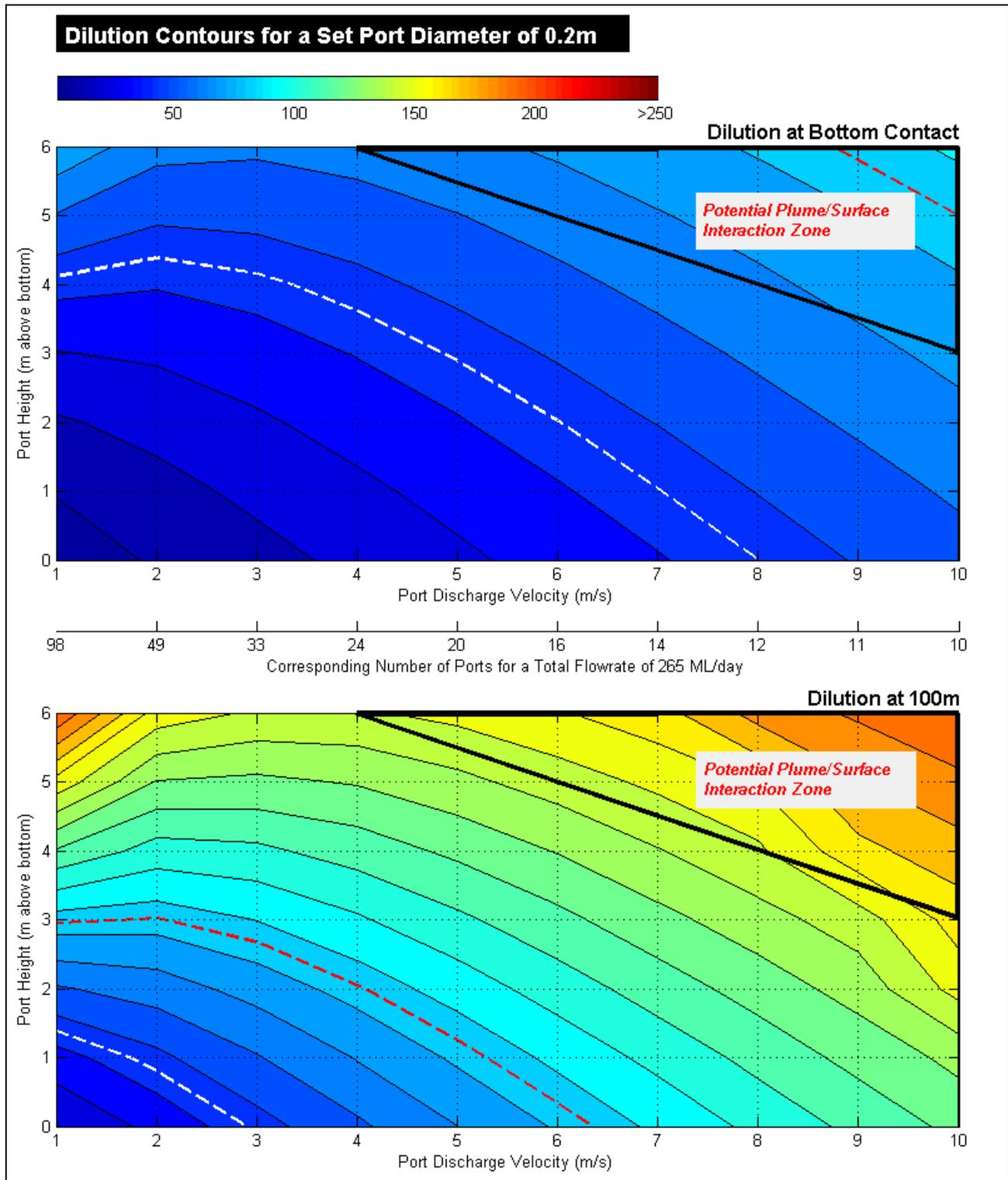
Figure 4-15 Dilution Contours – Port Diameter 0.2m
