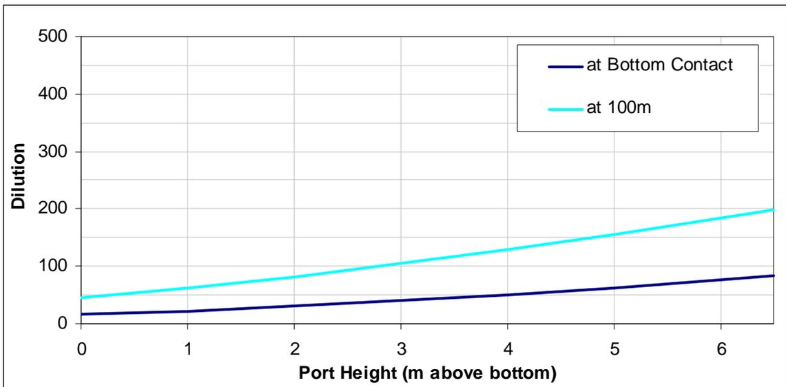
Figure 4-6 Dilution vs. Port Height above Seabed
