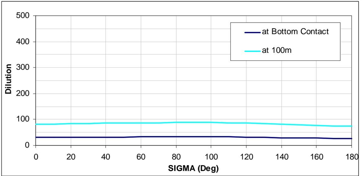
Figure 4-7 Dilution vs. Angle to Ambient Current
