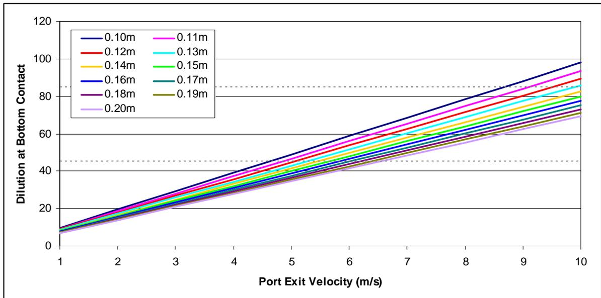
**Figure 4-10 Dilution vs. Port Exit Discharge Velocity for a range of Port Diameters**
