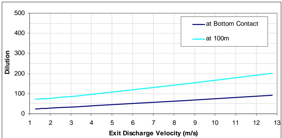
**Figure 4-9 Dilution vs. Port Exit Discharge Velocity**
