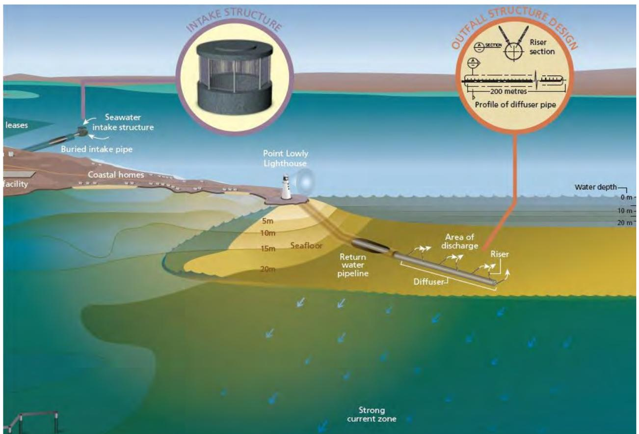
Figure 2-1 Draft EIS Diffuser Design
