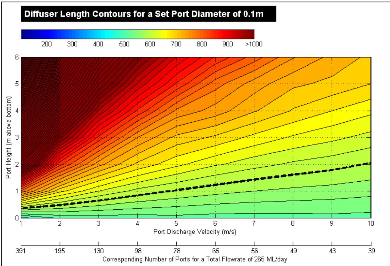
Figure 4-20 Diffuser Length Contours – Port Diameter 0.1m
