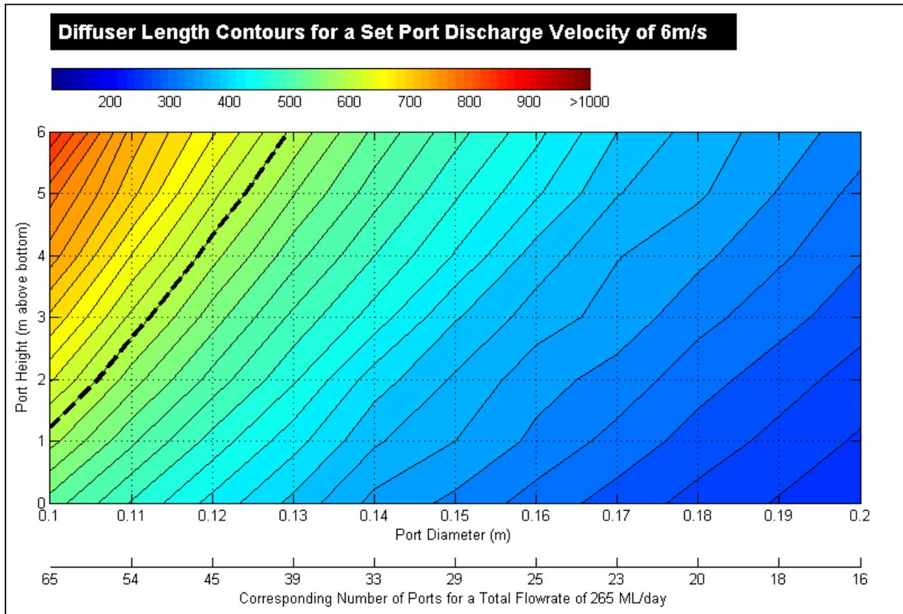
Figure 4-22 Diffuser Length Contours – Port Discharge Velocity 6 m/s
