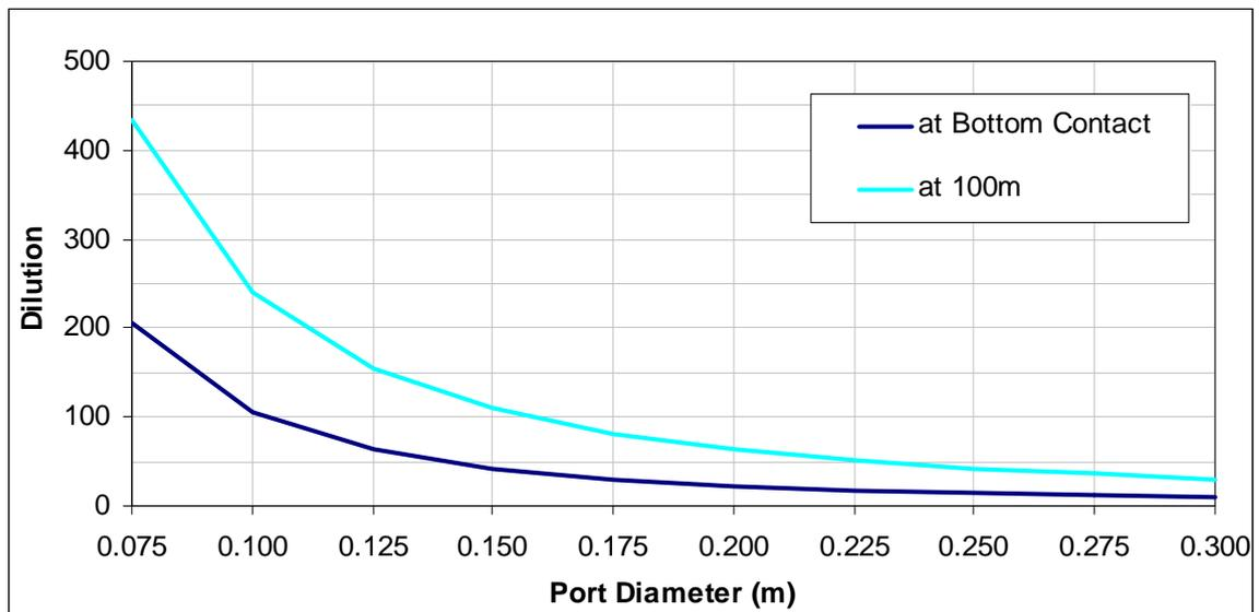
Figure 4-4 Dilution vs. Port Diameter
