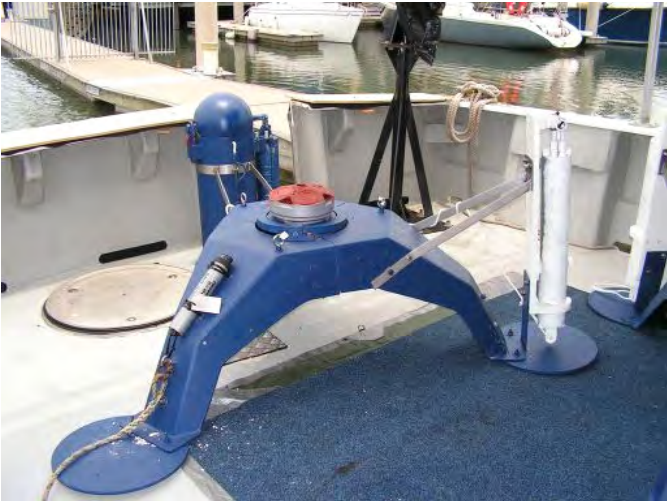
Figure 2-2 Typical instrument arrangement in the “spider” frame. ADCP housed in the centre and additional probe and retrieval systems attached to the frame as required.
