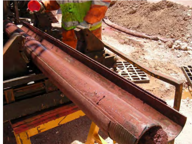
Tailings in a liner immediately after splitting the rod
