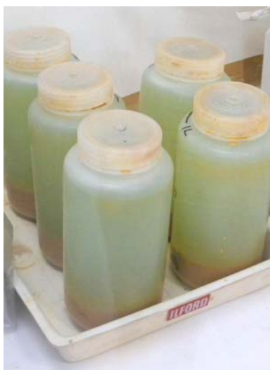
Figure 2. Partial neutralisation of tailings liquor using calcite
