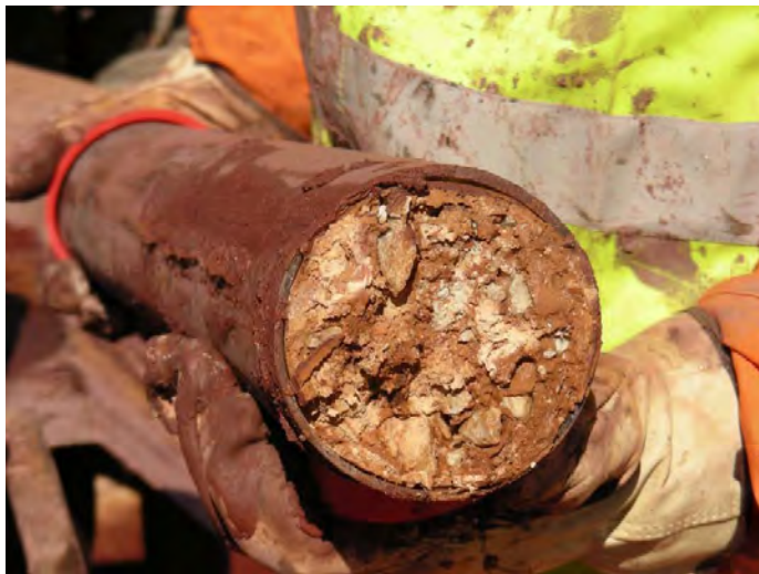
Uncapped liner at contact with ground
