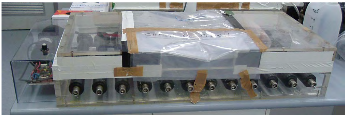
Figure 3. Rolling of materials in a nitrogen atmosphere for leach and adsorption tests
