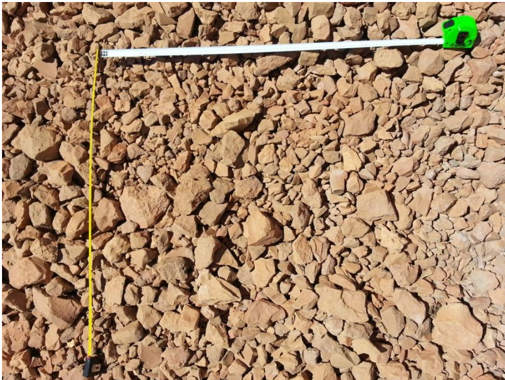
Figure 2: Cell 1 lower slope batter section with D_{50} of 13.7mm.
