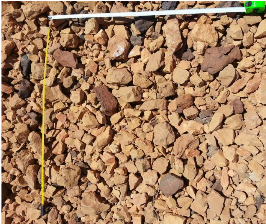
Figure 4: Cell 2 upper slope batter section with D_{50} of 43.3mm.
