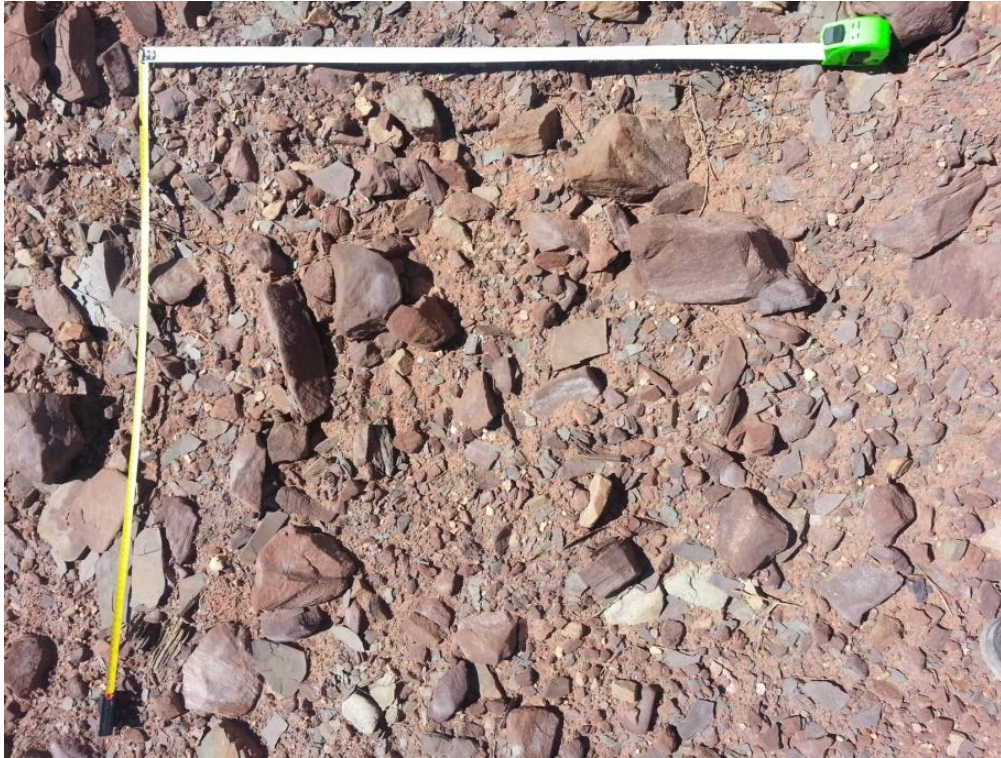
Figure 2: Cell 1 lower slope batter section with D_{50} of 13.7mm.
