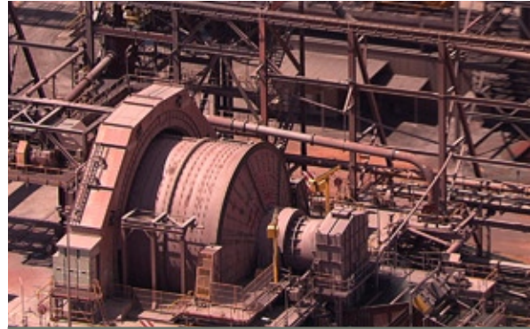
Plate 2.6 A primary semi-autogenous grinding mill
