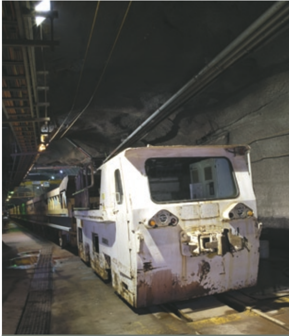
Plate 2.4 Underground electric ore train
