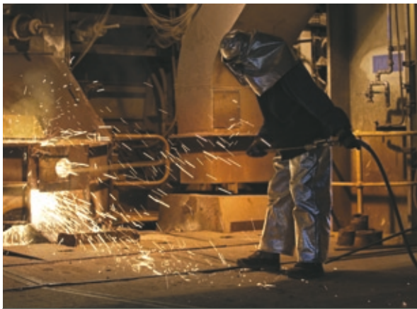
Plate 2.9 Blister copper tapping in the smelter
