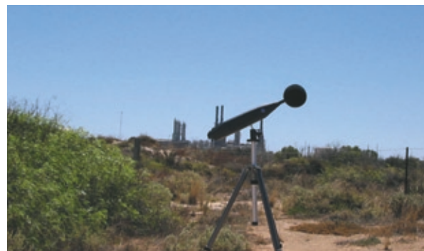
Plate 14.1 Attended noise measurement at Olympic Dam Village
