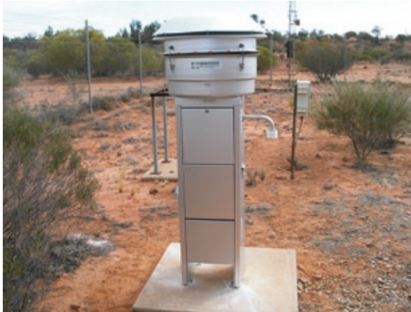
Plate 13.8 PM 10 high volume air sampler at Roxby Downs
