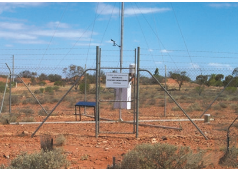
Plate 13.2 Site Automatic Weather Station (AWS)
