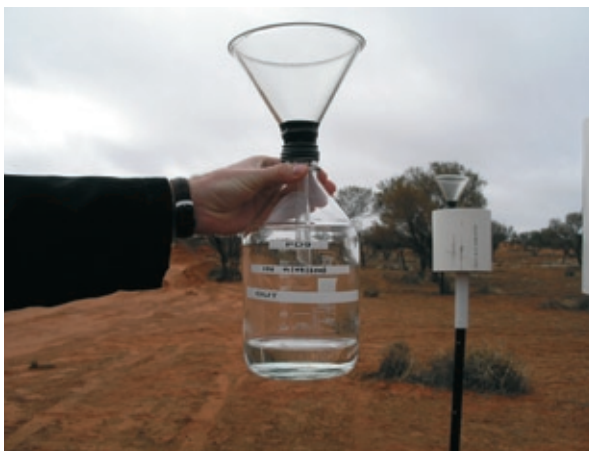
Plate 13.9 Dust deposition gauge
