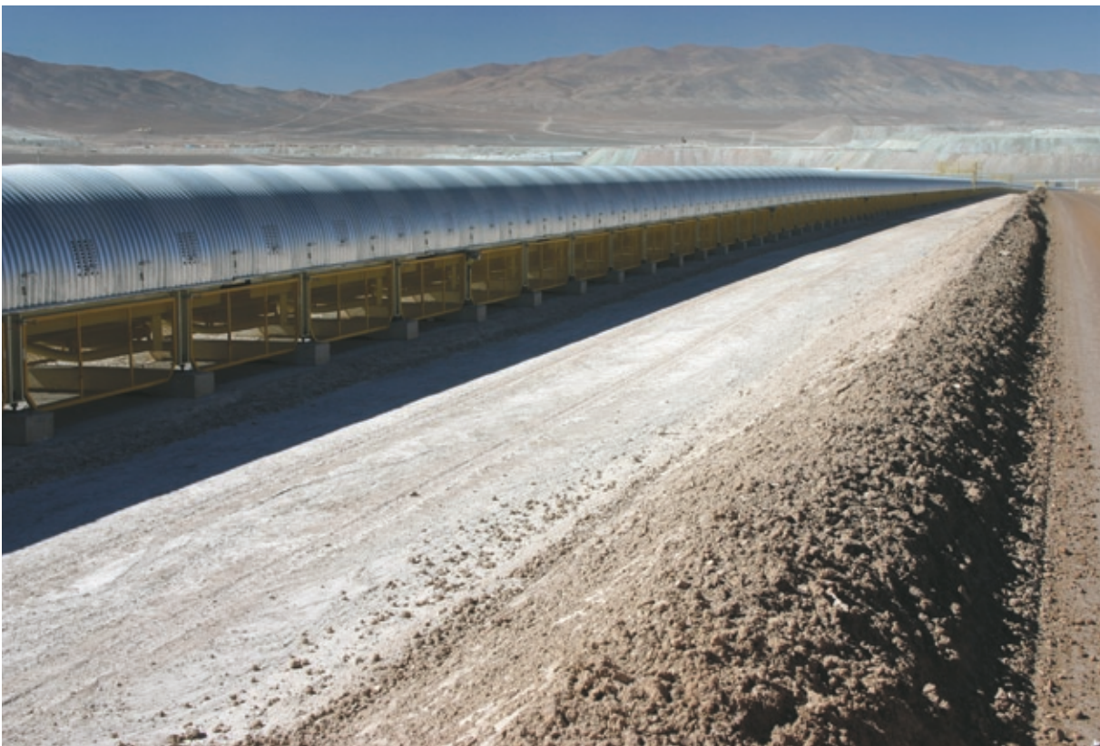
Covered conveyors would reduce dust
