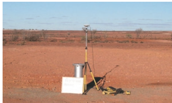
Plate 12.1 Differential GPS equipment
