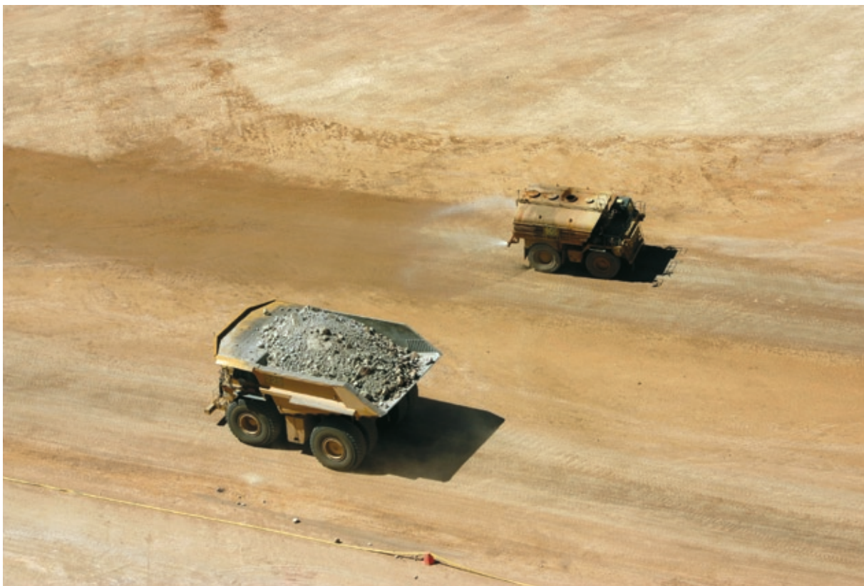
Watering of haul roads for dust suppression
