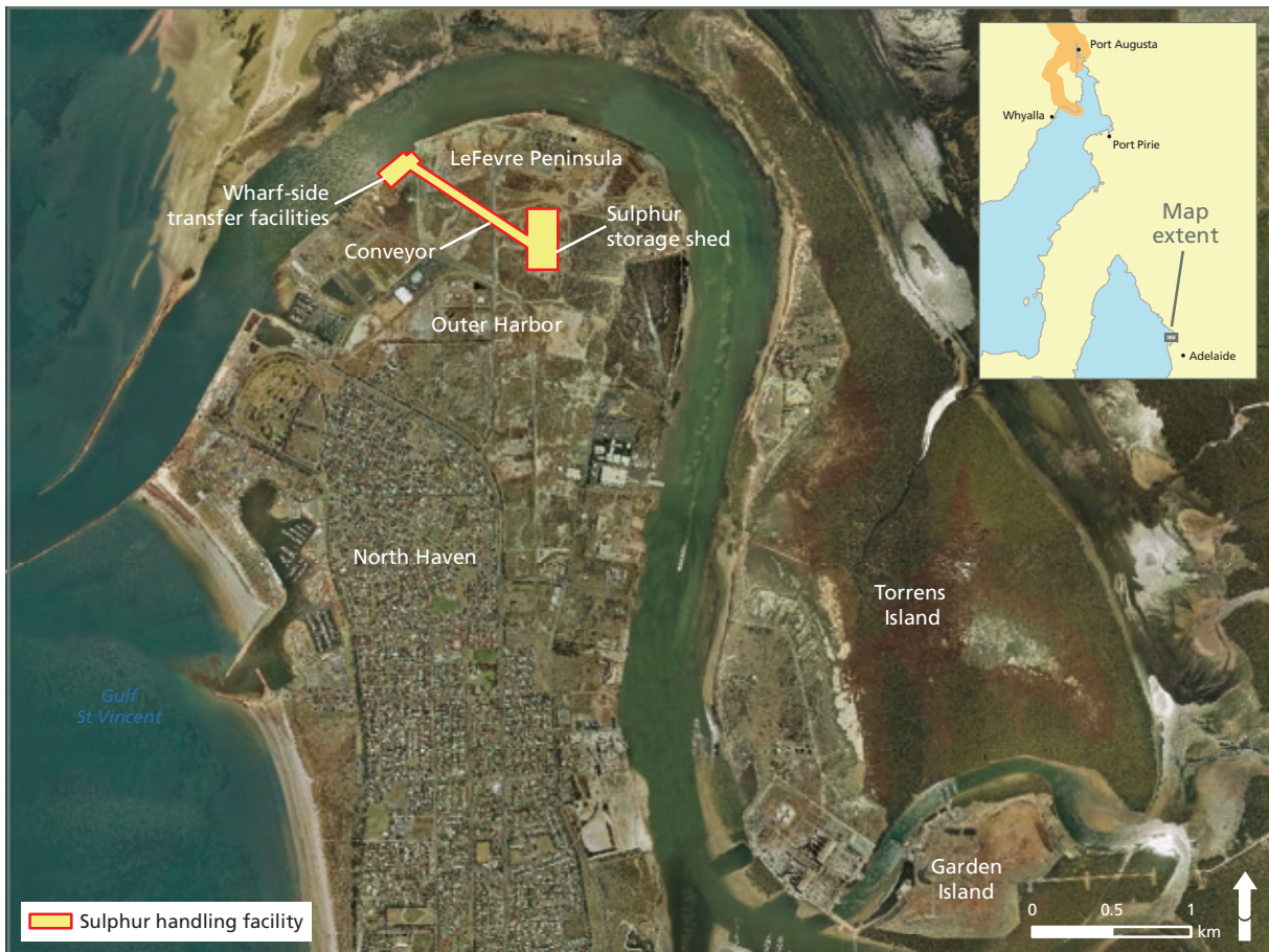
Figure 14 Indicative location and configuration of the Outer Harbor sulphur handling facility at Port Adelaide
