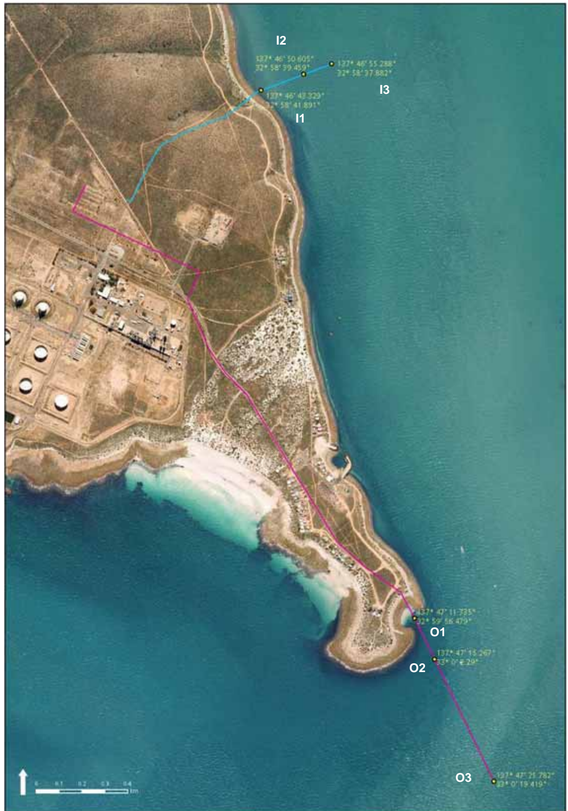
Figure 1: Proposed Desalination Plant Inlet and Outlet Locations
